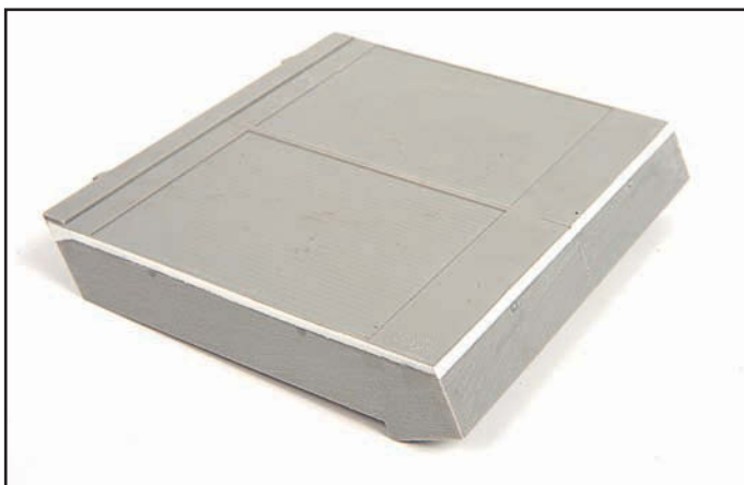
The twin radiator assembly is comprised of two parts but a difference in sizes required a fillet of plastic card to be glued around the edge to eliminate the step.
