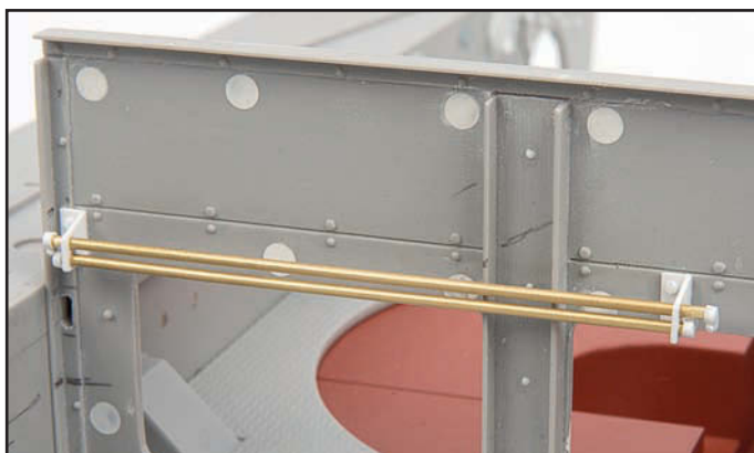
In the engine bay I started to construct the control rods for the throttles. I used Albion Alloy's brass tube to make the rods in order to avoid any possible warping that might occur with plastic.
