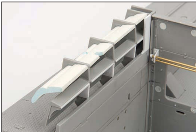
The foamboard was sprayed with a dedicated aerosol primer and sanded smooth. The new deflectors were cut to size and glued in place with CA glue.
