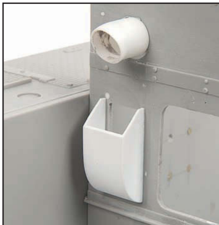
Returning to the firewall I started work on the vents on the crew side. The lower vent sits tight against one of the ammunition racks so this allowed me to establish the size of it. Plastic tube was used to create the crew heater vent at the top of the firewall.
