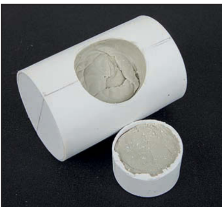
Both the parts have been filled with the putty to give the whole thing more strength as the 20 thou plastic is quite fragile.
