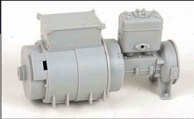
A change of scene now as we move to the engine bay and this little chap. He is the auxiliary generator providing electrical power without running the engine and identifiable by the small square exhaust muffler on the rear of the hull. The kit version seen here is only applicable for the Ausf. A to D.
