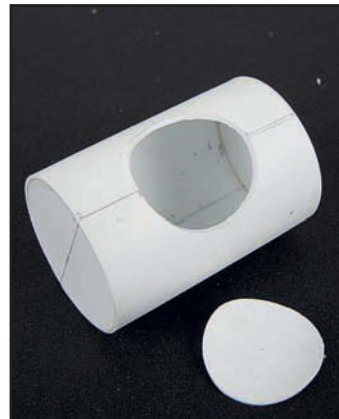
I used a compass cutter to cut out a disc of plastic to accept the generator 'tower'. I constructed the tower by wrapping 20 thou plastic around a circular former and then dipping it in boiling water to fix the shape. This was then
