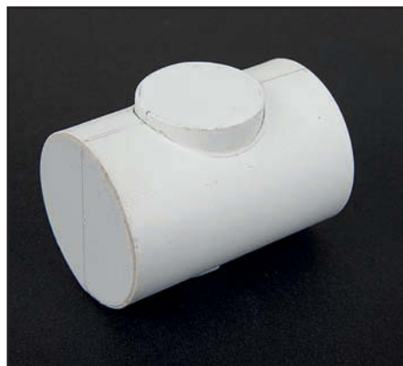
Before the putty set I fitted the tower and made sure that it was sitting at the correct height above the top of the cylinder.
