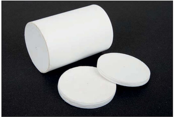
I began to make the new generator by starting with the generator housing by constructing a hollow plastic card cylinder from 20 thou plastic with 30 thou end caps. This was shortened in order to accept the laminated plastic discs seen here which were made of 2 and 3 40 thou discs.
