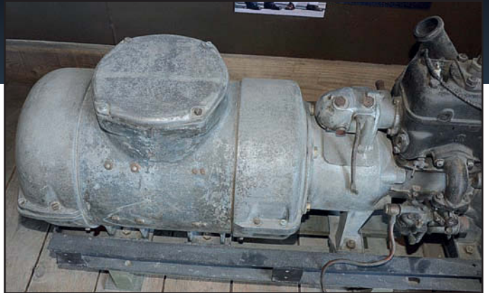
This is the version of the generator for the Ausf. E to H and quite different to the earlier example. The more streamlined generator housing is seen here.
