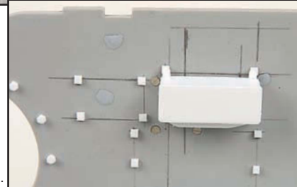
Above Here is the hull wall in an Ausf.H showing the Radio Operator's back rest with the transformer rack tipped on its side below it. The assorted square lugs on the wall mark the fixing locations for fittings and cables on the wall. Studying different vehicles showed the position of the MG Werkzeug box and the communications switch box under the small shelf type cover. This is provided in the kit but is the wrong shape.
