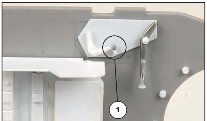
The ball connectors 1 for the rods were made by dipping the end of some plastic rod into Mr Surfacer - two or three coats achieved the correct size.
