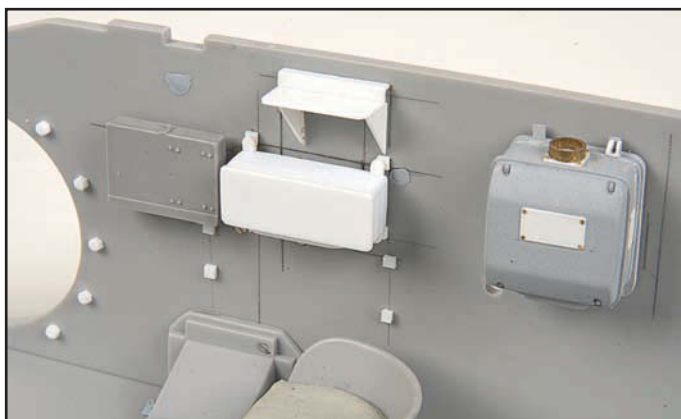
14 The step/shelf/guard was assembled next with sizes established from the photos of the real thing. It appears that the stepped upper edge may be to carry a cable running to the transformer on the right but this will need more research.
