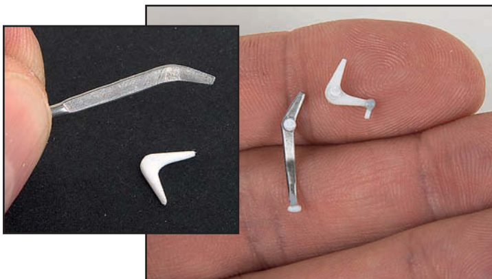
16 To make the pivot connector bracket I cut the basic shape from plastic sheet but for the choke lever I used solder wire which I squashed flat between some pliers. This allowed me to easily create the bent leg of the handle.
