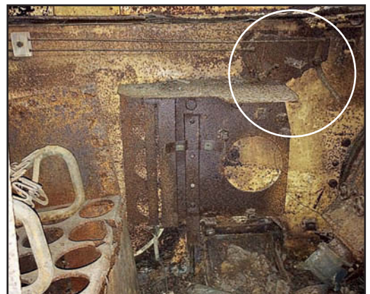
Switching to the other side of the hull I needed to add the throttle linkage starting with this bracket which sits behind the fusebox panel. In this picture of the real thing you can see the control rods running along the hull side, supported by wooden blocks. The protective cover for this has been removed.
