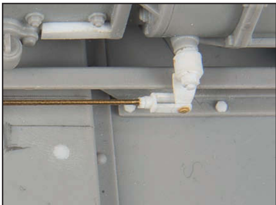
Above The actuating bar is missing from the gearbox but the stub of the shaft is present. Its a simple fitting to make from plastic card and rod. Right The completed dry fitted assembly. Brass rods for the connectors add stability to the fragile assembly.
