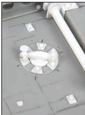
Just in front of the Driver's seat is a small port probably to drain any build up of water in the bottom of the hull. The kit representation is quite basic and lacking the hinge and latch, so these and other missing details were added.
