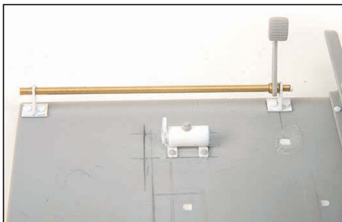
Work starts on the throttle pedal - the kit has it glued into the floor in the wrong position. I modified the kit pedal and used Albion Alloys slide fit brass tube to make the shaft.
