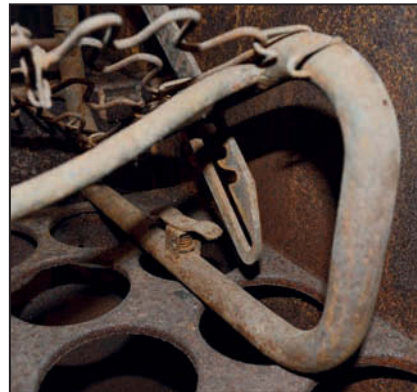
The real seat frame seen here in situ but balanced on top of the ammunition bin that it normally sits in front of. Although some parts of the base have been bent the frame is mostly complete. The seat back angle is adjustable by means of the slotted angled rails on each side and the remains of the original black paint is still visible in places.
