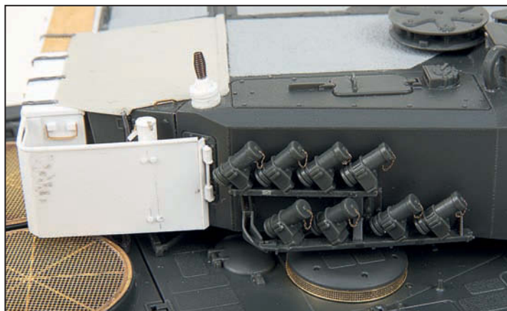
Small photoetched chains from the Hauler set HLU35068 were added to the smoke grenades. The fire extinguisher can be seen stowed in the new bin. The photoetched grilles on the engine deck are supplied in the Meng kit.
