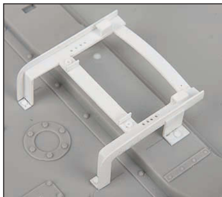
The Driver's seat sits on a frame that is mounted on the raised cover for the suspension system which runs across the hull. The kit simply glues the Driver's seat onto this cover. I constructed my own frame from plastic card
