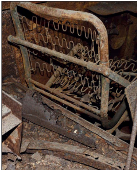
The real seat frame seen here in situ but balanced on top of the ammunition bin that it normally sits in front of. Although some parts of the base have been bent the frame is mostly complete. The seat back angle is adjustable by means of the slotted angled rails on each side and the remains of the original black paint is still visible in places.
