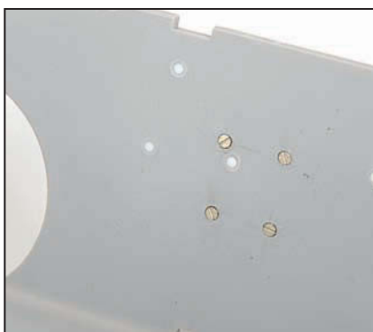
I made the four locking latches with their tapered handles and fitted them ensuring that they were in the locked position otherwise the hatch drops out!
