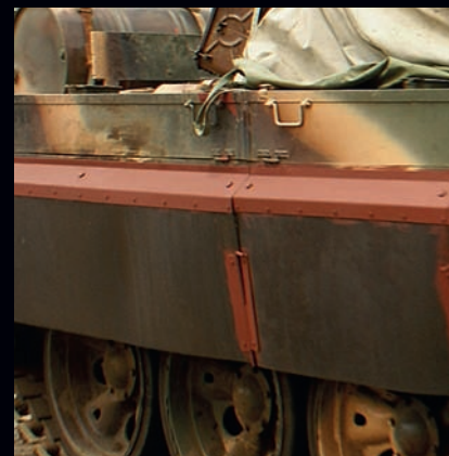
A completed T-55 tank has seen refurbishment and has received the first pattern of side boxes which lacked the reactive armour package. The side fenders are a late addition and are still unpainted.
