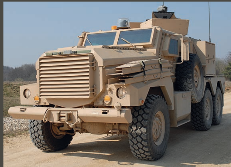
Cougar HEV on exercise mounting a L134A1 40mm Grenade Machine Gun
