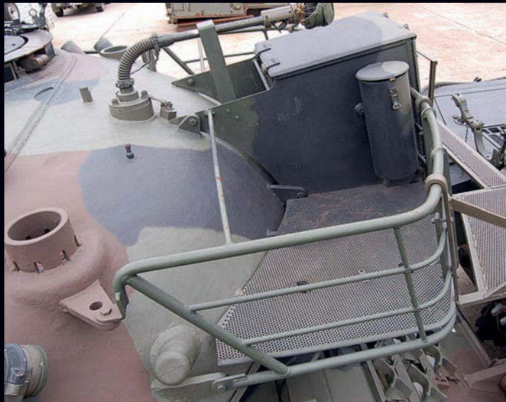
The turret basket features an additional extension rack that is another feature of the Belgian Leopard 1A5BE.
