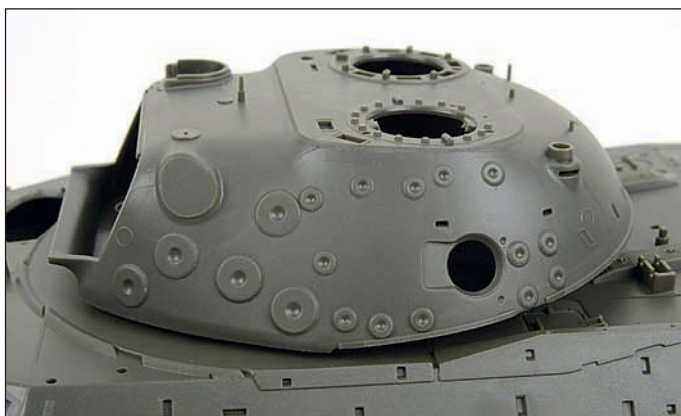
The basic parts of the turret assembled showing the location points for the spaced armour attachment points.
