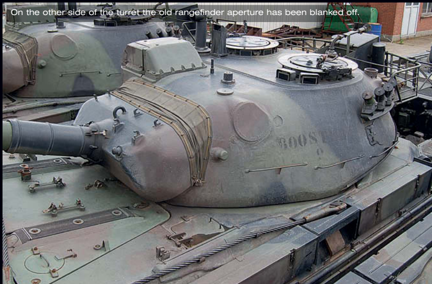
The rather ugly gunner's sighting system distinguishes the Belgian turret and we can see the loopss and cable used to secure the waterproof cover to the mantlet.
