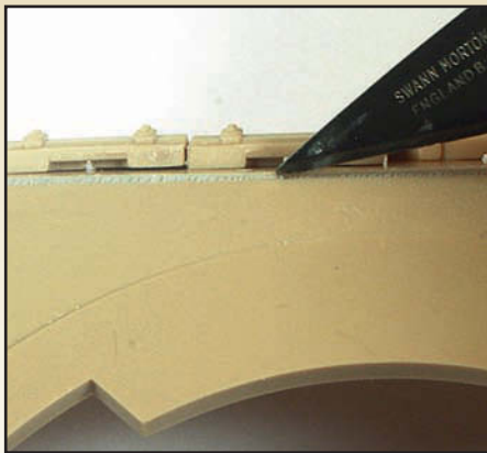
An unwanted seam is filled with Magic Sculp that is sculpted into a weld seam with the point of a knife.
