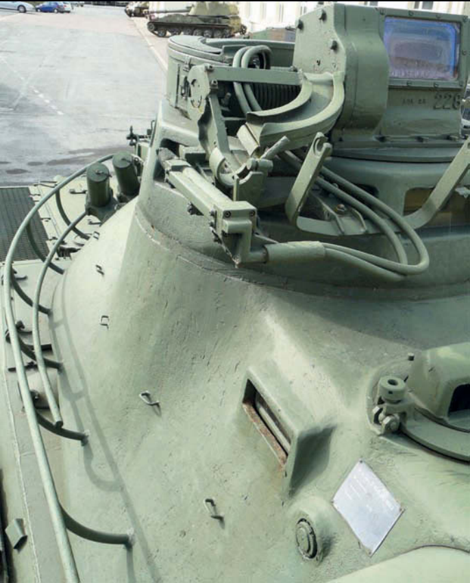
Views of the cupola and MG mount, notice the casting numbers on the front face of the uppermost periscope mount.
