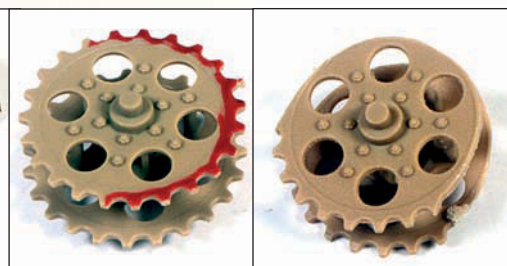
The Friul tracks won't fit the drive sprocket of the kit so the teeth were removed.
