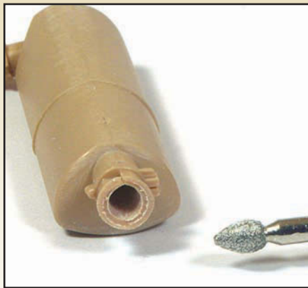
A quick twist with a burr sweetens up the exhaust outlet, the seam running the length of the muffler also needed attention.
