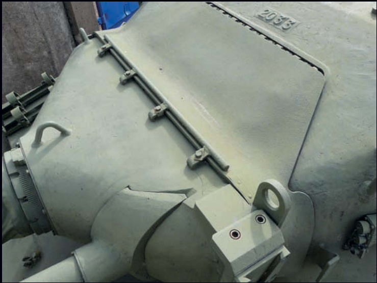
The mantlet cover and casting number on the turret roof.
