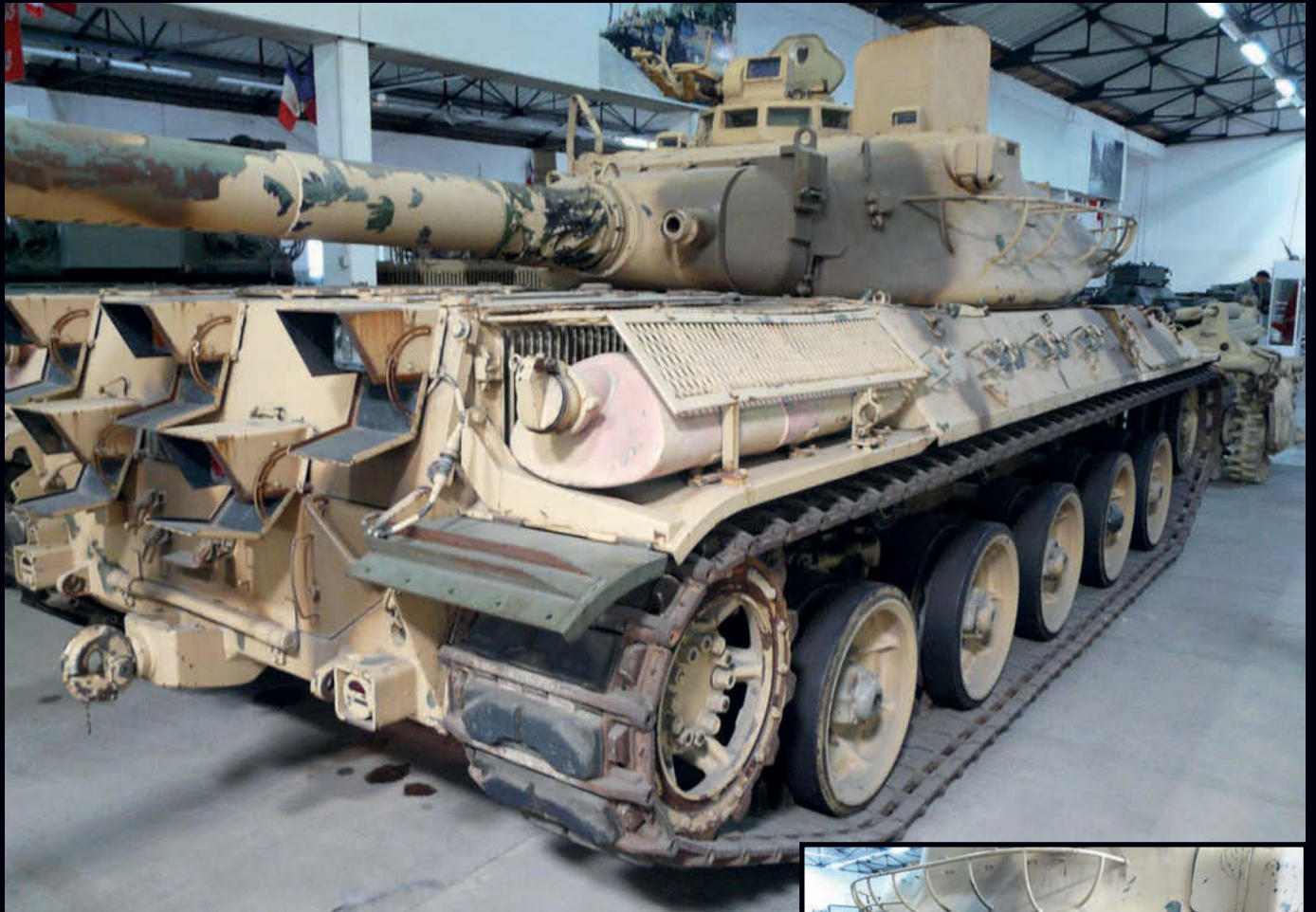
Still carrying its Gulf War Camouflage this AMX-30B has been adapted to carry a mine roller which might explain the non-standard system of lights mounted on the rear of the hull. The pink tone of the exhaust mufflers is also interesting.
