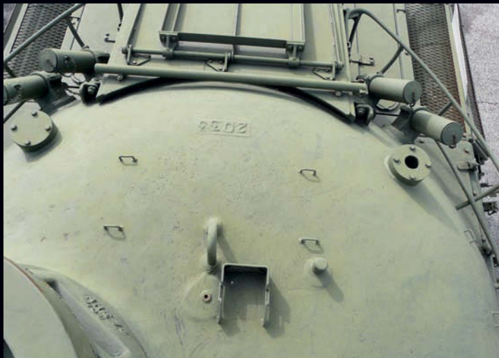
The rear of the turret showing the casting number and tie down loops.
