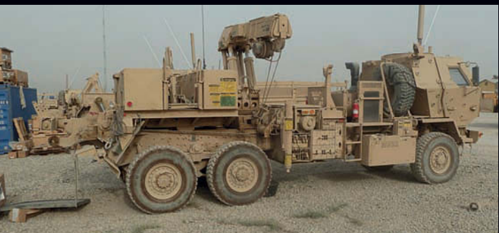
Above A M1089A1 5 ton wrecker fitted with the Low Signature Armored Cab.
