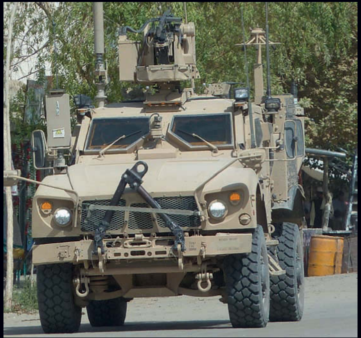
Below An MATV securing a RCP in an Afghan city. This MATV is fitted with a 7,62 Common Remotely Operated Weapons Station (CROWS).
