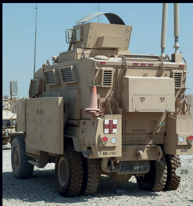
Below : Rear view of a MaxxPro Plus ambulance. Note the double tyres on the rear axle.
