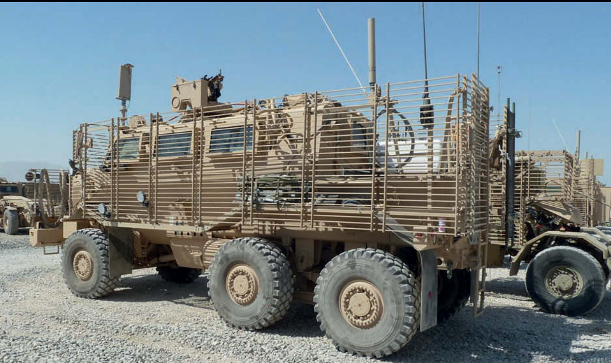
Above Side view of the Buffalo MCV which offers excellent protection from the six man crew during route clearance with the hydraulic interrogation arm.
