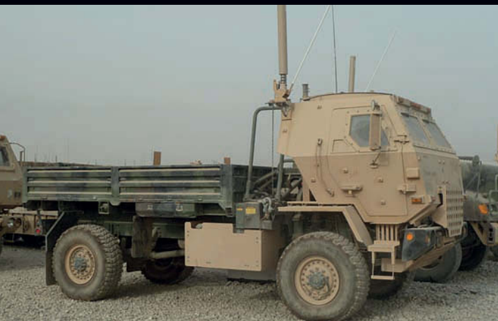
Above Side view of a M1078A1 with Low Signature Armored Cab. This LSAC is a complete replacement for the original cab and not an upgrade to the existing cab.
