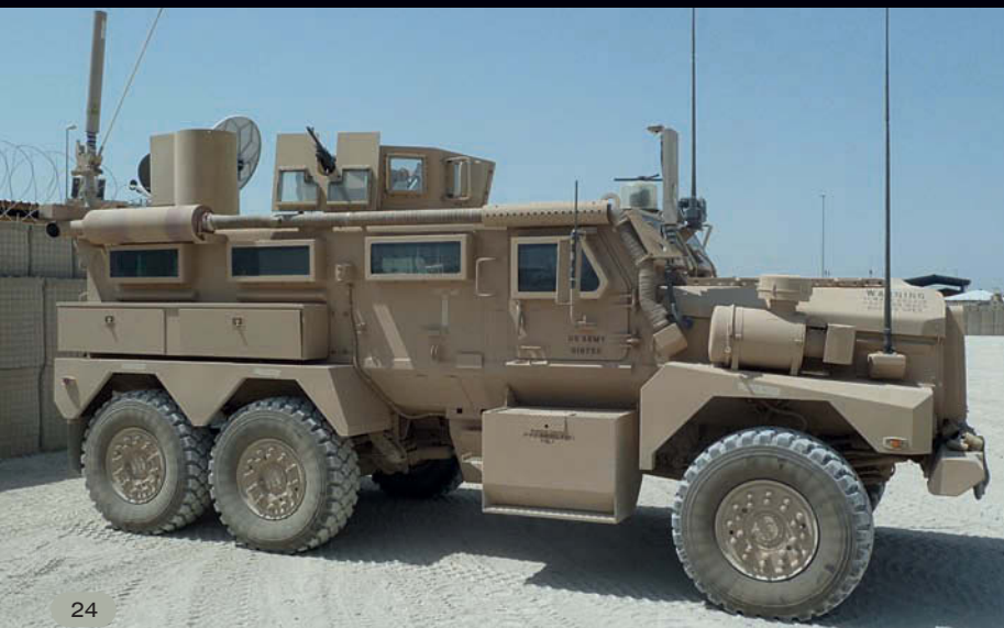
Above General view of the Cougar 6x6 Joint EOD Rapid Response Vehicle or JERRV. The vehicle is fitted with a Vehicle Optic Sensor System (VOSS).
