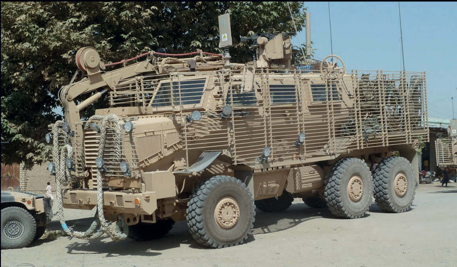
Above A Buffalo fitted with slat armor. This vehicle is a High Value Target of the insurgents.
