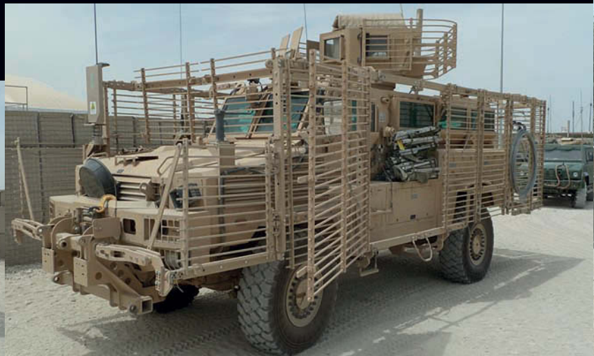
Below Another view of the RG33 with the open slat armour and folded cots stowed on the stowage bins.
