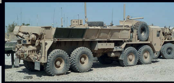
Above & below Side view of a M1120A4 HEMTT with Load Handling System (LHS). The LHS is a demountable flatrack providing self-load/unload capability and capable of transporting an 11-ton payload.
