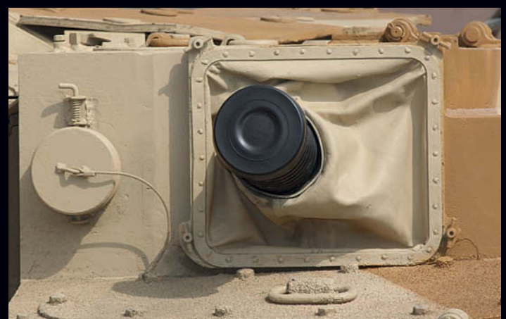
A good view of the anti-slip texture applied to this BMPT. Note also the retaining cable and the protective cap on the grenade launcher
