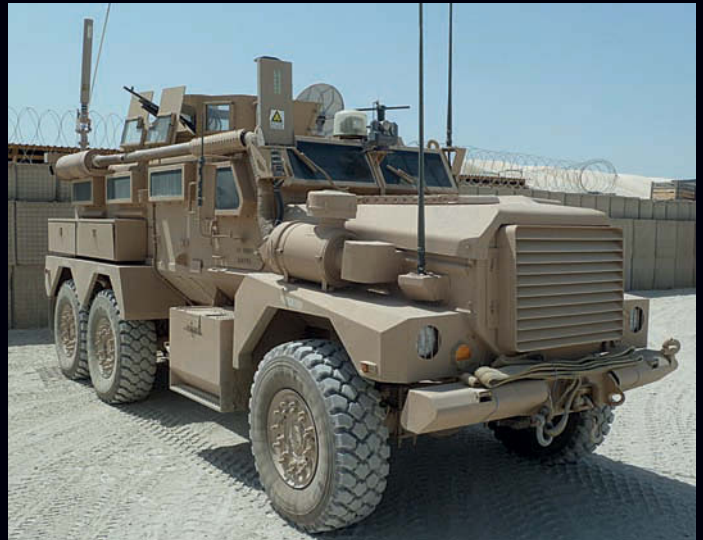
Above Front view of the Cougar EOD vehicle. Note the black Satcom antenna.
