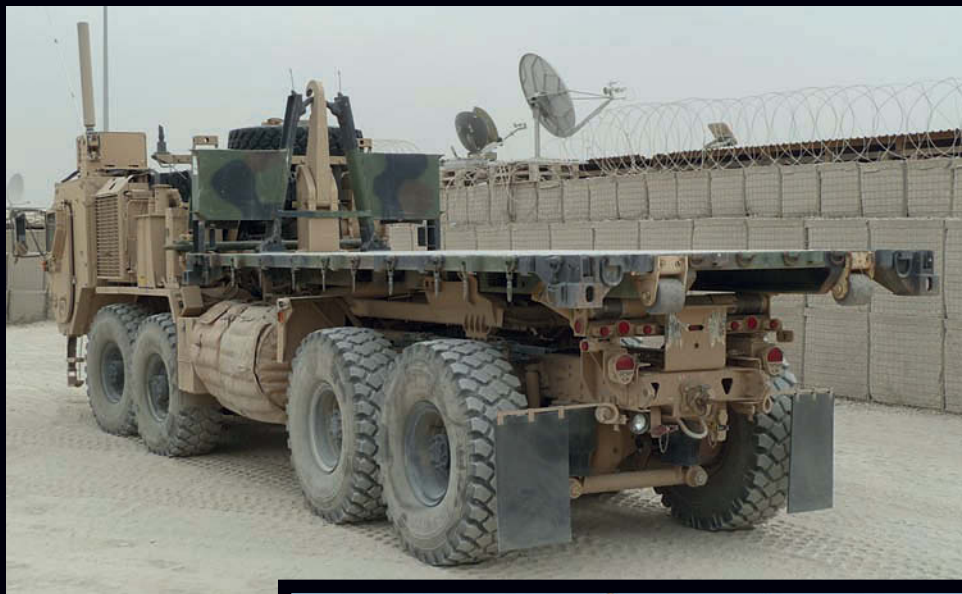
Above & below Side view of a M1120A4 HEMTT with Load Handling System (LHS). The LHS is a demountable flatrack providing self-load/unload capability and capable of transporting an 11-ton payload.
