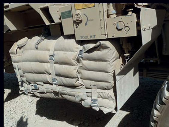
Above Detailed view of the protected fuel cell.
