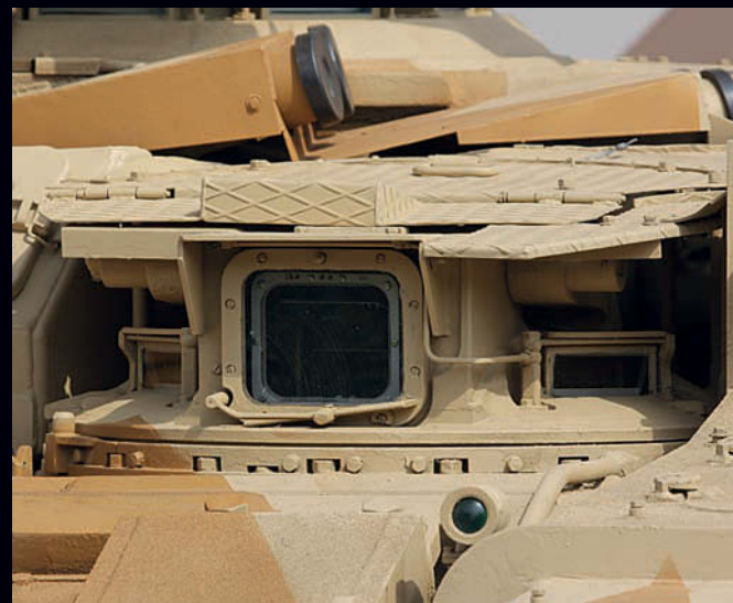
Note the engine intake mesh covers on this vehicle on display in Abu Dhabi not included in the Meng kit.
