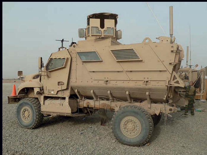
Below : Rear view of a MaxxPro Plus ambulance. Note the double tyres on the rear axle.
