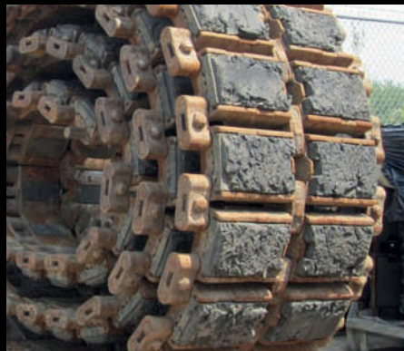
The heavy wear on the track pads can be seen here especially when compared to the neatly coiled new tracks.
