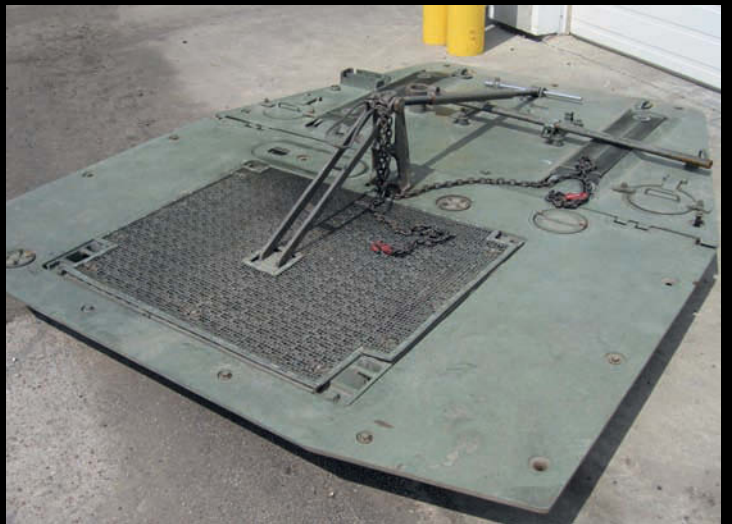
One of the Leopard engine decks showing the clamps which used to extract the whole deck which are usually stowed folded on the left side hull.
