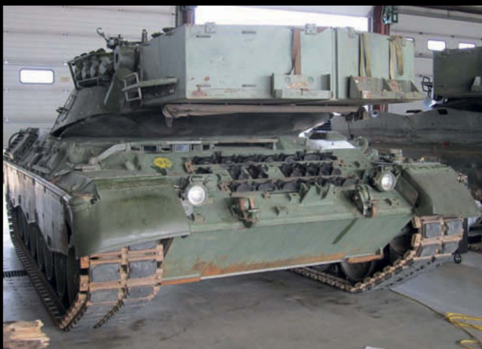
In order to open the engine deck the front section of the spaced turret armour has to be removed, exposing the mounting lugs.
