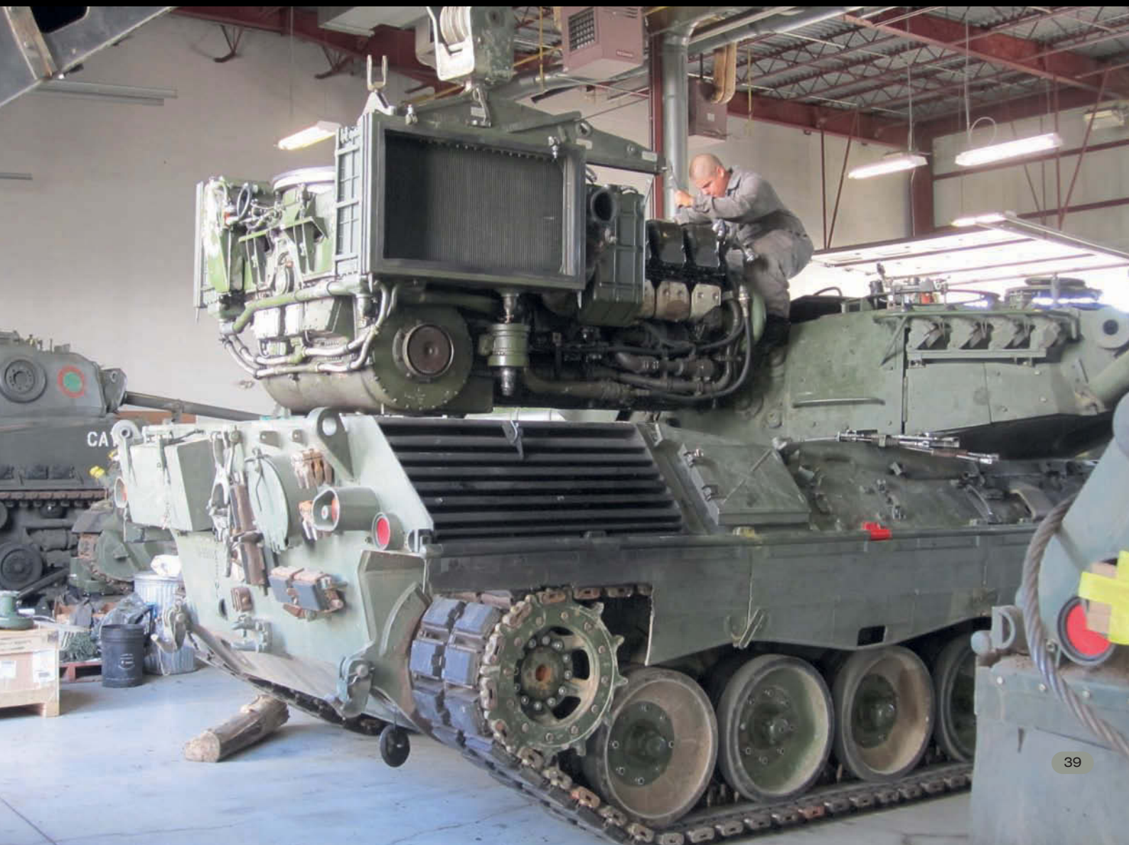
Below With new tracks and roadwheels fitted the power pack is lowered back into the engine bay.
