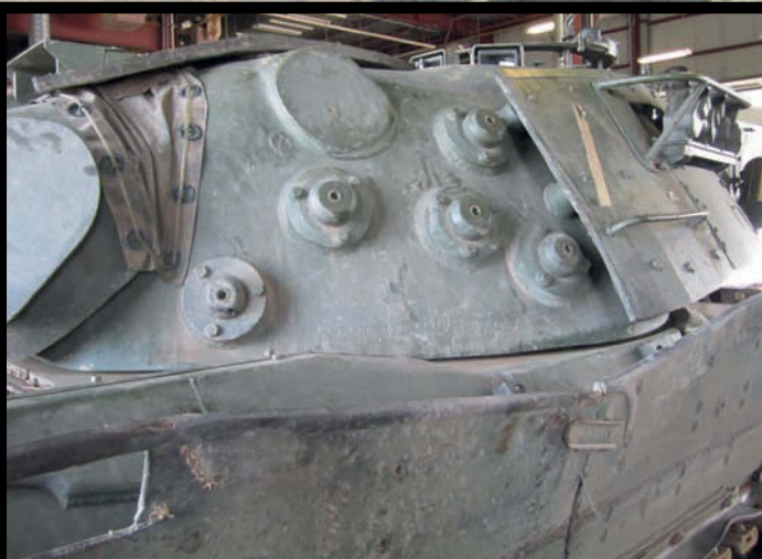
In order to open the engine deck the front section of the spaced turret armour has to be removed, exposing the mounting lugs.
