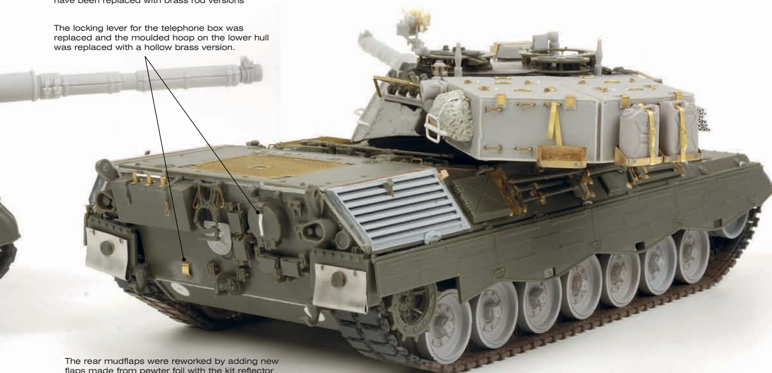
Albion Alloys' aluminium tube was perfect to make the tent pole stowage and easily cut with a scalpel blade. Notice also that the solid filler cap handles have been replaced with brass rod versions
