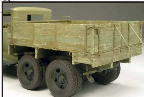
Now it's time to work the wood texture on cargo bed. Weathering for wood is not the same as on a metal surface, with subtle differences in colour, chipping and paint wear. Remember again to use the logical approach...a side of cargo bed won't have the same weathering process and fatigue as the floor or the tail gate.
