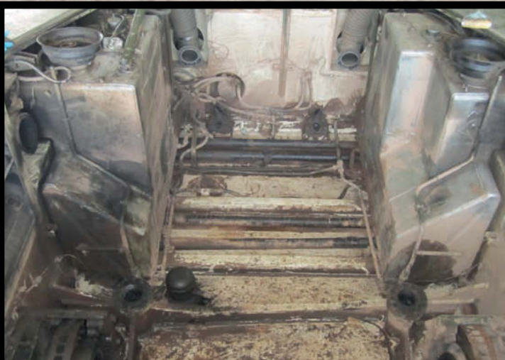
A view of the empty engine bay with the two fuel cells mounted on each side of the front of the bay.
