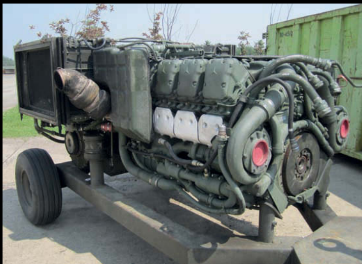
The Leopard power pack sitting on a dedicated servicing trolley
