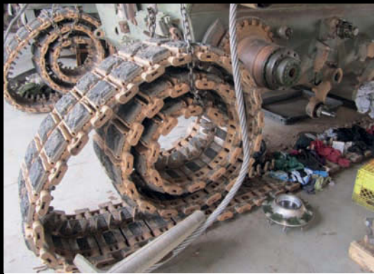
The heavy wear on the track pads can be seen here especially when compared to the neatly coiled new tracks.
