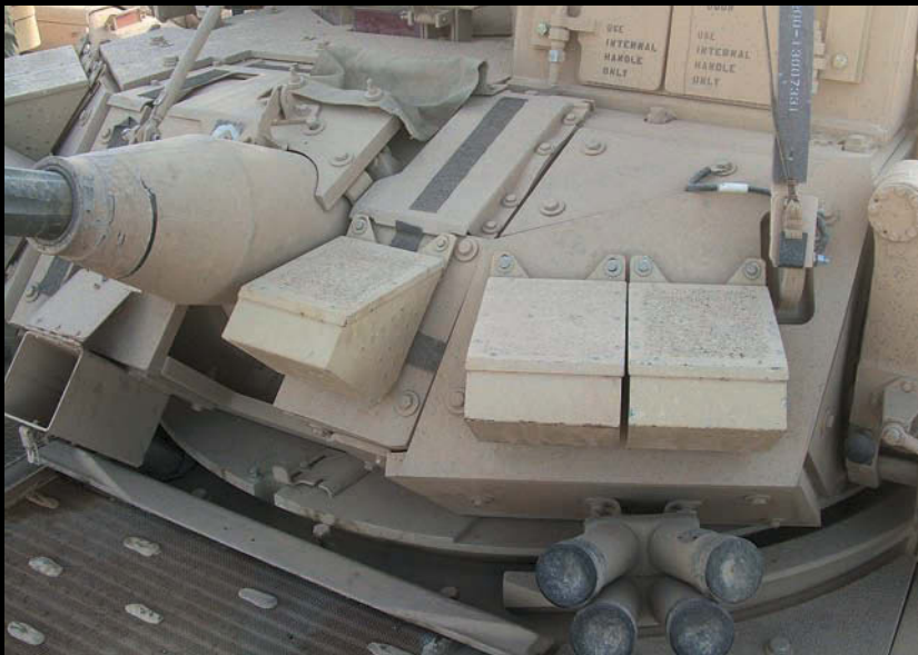
Gunner's Integrated Sight Unit at the top of the image, note the stenciled text (provided in the kit as a decal).
