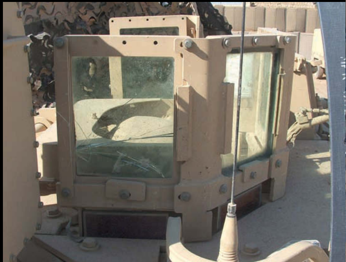
Commander's armoured glass showing some damage
