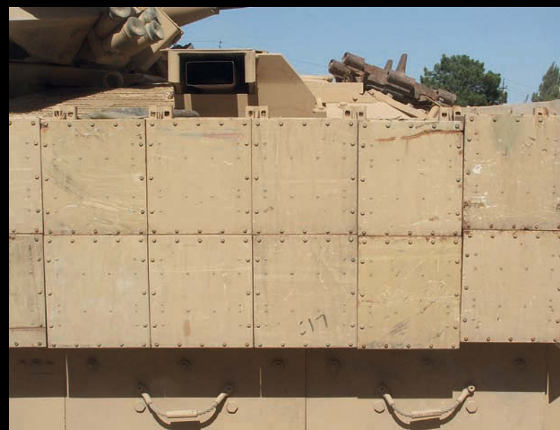
These close-ups of the ERA blocks show plenty of scuffs and scrapes, even signs of rust
