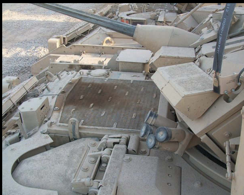
Note the staining around the intake screen and the distinctive fluted design of the gun barrel
