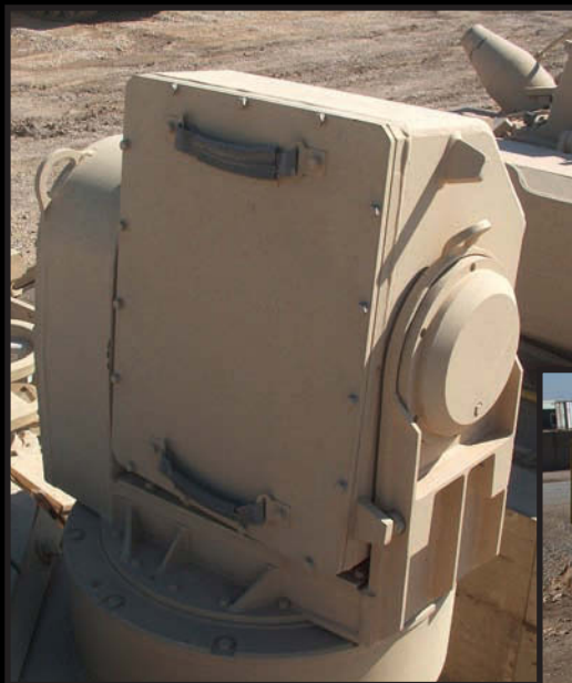
Commander's Independent Thermal Viewer in a folded position
