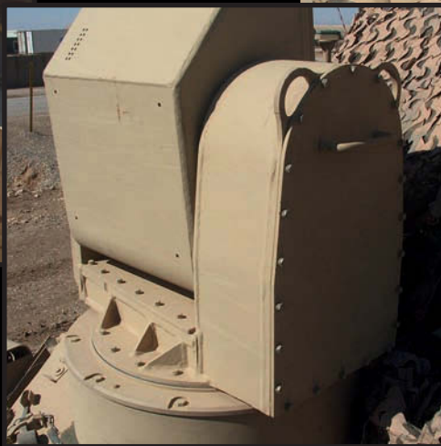
Rear of the CITV showing the heavy welding. The MENG parts allow full rotation and elevation
