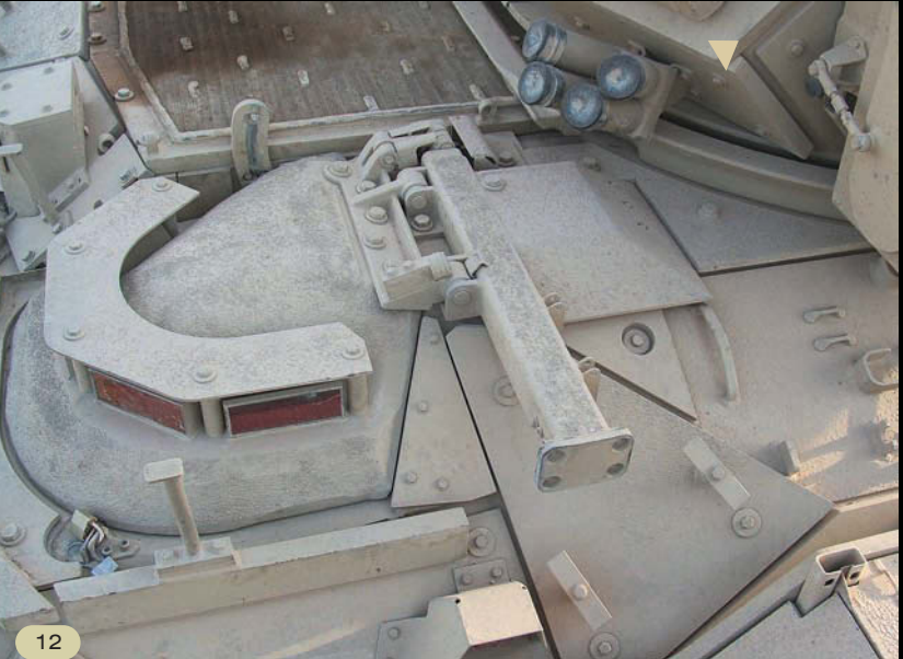
Driver's hatch, note the empty brackets where the spare trunk link and shovel have been removed
