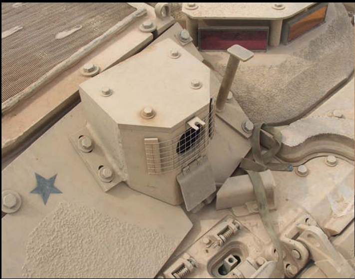
The Driver's viewer optic shown open and a good close-up of the vision blocks with distinctive reflective finish.
