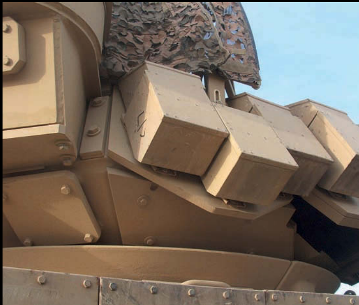
Underside of the turret showing the complexed multi-layered armour
