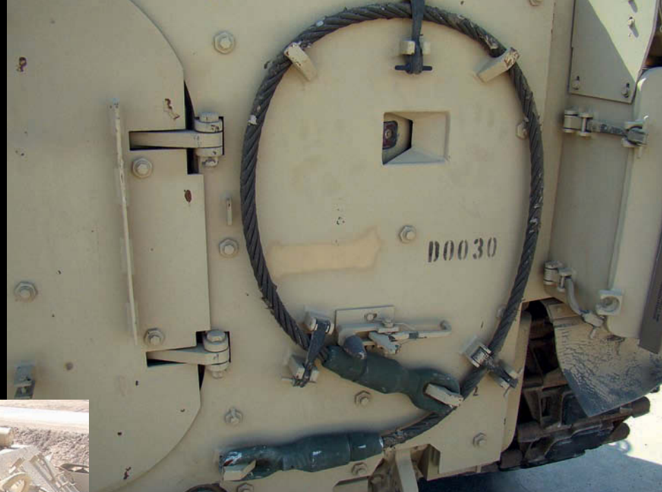
The tow cable finishes are shown to good effect here, note also the rubber retaining toggles have lost all of their paint finish with a similar effect on the mud flap
