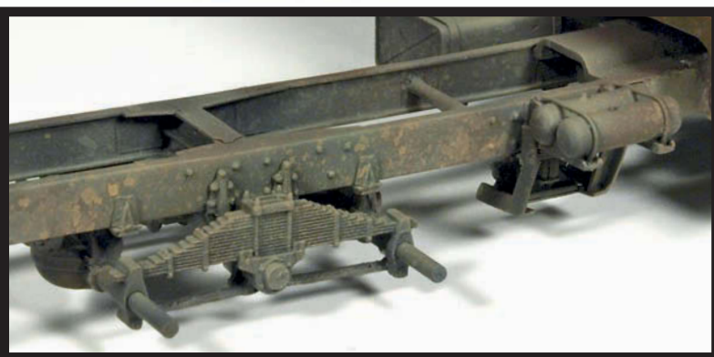
Initial weathering stages of the chassis and wheels shown above. See how the gradual build up of layers of subtle effects results in the realistic and interesting finish below.
