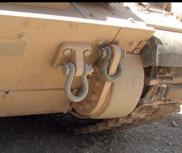
Tow hook detail showing a different colour finish
