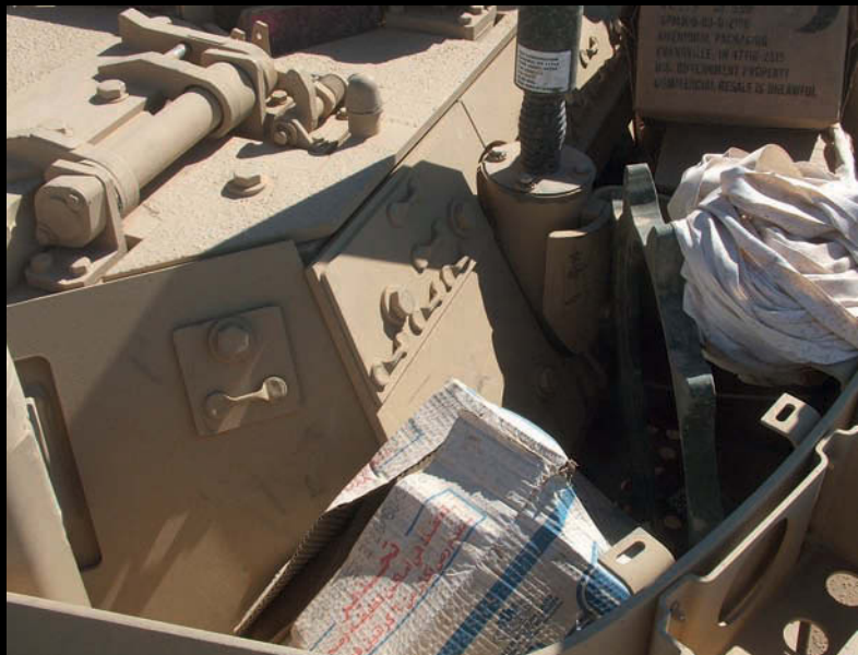
To the rear of the gunner's hatch an assortment of stowage in the rear bin including a spare drive sprocket
