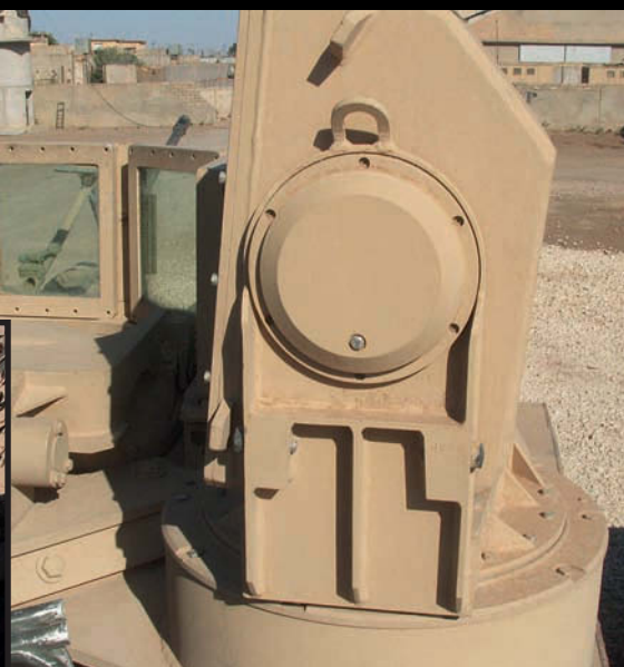
Rear of the CITV showing the heavy welding. The MENG parts allow full rotation and elevation
