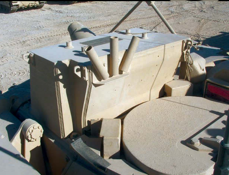
The rear of the gunner's vision unit, note the heavy weld beads and the absent bushmaster gun barrel
