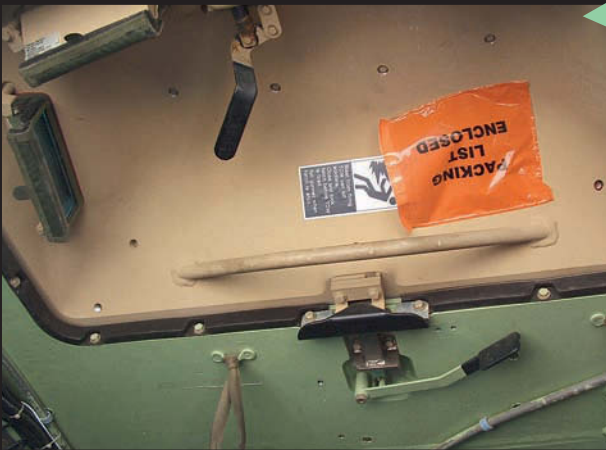
The roof hatch viewed from the passenger compartment. Note the external colour finish, the heavy rubber bump strip / seal and the handle detail.
