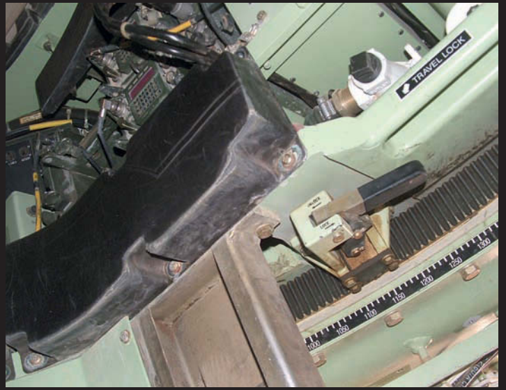
A view around the turret showing the high-tech 25mm M242 Bushmaster 'Chain Gun' system (referring to the roller chain that drives the bolt back and forth) Note the toothed turret ring and travel lock.
