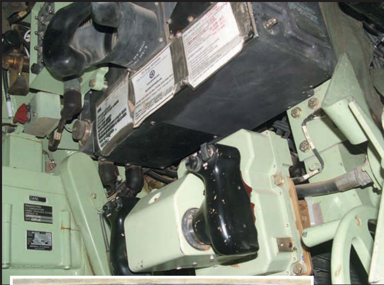
A view around the turret showing the high-tech 25mm M242 Bushmaster 'Chain Gun' system (referring to the roller chain that drives the bolt back and forth) Note the toothed turret ring and travel lock.
