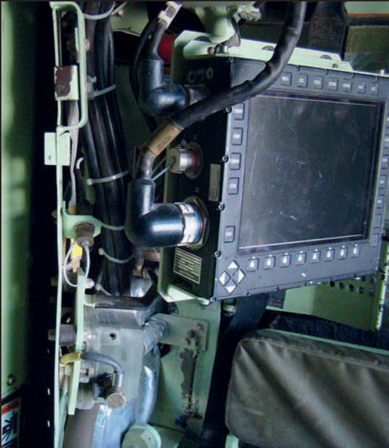
Complex wiring to the monitor on the right of the turret basket door
