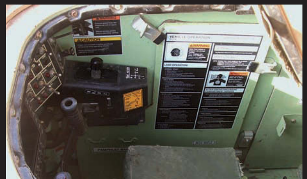
Views to either side of the driver. Note the folding seat back to allow access to the rear of the vehicle and the height adjuster at the left rear corner of the seat base.
