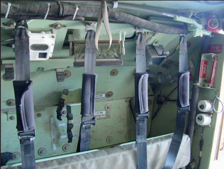
View towards the right rear corner, note the improvised hanging grab-handle and the anodized finish on the armour bolts and washers
