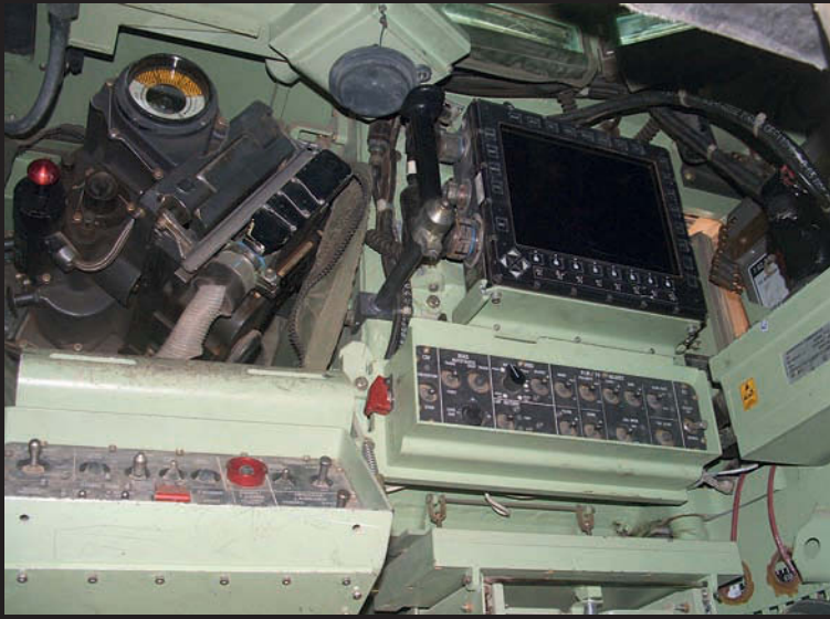
A view around the turret showing the high-tech 25mm M242 Bushmaster 'Chain Gun' system (referring to the roller chain that drives the bolt back and forth) Note the toothed turret ring and travel lock.
