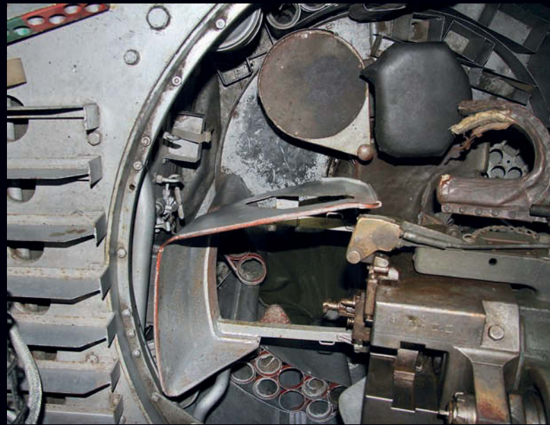
Note the various finishes on the different parts of the breech and the silver / white interior colour.
