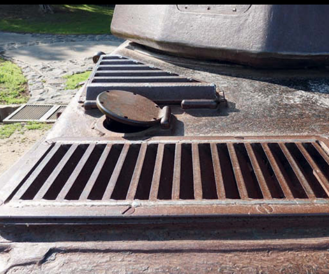
The bow is a mix of cast components and armoured plate. Note the conical head bolts and the flush fitted screw heads.
