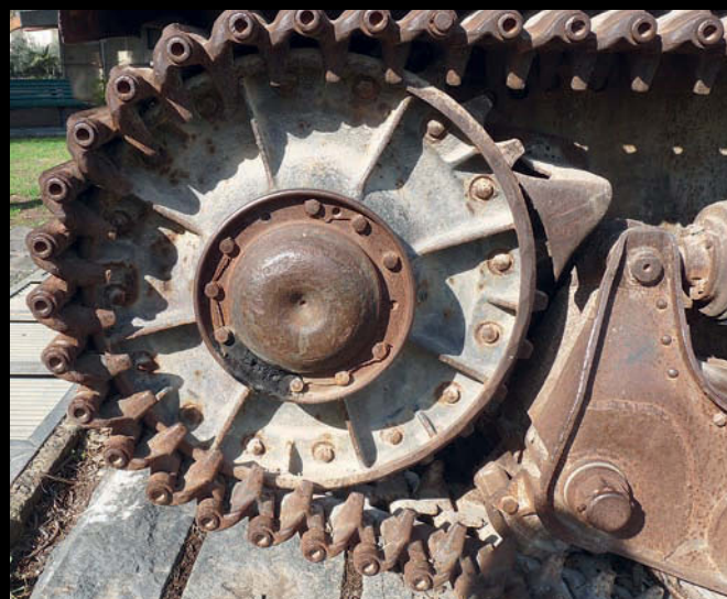
Close ups of the running gear where sadly most of the roadwheel tires have been burnt away.
