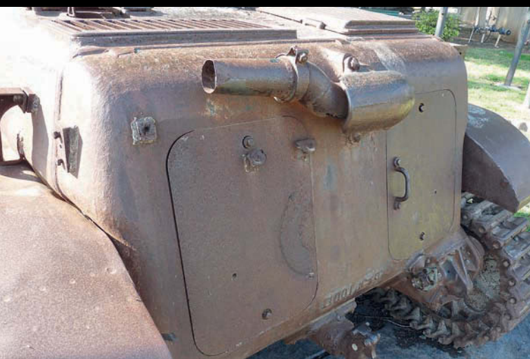
The rear of the Renault with the pair of engine inspection hatches. This is another cast component as indicated by the casting number above the tow hook.
