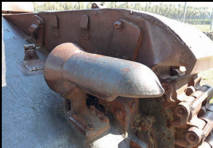
The shielded headlamp was a standard fitting on all French armoured vehicles.
