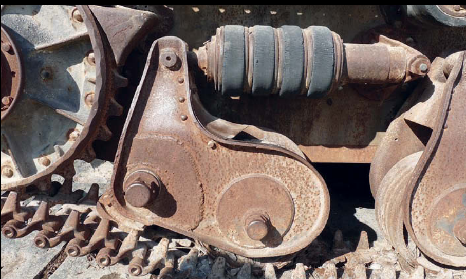
Close ups of the running gear where sadly most of the roadwheel tires have been burnt away.
