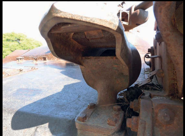
The damaged gun gives the turret a very different look with the barrel extended far beyond its normal resting position. Note the prominent casting numbers on the turret and the empty location hole for the missing lifting hook above the vision port.
