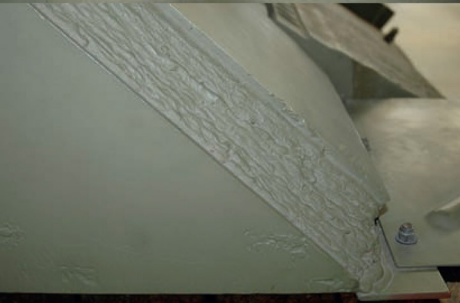
The left side front lift ring has heavy weld beads where it is attached to the glacis. In the background is the riser for the gun travel lock mounts. This changes the geometry of the travel lock necessary because of the additional armour on the hull.
