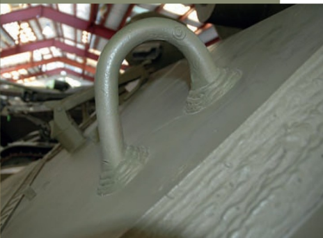
The left side front lift ring has heavy weld beads where it is attached to the glacis. In the background is the riser for the gun travel lock mounts. This changes the geometry of the travel lock necessary because of the additional armour on the hull.
