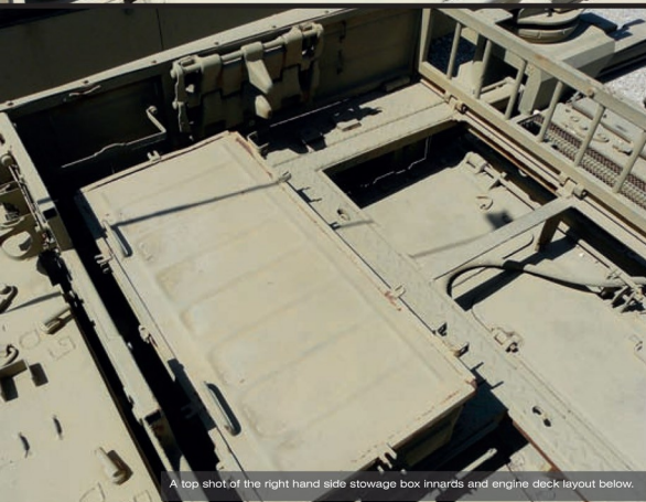
Interesting photos of the storage box framework missing a number of floor sections below which we see the engine hatches and some of the winch box housing.
