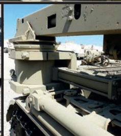
Detail shot of the rear inside of the jib arm which is attached to the upper hull at the rear right hand side of the VT.
