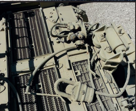
Rear shot of the VT showing the lowered tow anchor similar to that found on a wide range of Warsaw Pact ARVs.
