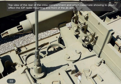
These empty brackets are for stowing oxy-acetylene welding bottles as associated with IDF recovery vehicles.
