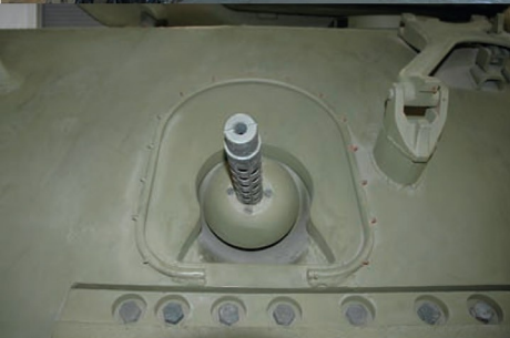
The additional armour added to the glacis has a bell shaped cut out to allow movement of the bow machine gun. Some of the first M4A3E2s produced did not have the fixture for attaching the m.g. foul weather cover.
