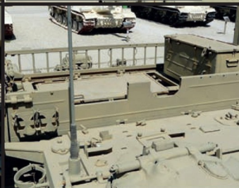
View of the jib arm as mounted on the upper hull of note are the various IDF fittings added to the VT-55.
