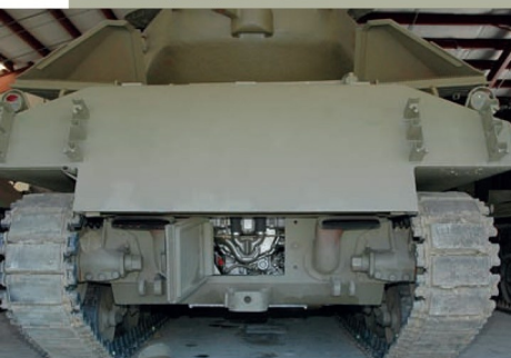
The M4A3E2 was equipped with the standard VVSS suspension system with the upswept bracket for the return rollers. The added weight made the suspension sit slightly lower. The restored example has the pressed wheels, most factory shots show the welded wheel, and due to wheel failures many received late big bearing wheels in the field.
