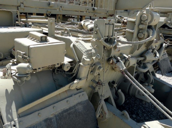
Detail shot of the formation lights and the horn on the VT
