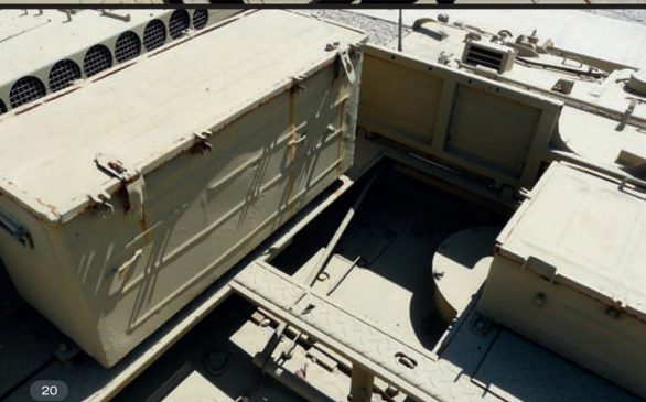
A top shot of the right hand side storage box innards and engine deck layout below.
