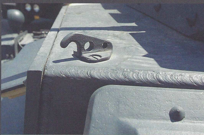
A close up of the welded hull joint clearly showing the section of additional armour bolted to the hull front.
