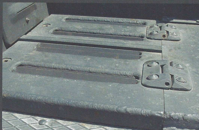
The radiator intake grille also doubled as a hatch providing access to the fighting compartment.
