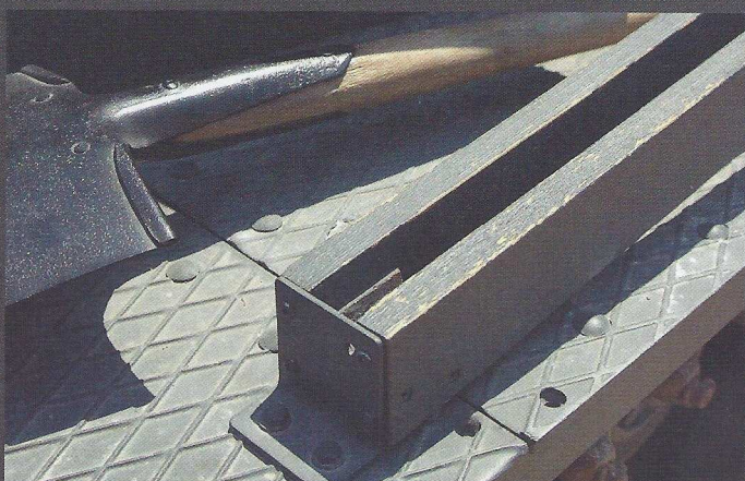
The front end of the wooden rack used to stow the antenna.
