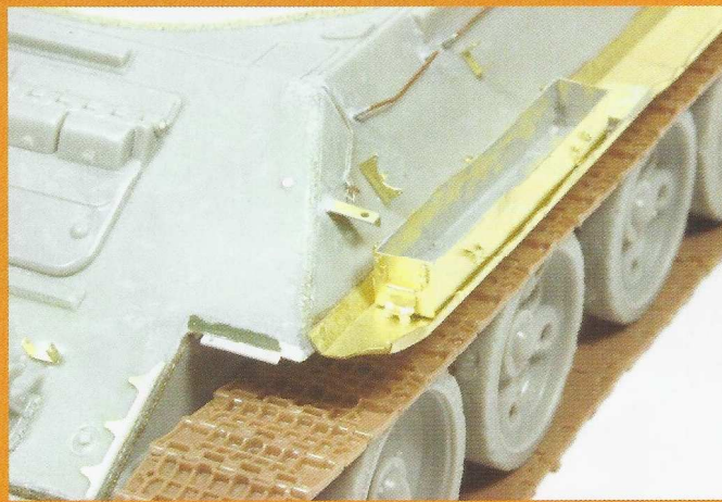
Pieces of plastic strip representing flat bars, where the missing mudguards would have been attached, were glued on the end of the fenders.
