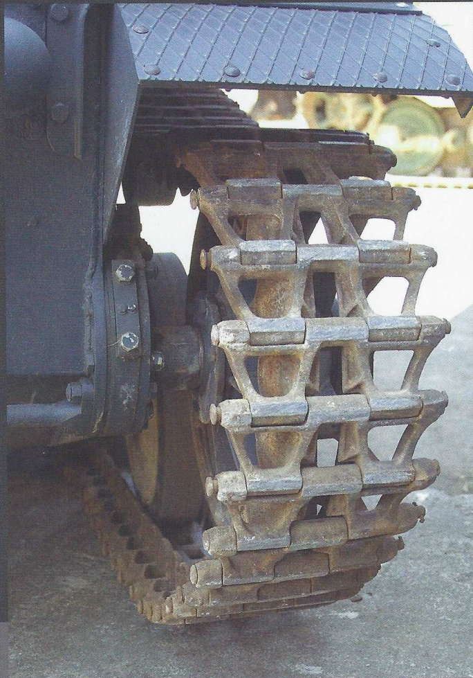
Two views of the rear corners of the hull showing the bracket used to secure the trackguards, the weld detail and the mounting for the idler wheel. Note also the finish on the tracks.
