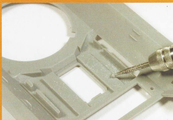
In order to properly fit the photo-etch air vents from the Aber set, I used my Dremel to remove some plastic ribs in the engine bay.
