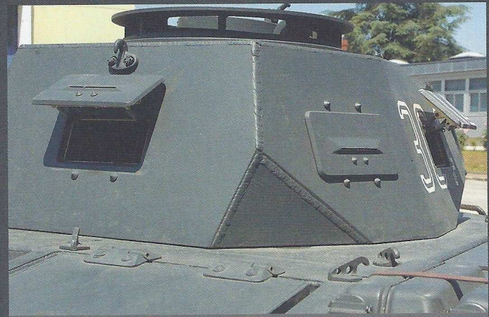
A rear three quarter view of the turret showing the weld detail and the vision ports.
