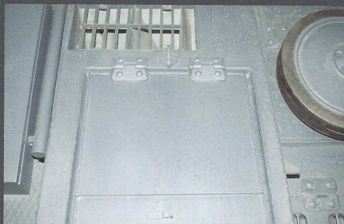
The engine hatch also features a rounded welded edge and has a distinctive trough around the the circumference.
