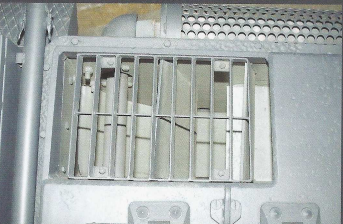
The hot air outlet at the rear corner of the engine deck with the exhaust outlet running through this space.
