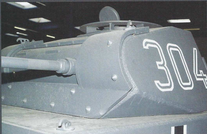
The front of the turret showing the same style of welded joints as the hull. The applique armour is comprised of three separate panels rivetted onto the turret.
