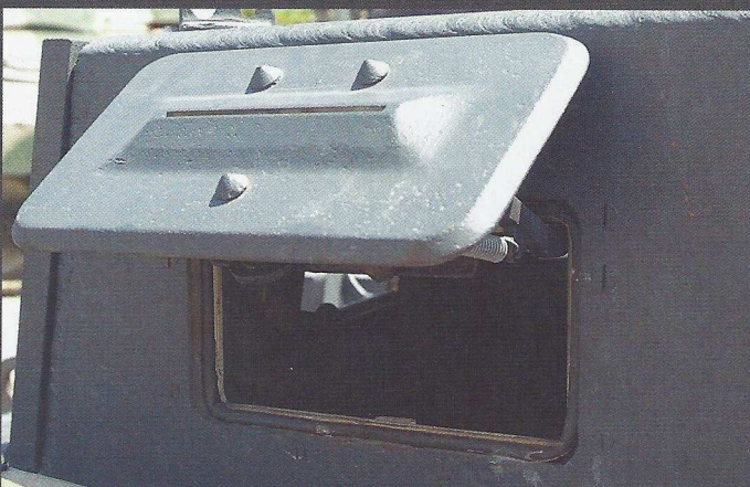
The driver's visor seen in the open position. Note the screwhead detail and rubber strip around the opening.
