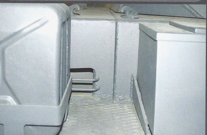
Just visible behind the jerry can stowage is the air intake opening running down the side of the engine deck.
