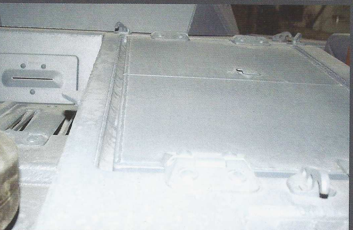
This view up the engine deck clearly shows the rebated trough around the engine hatch.
