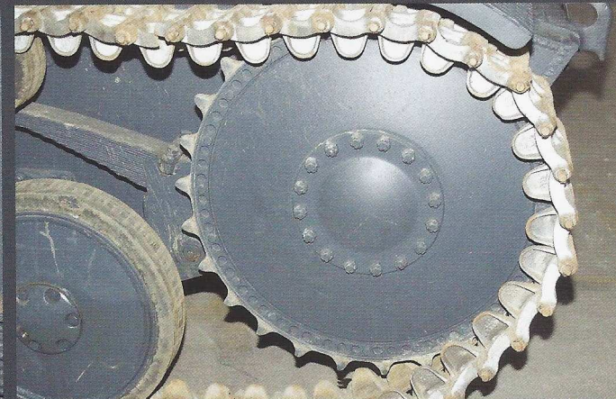
The drive sprocket, note the extended position of the glasis and tow hook.
