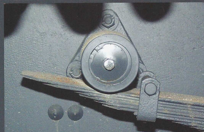
A close up of one of the rollers on the suspension leaf springs.
