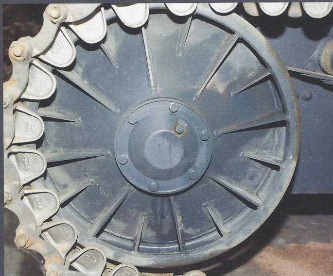
The idler wheel with its welded ribs
