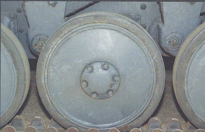
One of the roadwheels notice the lubrication point on the hub.
