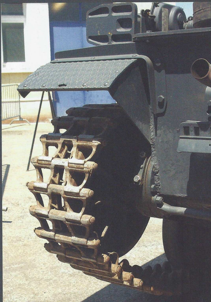
Two views of the rear corners of the hull showing the bracket used to secure the trackguards, the weld detail and the mounting for the idler wheel. Note also the finish on the tracks.
