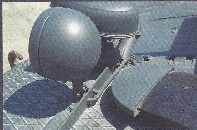
The headlamp fittings on the track guard - the fitting on the extreme right behind the Notek lamp is a padded stopper for the glacis hatch.
