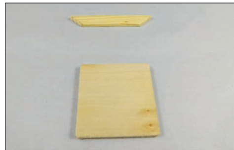
Step 6. Cut the bottom of the flower box to 1/8" x 1 9/16" x 1 9/16" square. Sand to fit. Cut the top frame of the flower box. 4 pieces 1/8" x 3/8" x 2 1/4" on long side (outside) at 45 de-
