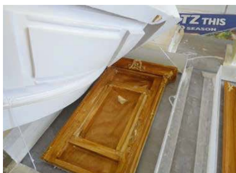
Removing the mould from the pattern.
