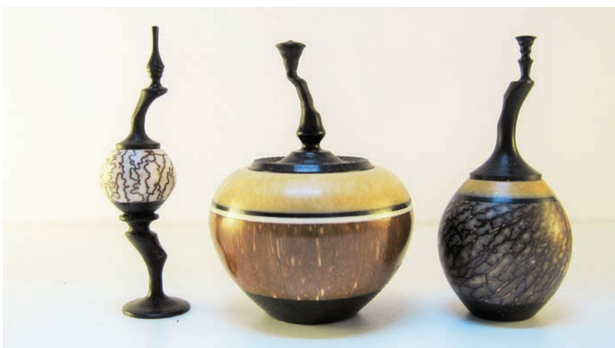
Examples of lidded vessels turned off axis with an eccentric chuck. These vessels are slightly larger at approximately 2" tall.
