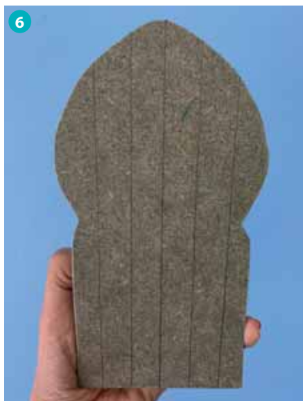
6 Mark planks with a pencil on both sides of the door.
