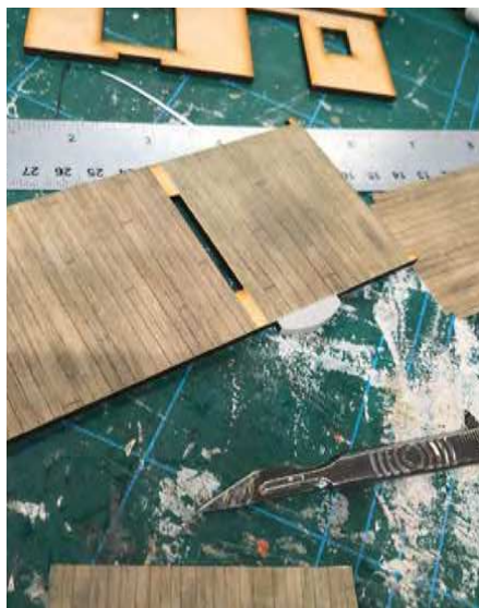
▲ Mind the gap! Always leave a gap in any floor covering to allow internal partitions to be fitted. Always leave a gap in any floor covering to allow internal partitions to be fitted.
