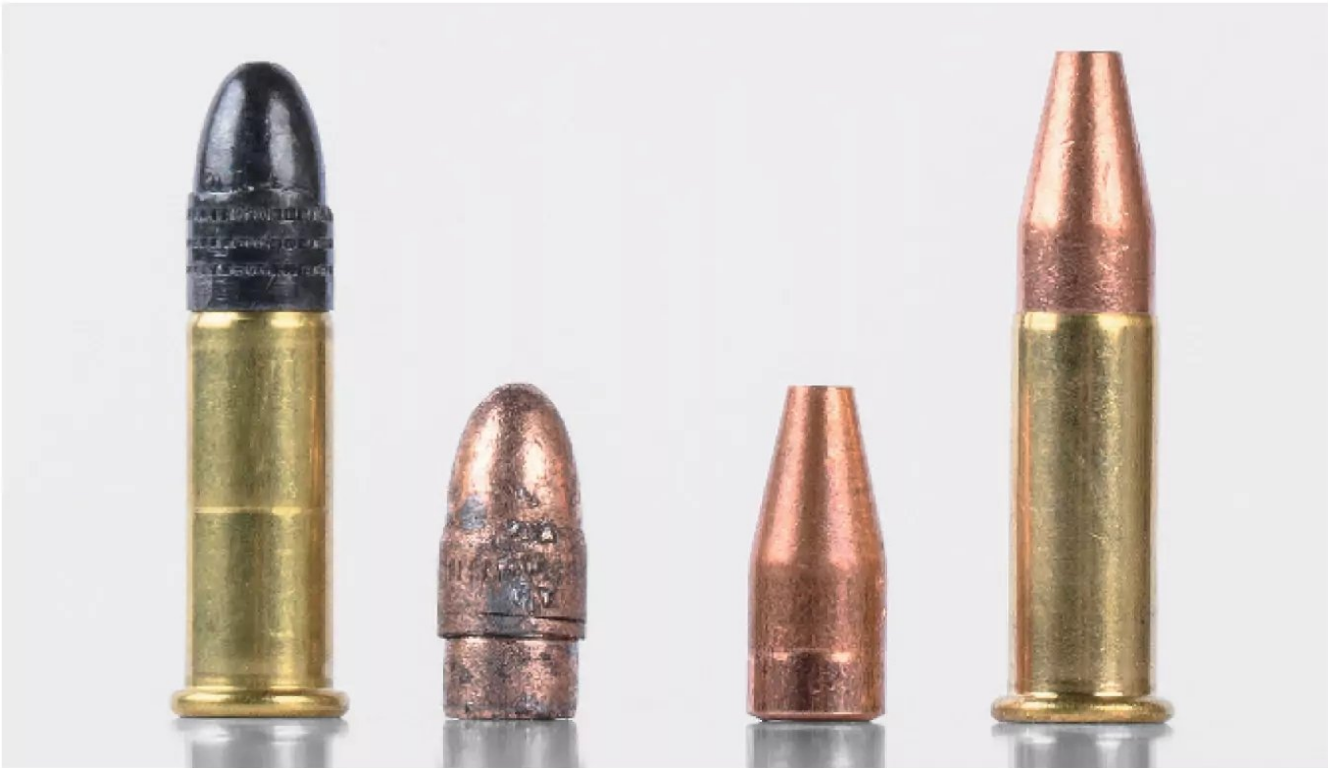
The .22 LR (l.) uses a heeled bullet while the .21 Sharp’s bullet—the monometal version is shown here (r.)—has parallel sides. Eliminating the heel is potentially beneficial to accuracy and consistency.
