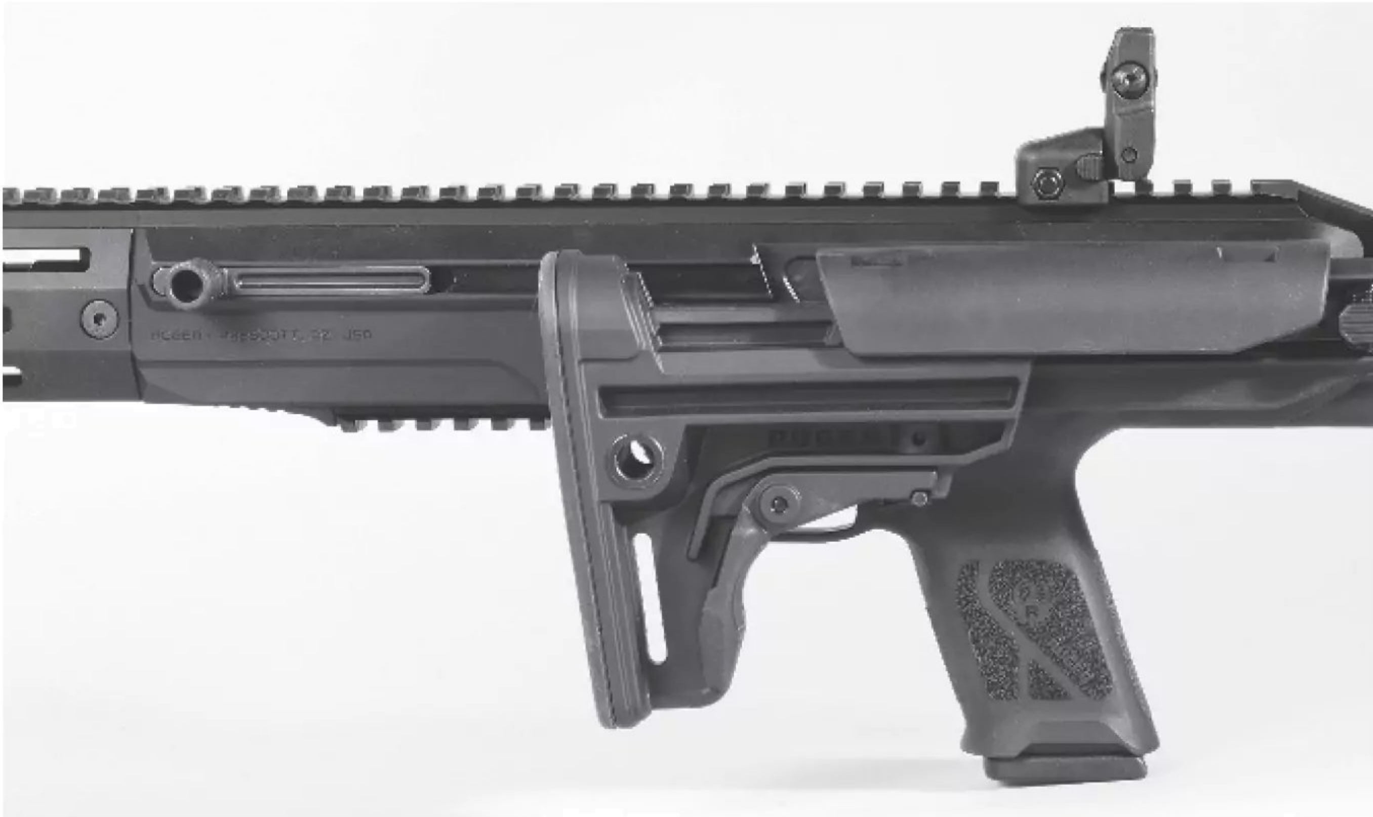
The folding stock makes the gun easy to transport and store. The charging handle is reversible, and the carbine sports a full-length optics rail—although the flip-up aperture sights are excellent in their own right.
