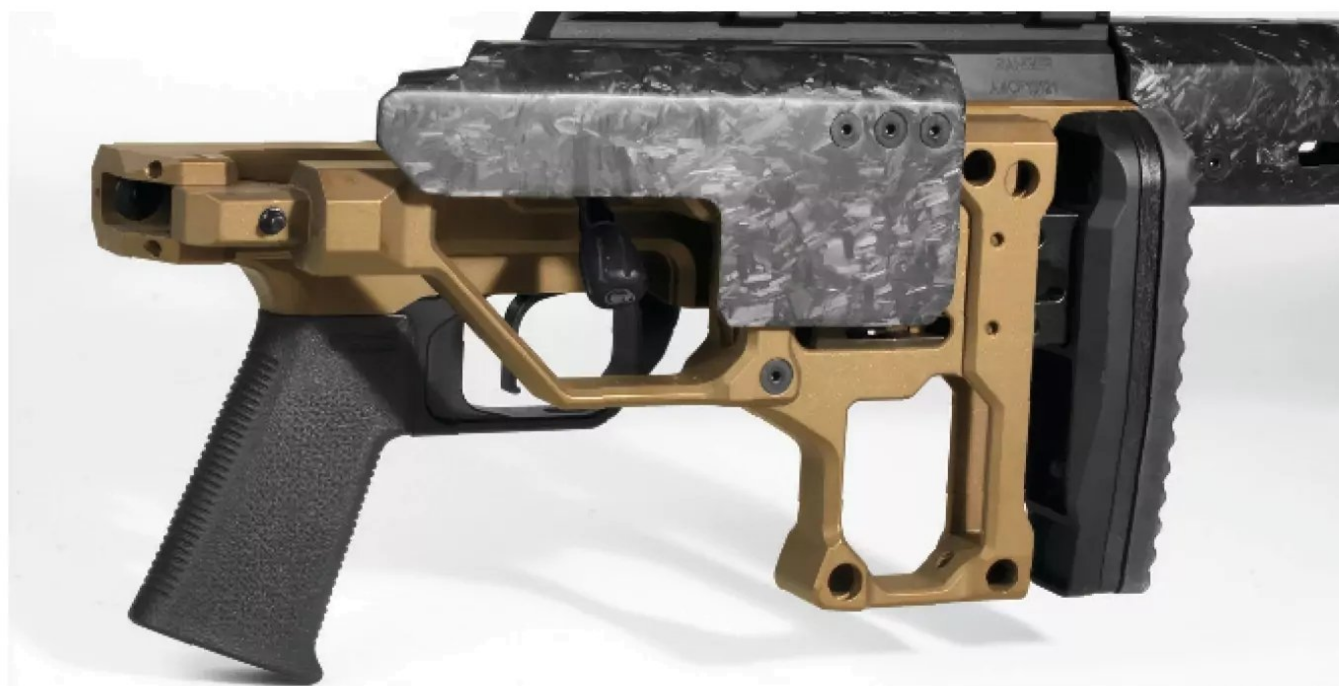
The stock folds with a simple press of a button on the left side, and it locks up courtesy of a strong magnet that keeps the stock folded without the need for a mechanical latch.
