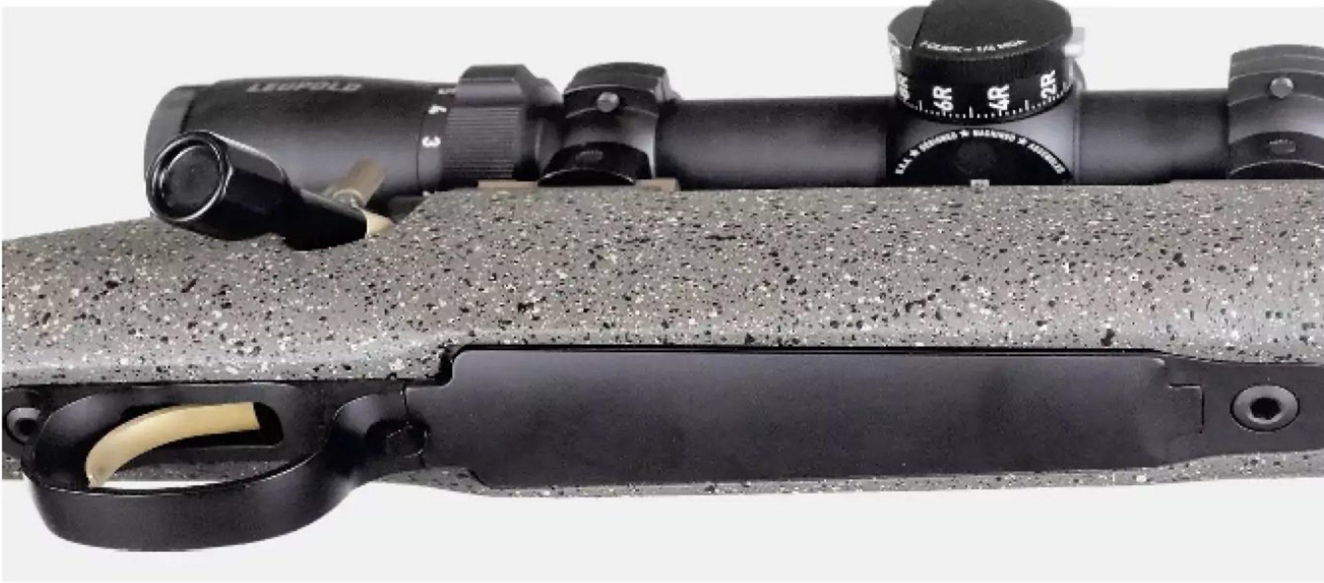
The black hinged floorplate's release is located at the rear of the floorplate, similar to a Model 70. The adjustable trigger sports a gold finger lever.
