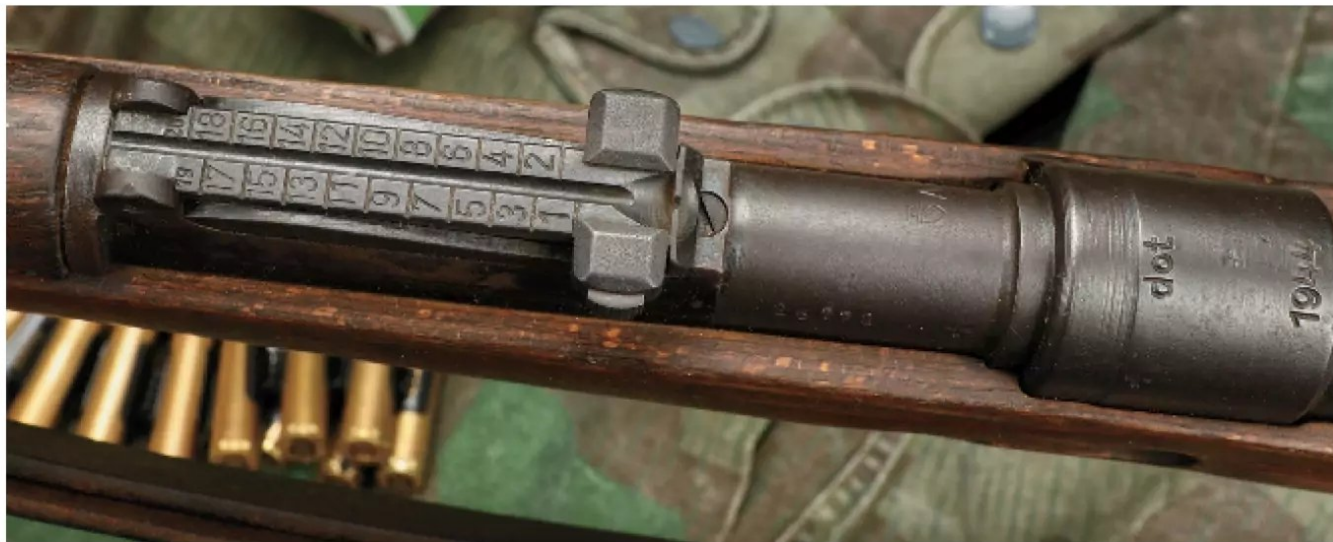
The rear sight matches the front with a V notch sensibly beginning at 100 meters to an optimistic 2,000 meters but is not windage adjustable. The front sight (below) is a simple inverted V post in a base offering minimal windage adjustment.
