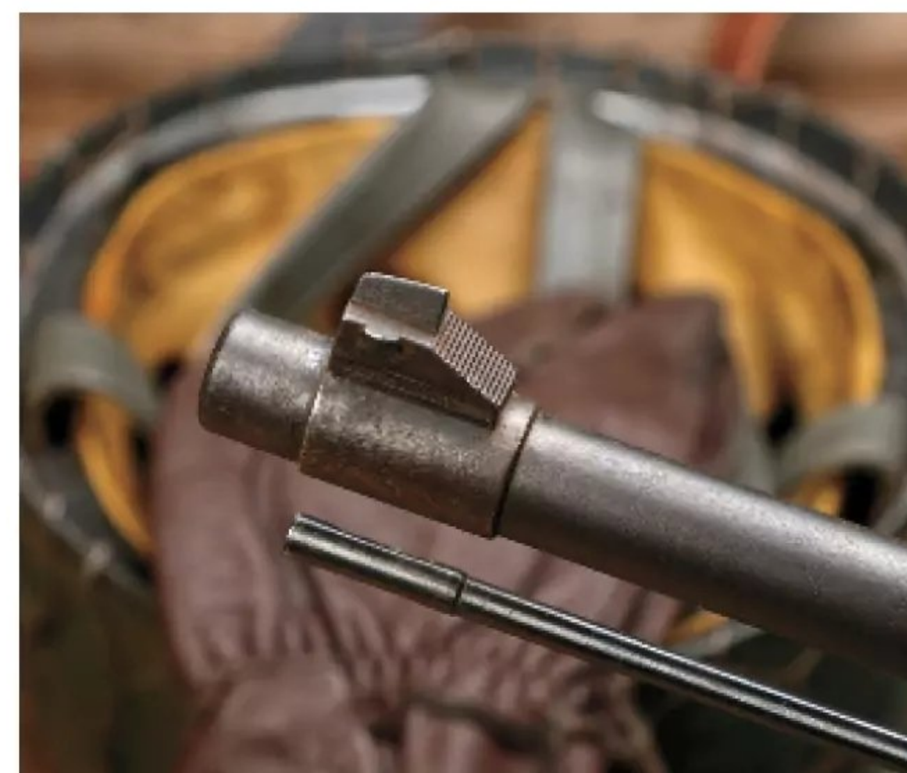
The rear sight matches the front with a V notch sensibly beginning at 100 meters to an optimistic 2,000 meters but is not windage adjustable. The front sight (below) is a simple inverted V post in a base offering minimal windage adjustment.
