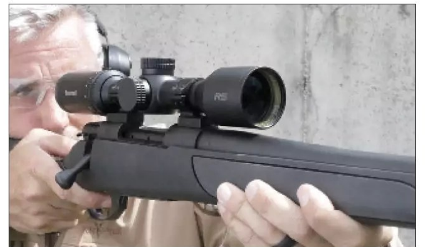
The windage and elevation knobs are capped, which is traditional for hunting scopes, and the side-focus knob doubles as the illumination control. (Below r.), the R5 offers a generous four inches of eye relief, and the 40mm objective (below l.) permits a low mount.
