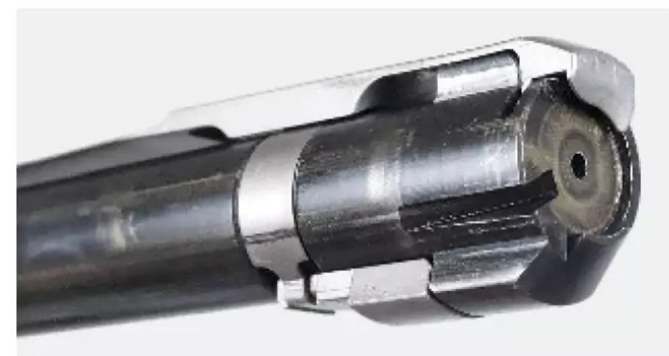
The non-rotating extractor features a relief cut that allows it to slip over the rim of a cartridge without damage, so the rifle can be single-loaded.
