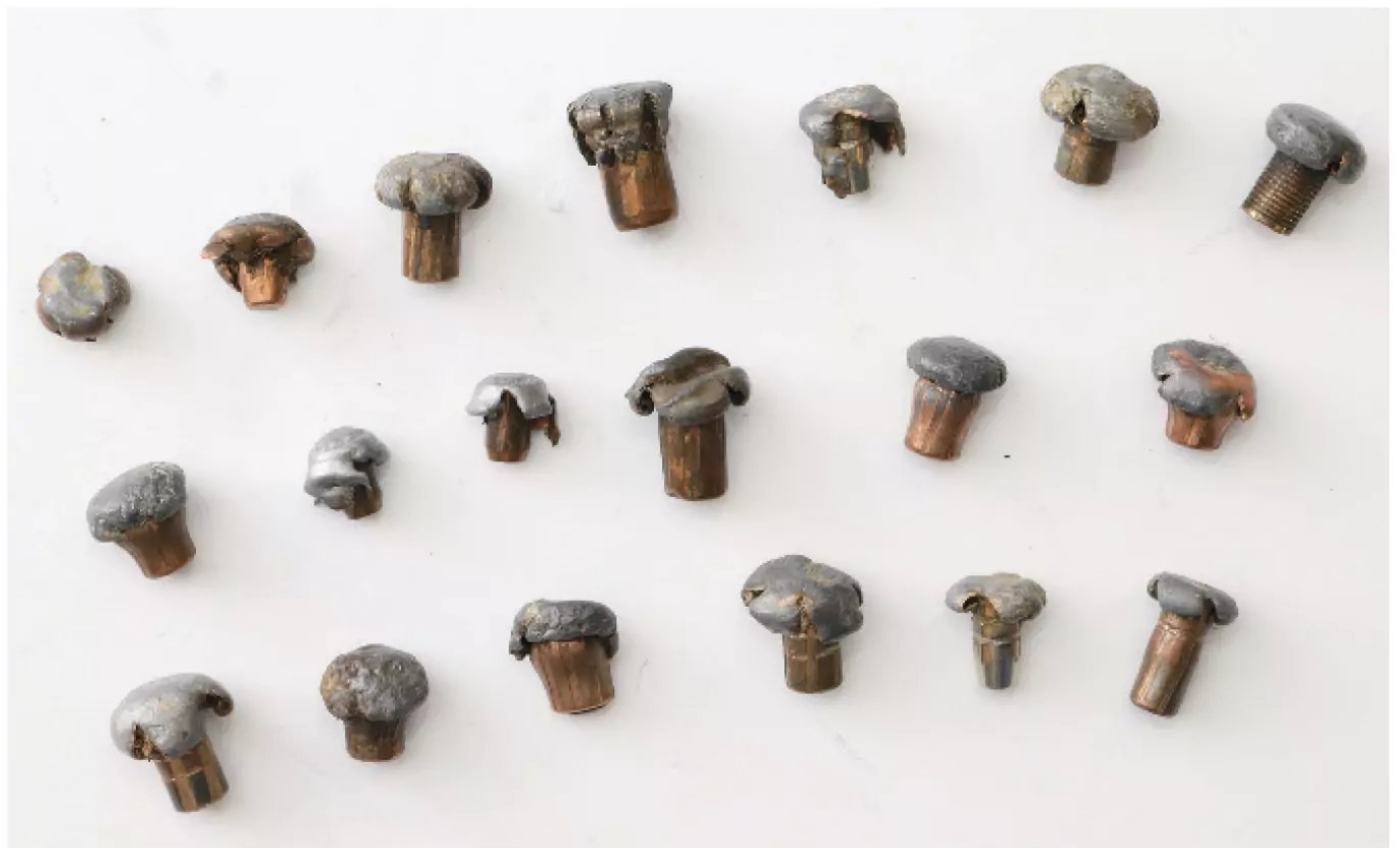
Bonded-core bullets probably create the widest-diameter mushrooms, plus high weight retention. However, they're not as likely to exit, if that's what you're after.
