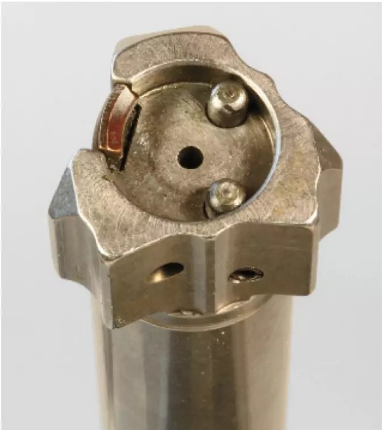
The bolt now boasts two plunger ejectors instead of a fixed blade.
