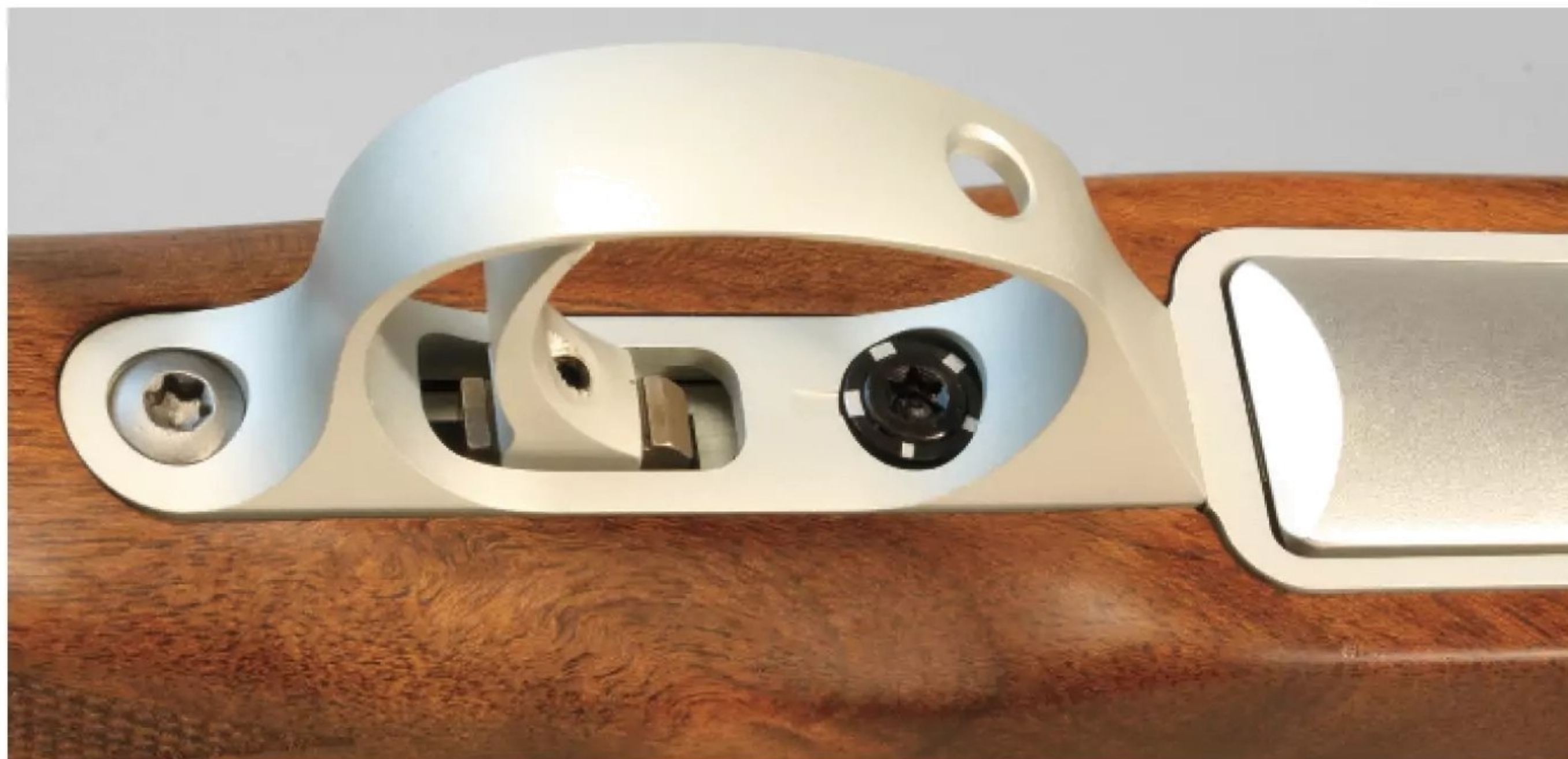
The adjustable trigger has five preset pull weights that can be changed without removing the barreled action. Loosening a set screw in the finger lever allows it to move on its rail to customize trigger reach.
