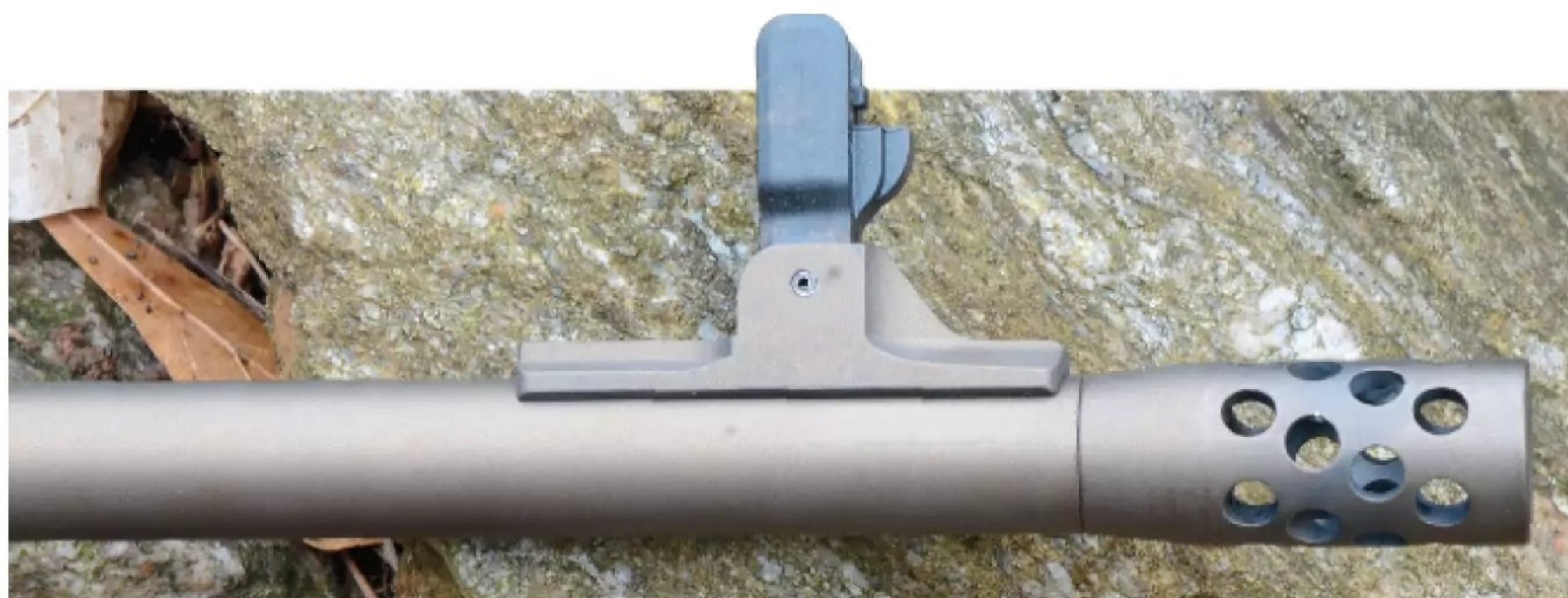
When flipped up, the elevation-adjustable front sight presents a post. When down, it brings a blade with white dot in view.
