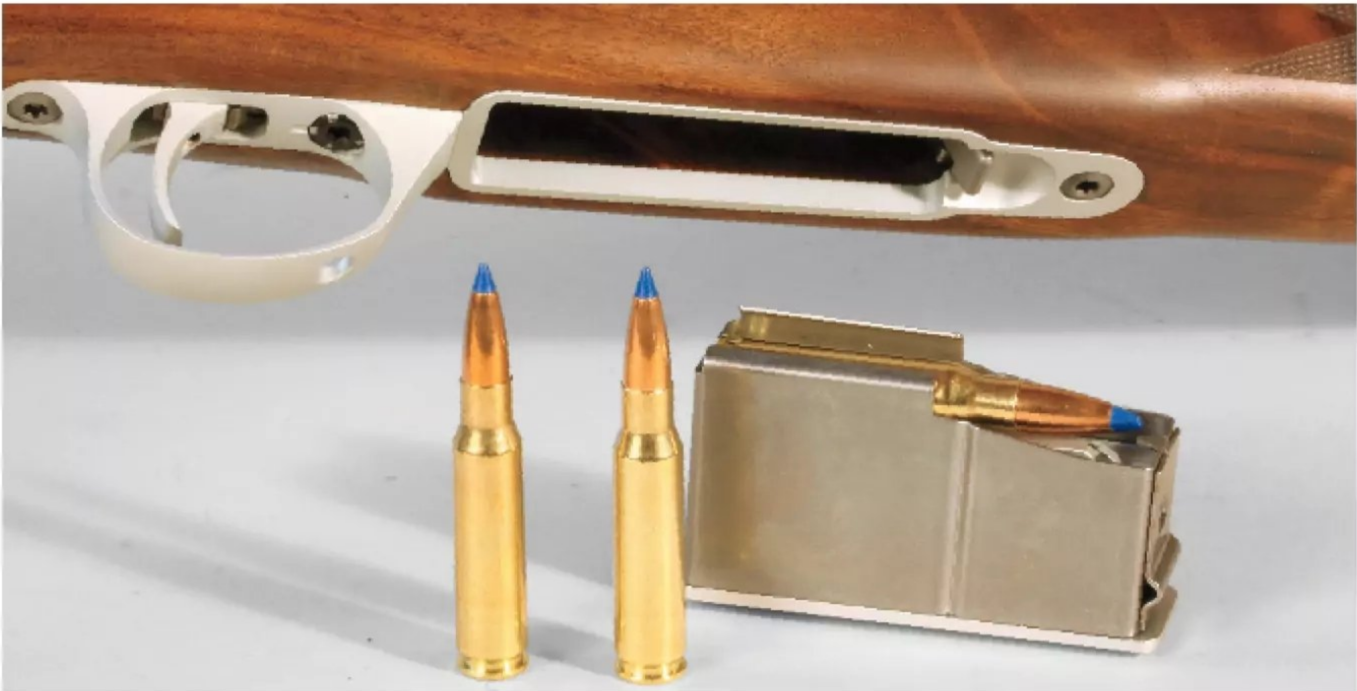
The detachable box magazine holds five rounds and is secured via Sako's Total Control latch. The magazine must be pushed in before operating the release, a system that ensures the mag can't fall out accidentally.
