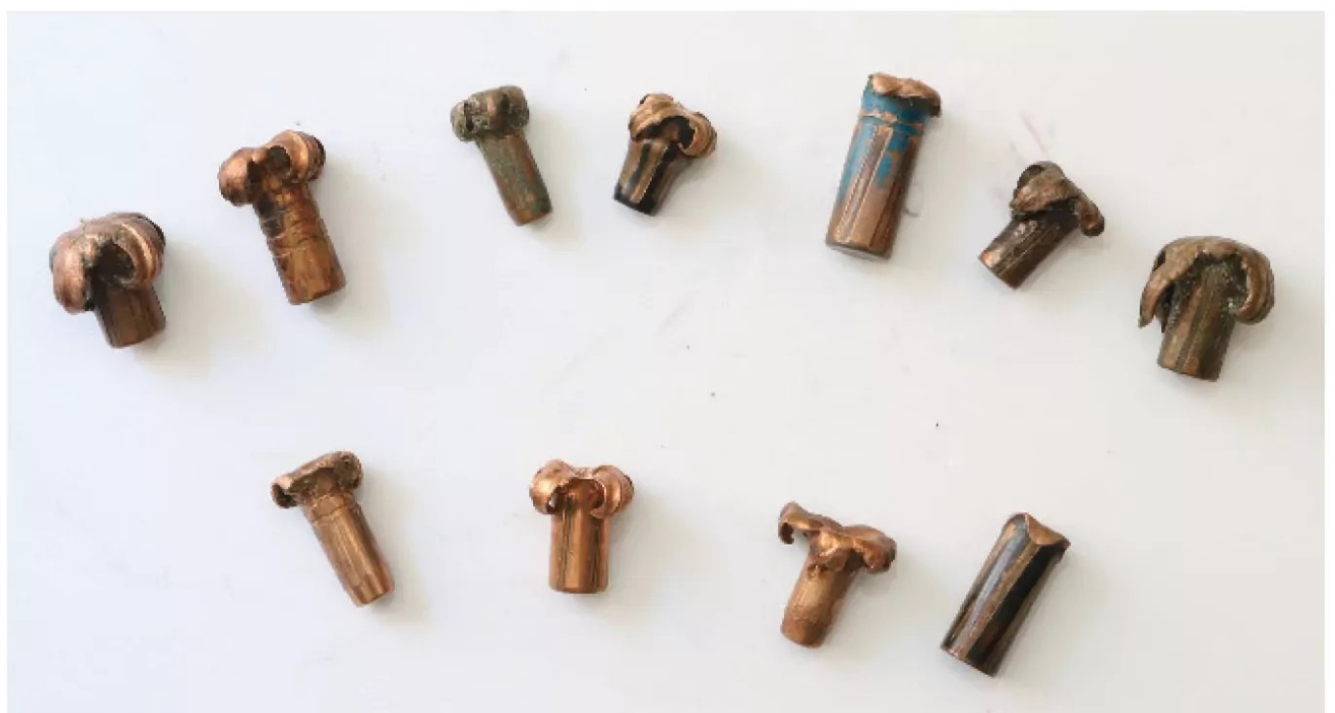
Copper-alloy bullets are typically the deepest-penetrating expanding bullets. They generally retain almost all their weight unless petals break off, which does happen.
