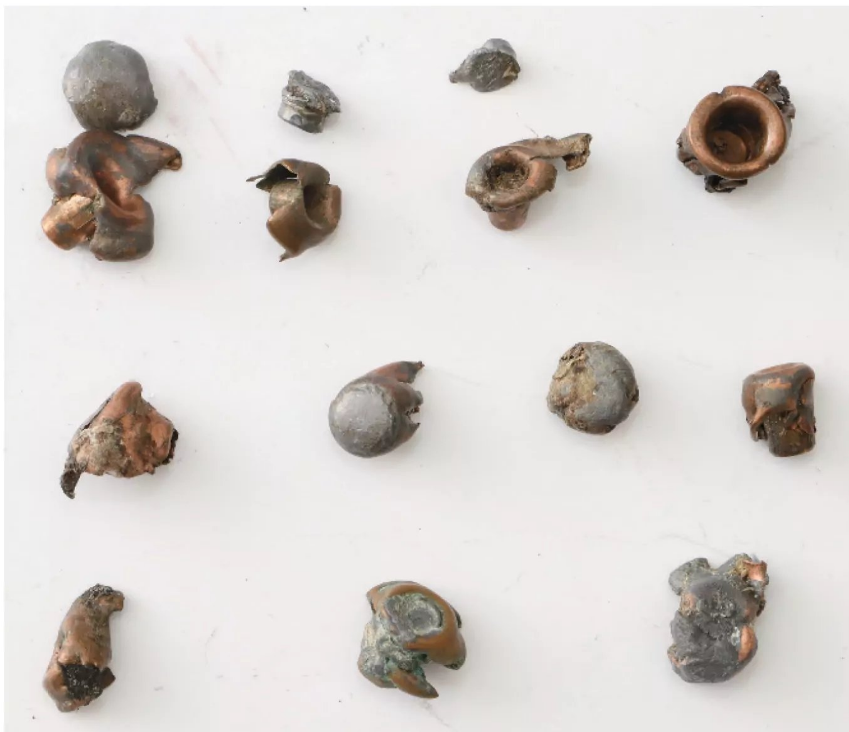
Cup-and-core bullets are going to shed some weight, and it's not uncommon for jacket and core to separate. But they're hard to beat for most deer-size game in most conditions.
