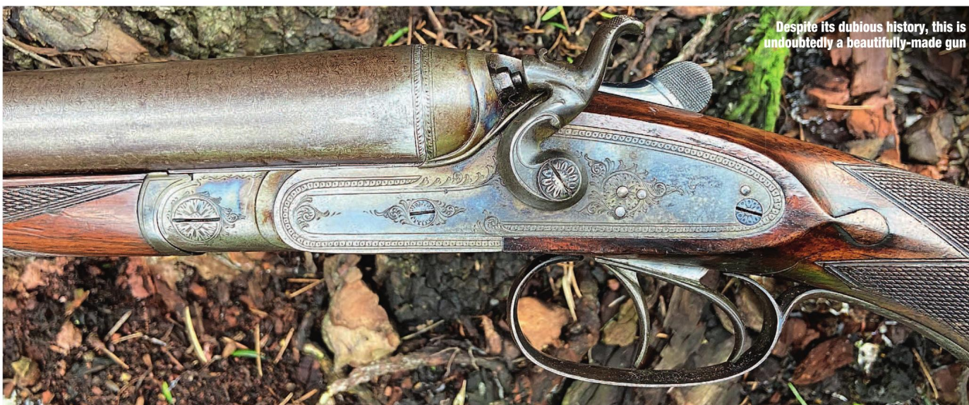
The extractor action is totally different than what you might expect, acting on a stud on the knuckle
