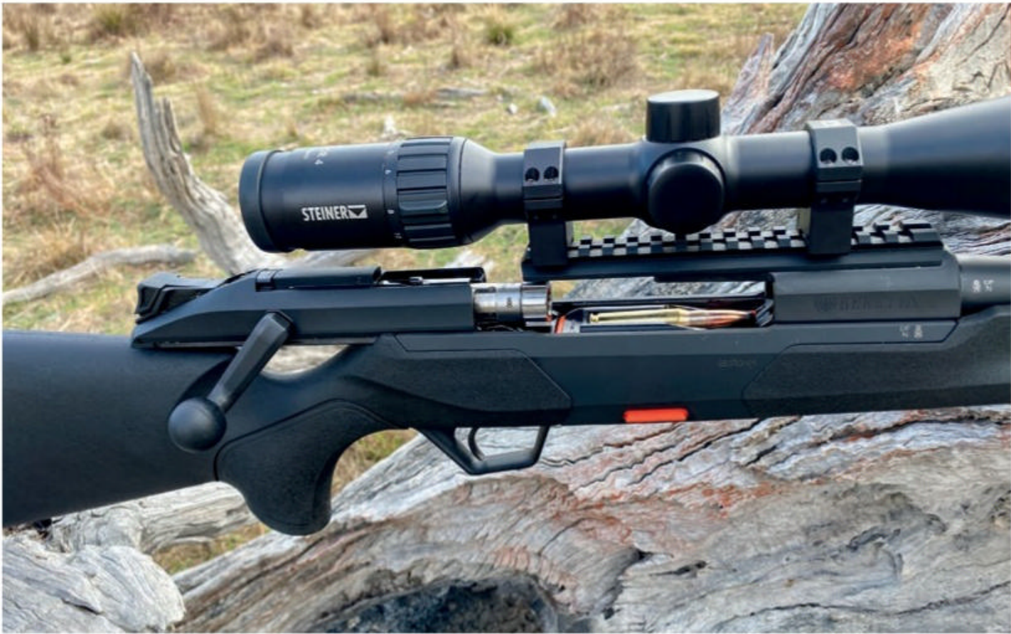
ABOVE: The bolt carrier shown in the rear position to reveal a strong eight-lug rotating bolt head. The massive bolt carrier runs on steel rails incorporated into the chassis
