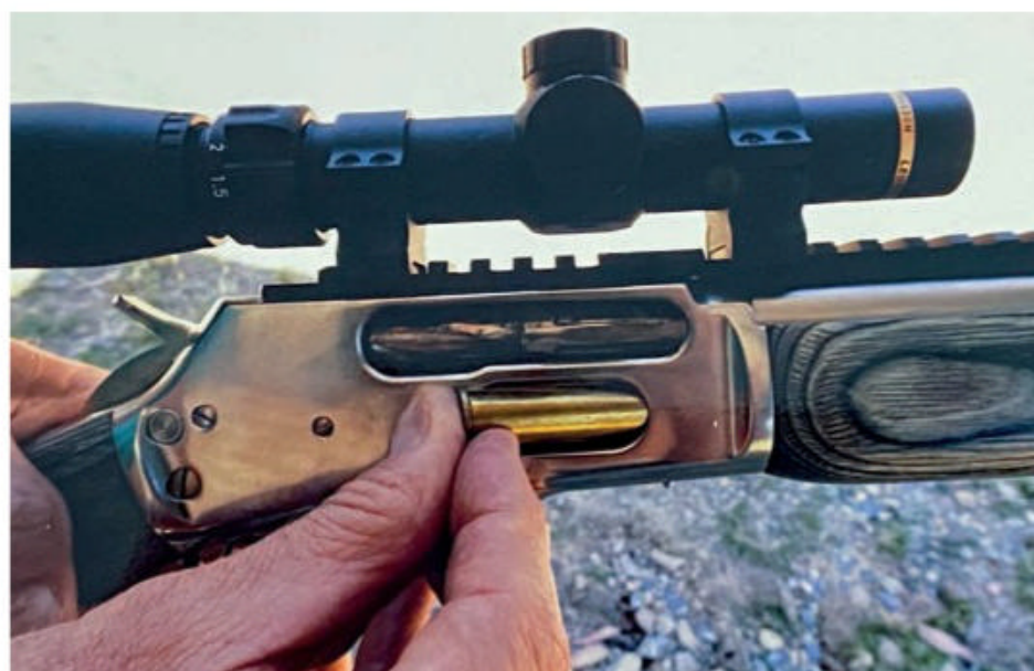
Lead bullets seldom give problems in the .45-70, but the recommended overall cartridge length must be right to work flawlessly through the action
