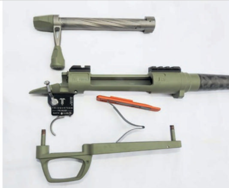
ABOVE: The rifle taken down showing the fluted bolt and squarish trigger guard with alloy follower and drop-out floorplate
