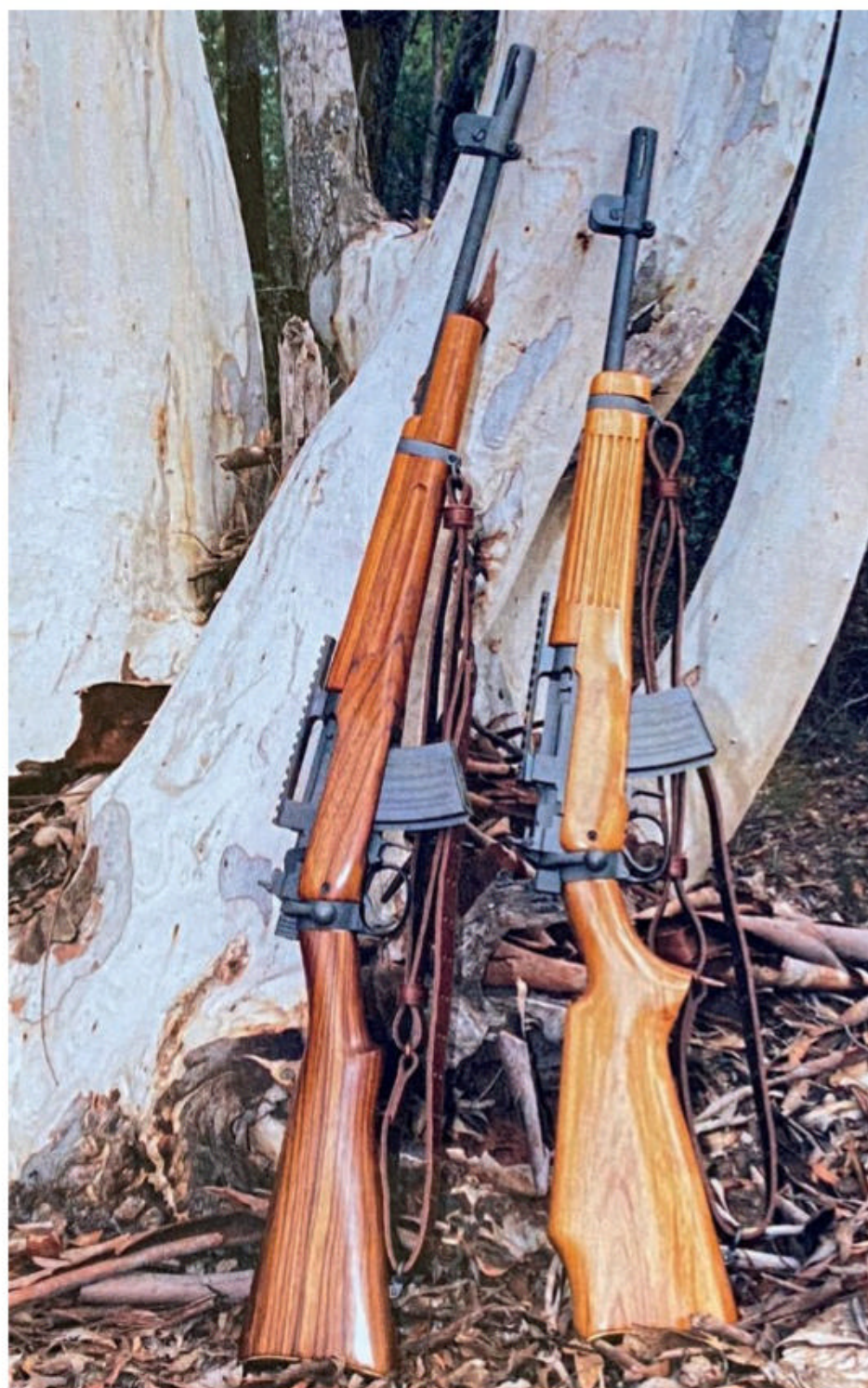
ABOVE: Made in Ishapore, India, the M10 No 4 Lee Enfield sporters showed fine workmanship and good wood. The muzzle has a flash eliminator and a front sight with protective ears
