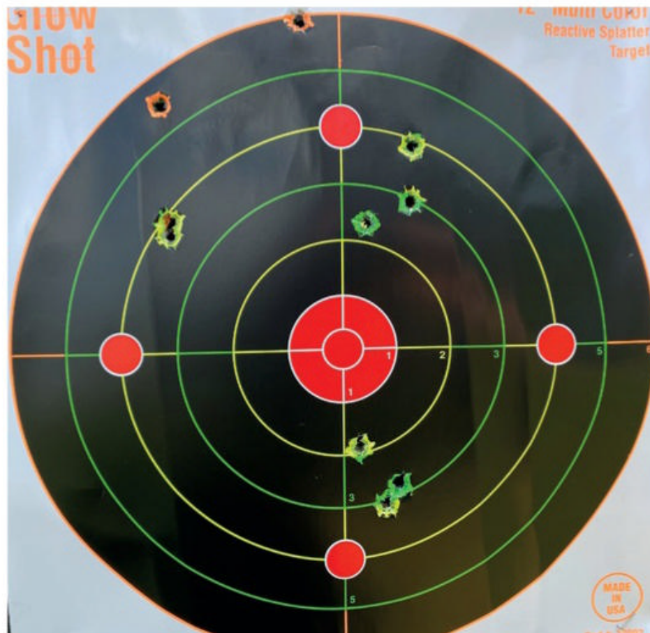
ABOVE: Same rifle, three bullet weights, three very different groups with different points of impact. The top-centre shot was a sighter, the three shots to the left were one group, the three at upper right were another group, and the three at lower right were the best group.
