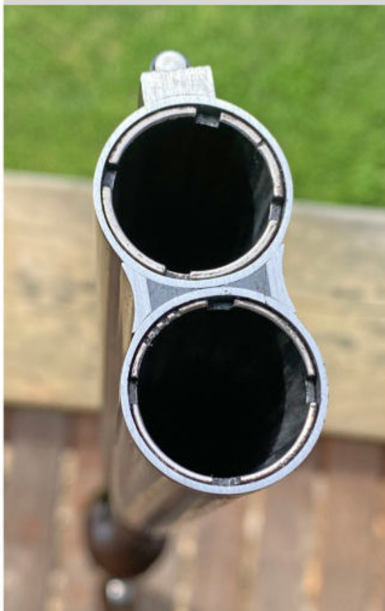
The lower barrel of an over-under shotgun is usually fired first, using a more open choke.
