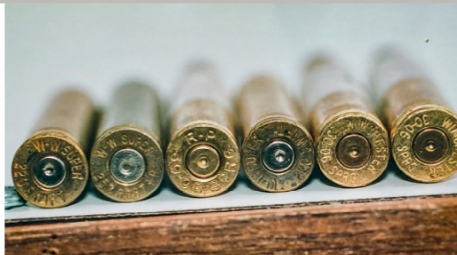
Primer cups vary in hardness and show different degrees of flattening and indentation with the same powder charge.
