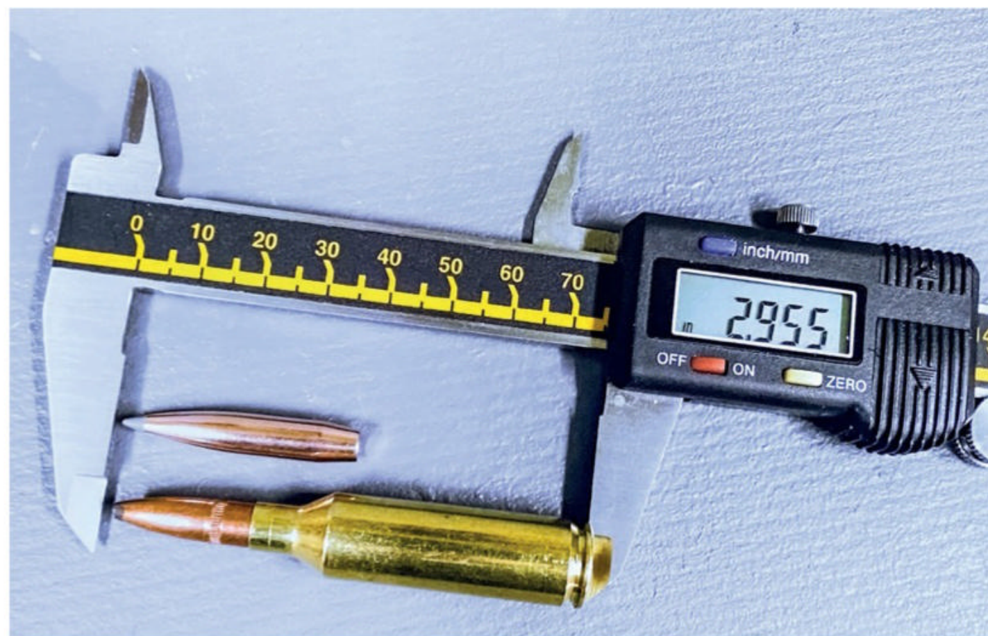
The 120gr Core-Lokt is seated level with base of neck. COL is 2.853". Long Nosler 142gr ABLR extends below the shoulder and COL was 2.925" in the Mauser M18.
