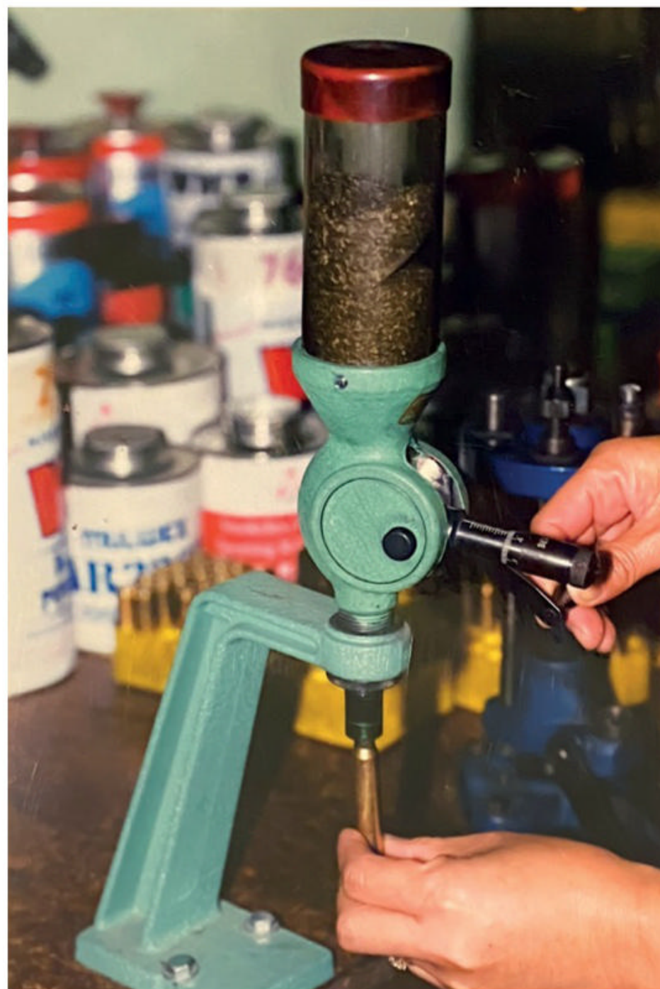
A surface coating of graphite helps powder granules flow smoothly through a volumetric measure.
