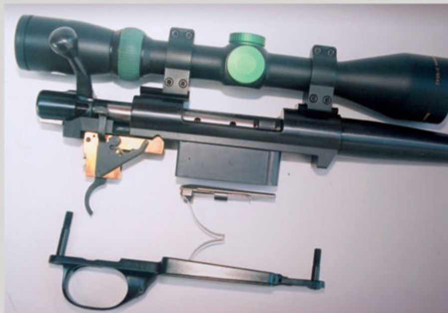
The Howa 1500 shares a good many features with the early Sako rifles. The action is slim and trim, has an integral recoil lug and excellent trigger.
