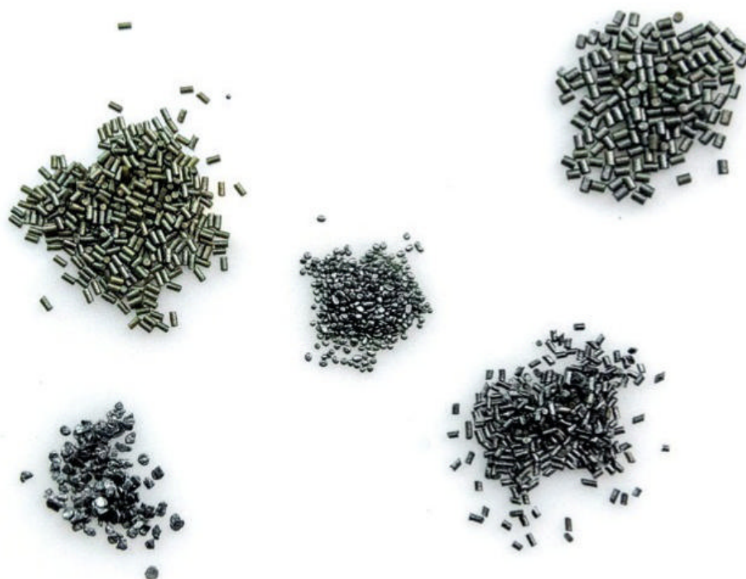
Granules of different powders for various uses. Bottom left and centre are flake powders, the others are extruded stick types. The centre and bottom right powders are out of .223 cartridges, while at top right you see AR2206H, which is also ideal for the .223. Bottom left is a fast-burning powder from a shotgun cartridge. Top right is slow-burning AR2225.
