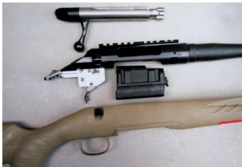
Ruger American cuts cost by having a cylindrical receiver, one-diameter bolt, recoil lug in stock and detachable polymer magazine.
