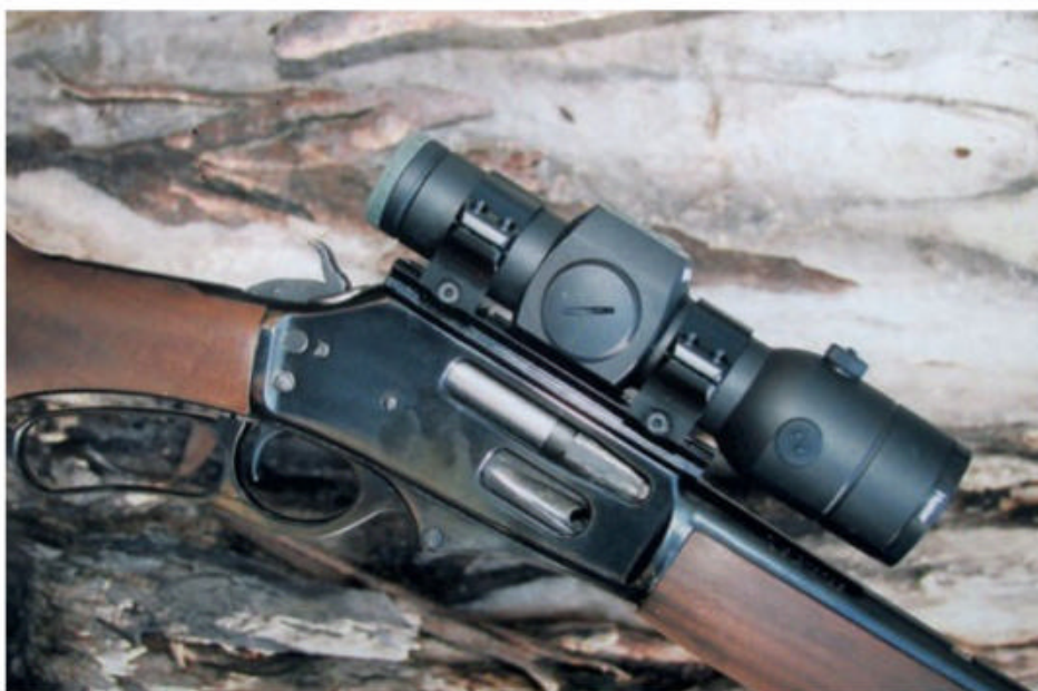
Rossi Rio Grande has a solid-top receiver and side ejection copying the Marlin's time-proven Model 336 design.
