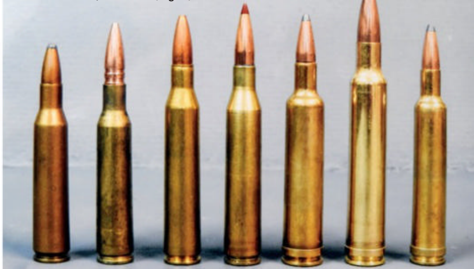
L to R: Factory seated bullets in the .257 Roberts and .25-06 show bullets seated out to take advantage of freebore. The .257 and .300 Weatherby chambers have 3/8" freebore, but .240 (right) has a standard throat
