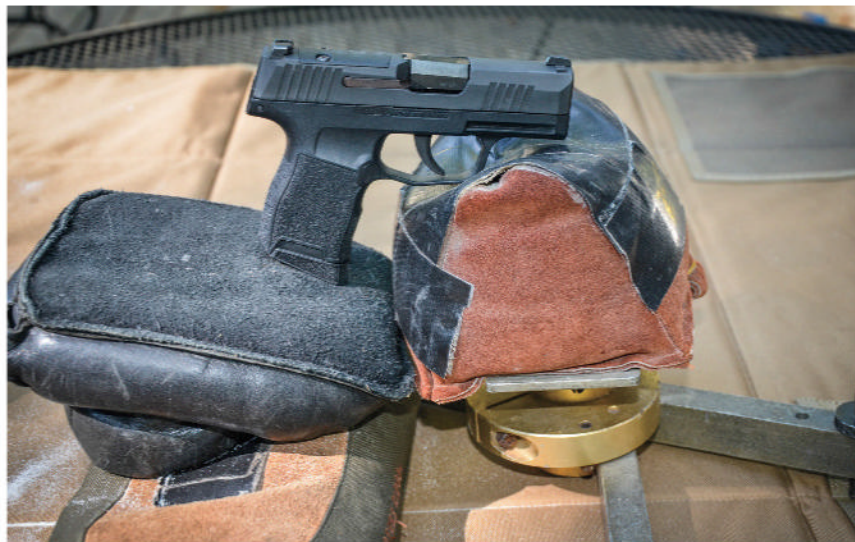
Layne uses a large sandbag (protected by Gorilla Tape) attached to a rest he purchased when he was in high school along with a bunny ear sandbag positioned bottom side up when testing small autoloading pistols like the SIG SAUER P365. The same combination works equally well for shooting small revolvers.
