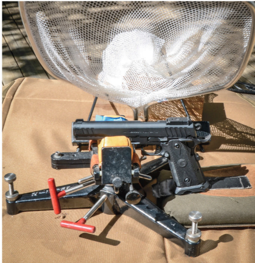
The Sinclair front rest and a flat sandbag are also used for accuracy-testing large autoloading handguns, such as this EAA double-stack 1911 in 10mm Auto. The Universal Brass Catcher from Brownells eliminates the chore of picking up spent cases after a shooting session.
