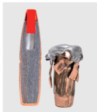
The 307-grain SUB-X bullet penetrated 16 inches in ballistic gelatin, with the bullet beginning to tumble in the last four inches or so. The recovered bullet is shown next to a sectioned bullet. Photos courtesy of Hornady.
