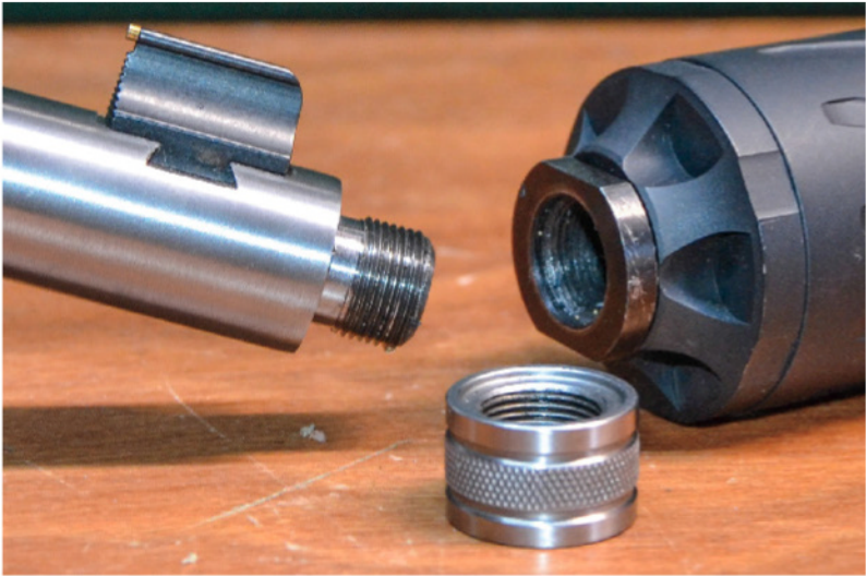
The muzzle has 1/2-28 threads for attachment of a suppressor or a muzzle brake, and a thread protector is included. Note that the gold-bead front sight is dovetailed to the barrel.
