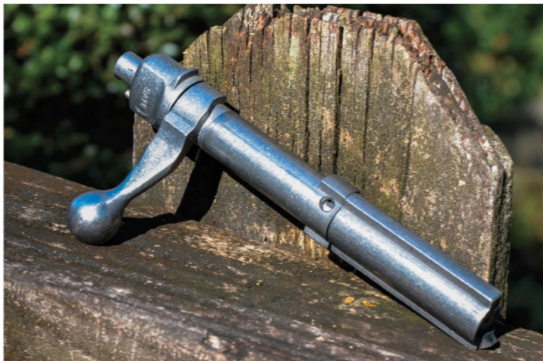
The bolt is a two-piece design with a nonrotating front section containing the extractor and a rear rotating section with two large dual-opposed locking lugs that engage recesses machined into the inner wall of the receiver.
