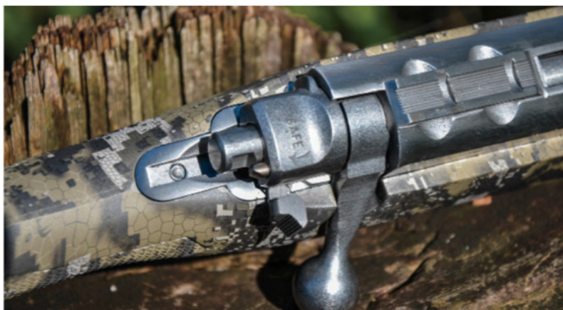
Located at the right side of the receiver, the three-position safety lever is easy to reach, and it can be operated quietly, which is important for a hunting rifle.
