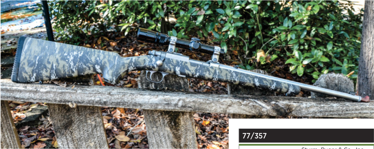
Layne really likes the size and shape of the camo synthetic stock. Note that the top of the stainless-steel receiver is machined for Ruger scope-mounting rings, which come with the rifle.
