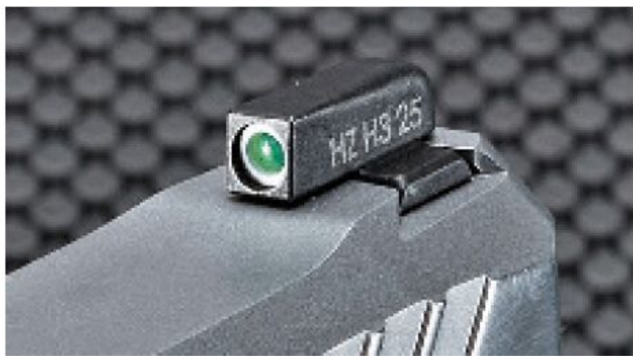
The all-black rear sight has a U-shaped notch, and the front sight has a green tritium dot surrounded by a white ring. Both sights are dovetailed into the top of the slide.
