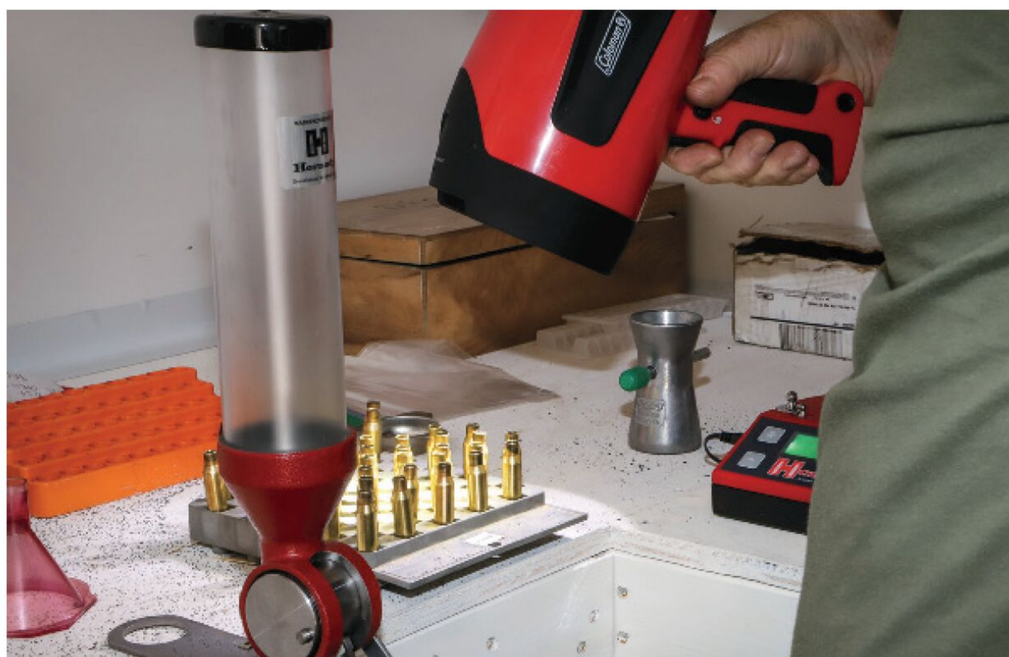
After charging cases with powder, Boddington uses a strong light to visually inspect the powder level in each and every case.
