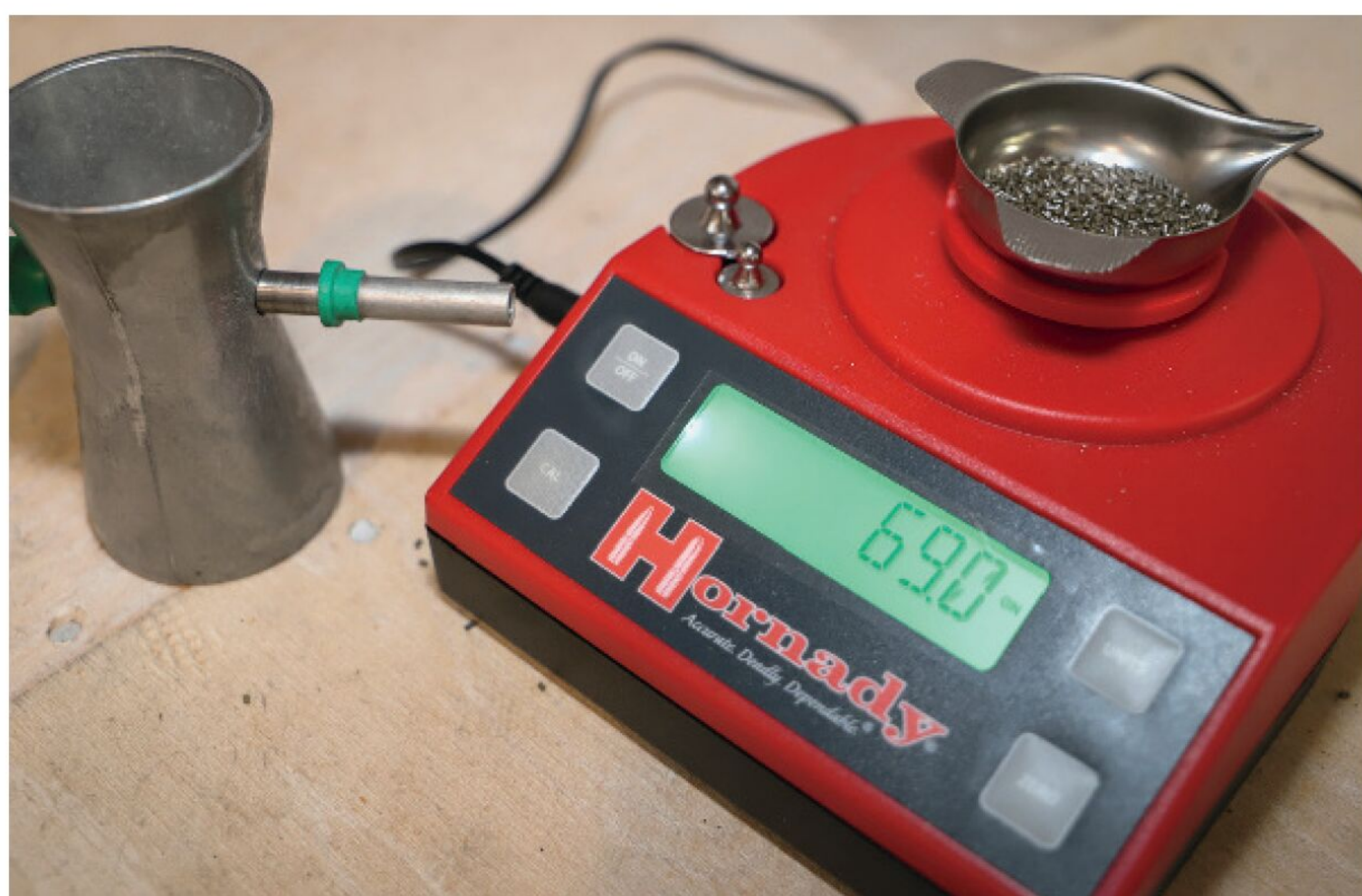
Although modern powder dispensers are wonderfully accurate, Boddington loads hunting ammo as he always has by dispensing low and then trickling in the last few grains to the tenth.
