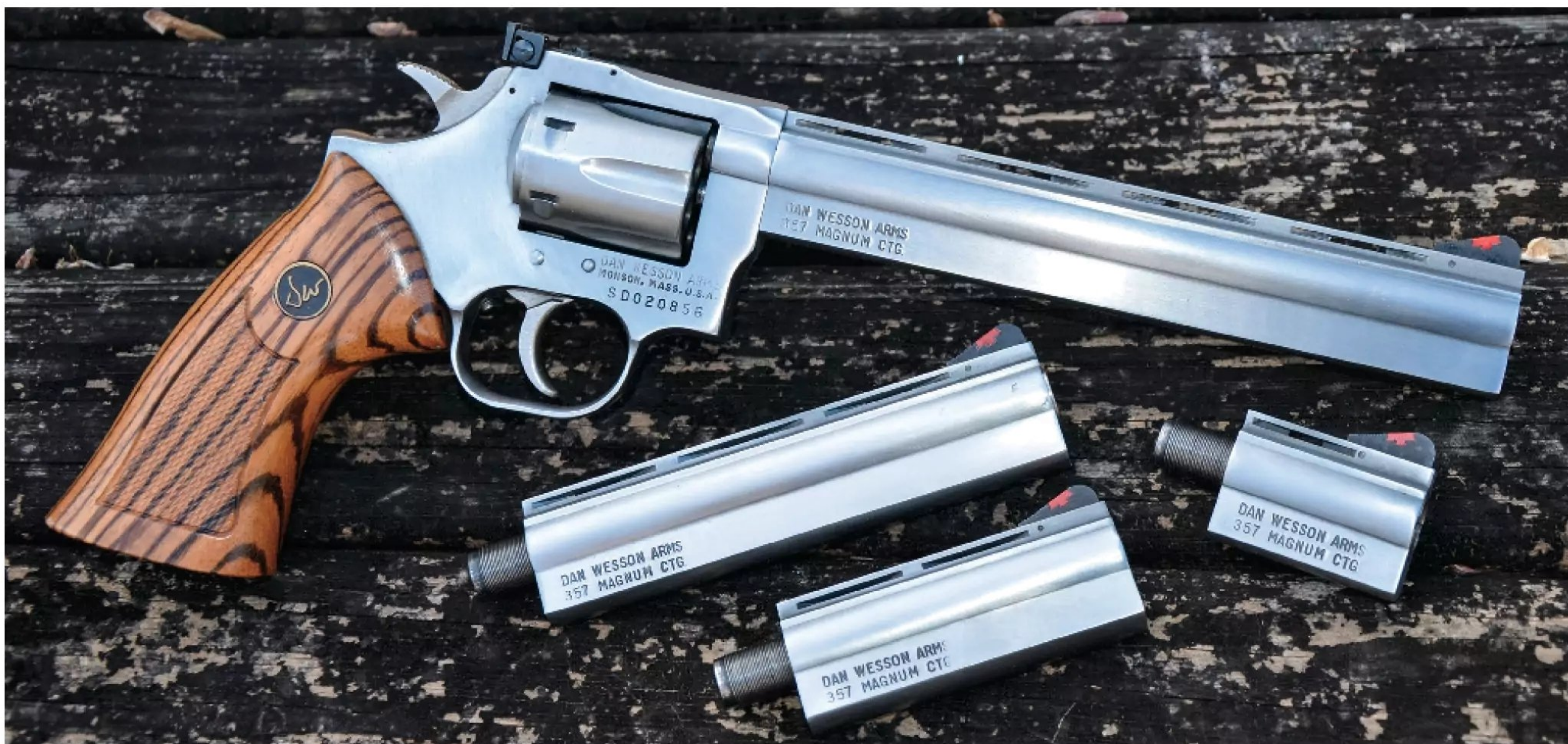
A Dan Wesson Arms Model 715-VH revolver with interchangeable 2.5-inch, 4.0-inch, 6.0-inch, and 8.0-inch barrels was used to test the velocities of full-power charges of W296 behind five Hornady 0.357-inch bullets weighing from 110 to 180 grains.
