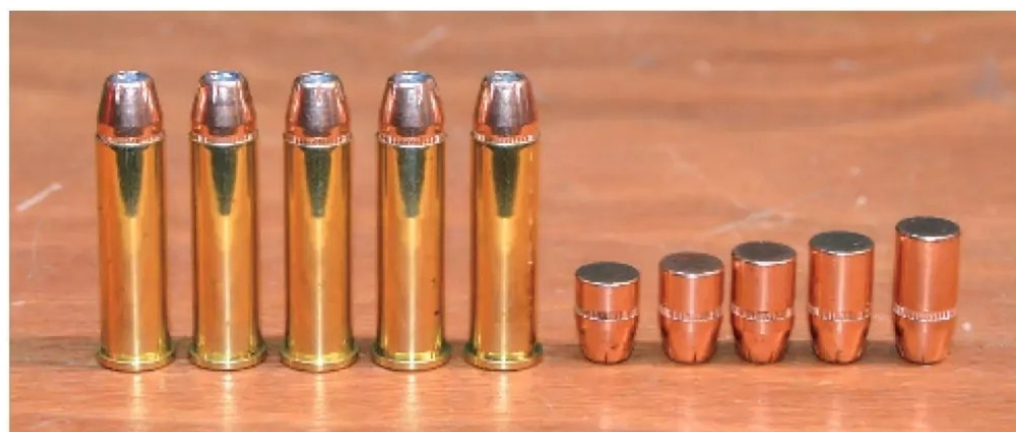
The five upside-down Hornady 0.357-inch XTP bullets at right show that their dimensions from cannelures to noses are the same, while differences in their overall lengths are due to different lengths of their full-diameter shanks. (left to right) Hornady 110-grain XTP, Hornady 125-grain XTP, Hornady 140-grain XTP, Hornady 158-grain XTP, Hornady 180-grain XTP
