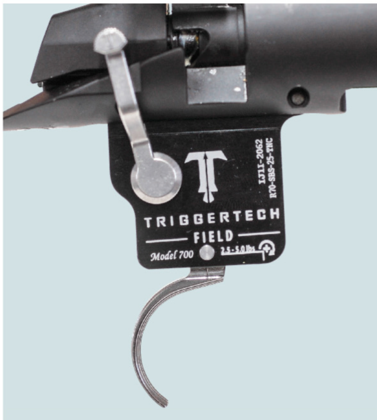
The all-new Model 307 Range XP rifle features a user-adjustable TriggerTech trigger. Steve's rifle's trigger pull averaged 3.12 pounds right out of the box.
