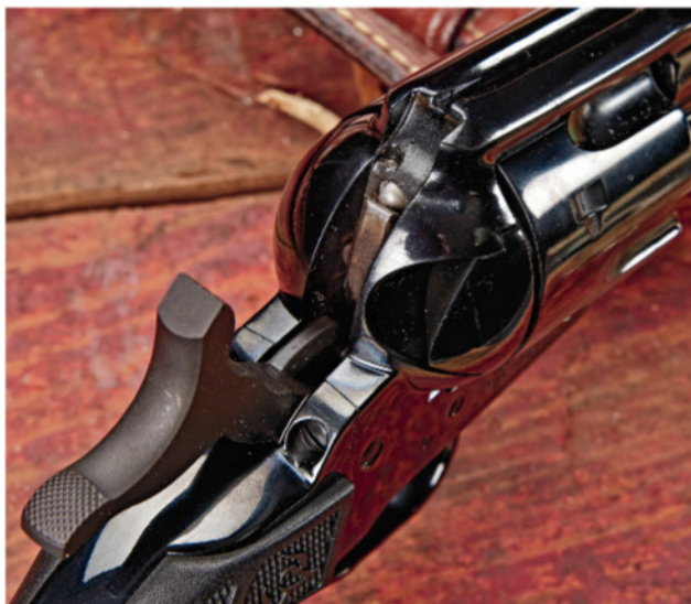
Unlike old, traditional Colt SA revolvers, the Deputy has a transfer-bar firing mechanism with a frame-mounted firing pin.
