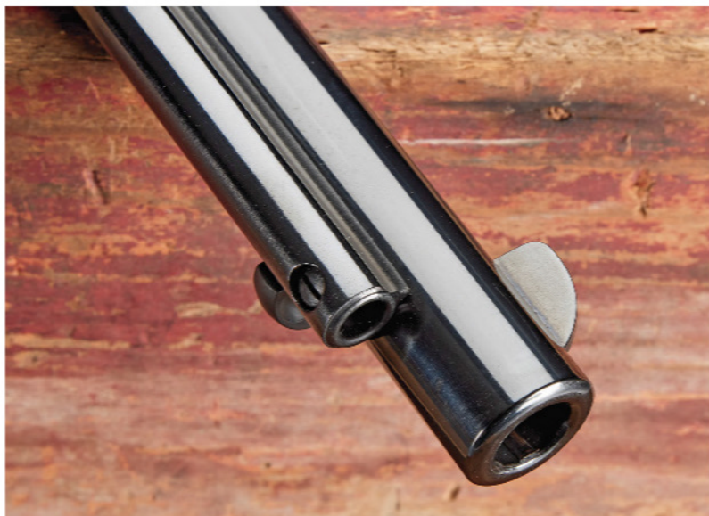
The sights are very traditional, consisting of a groove in the topstrap for the rear sight and a shark-fin blade for the front sight.
