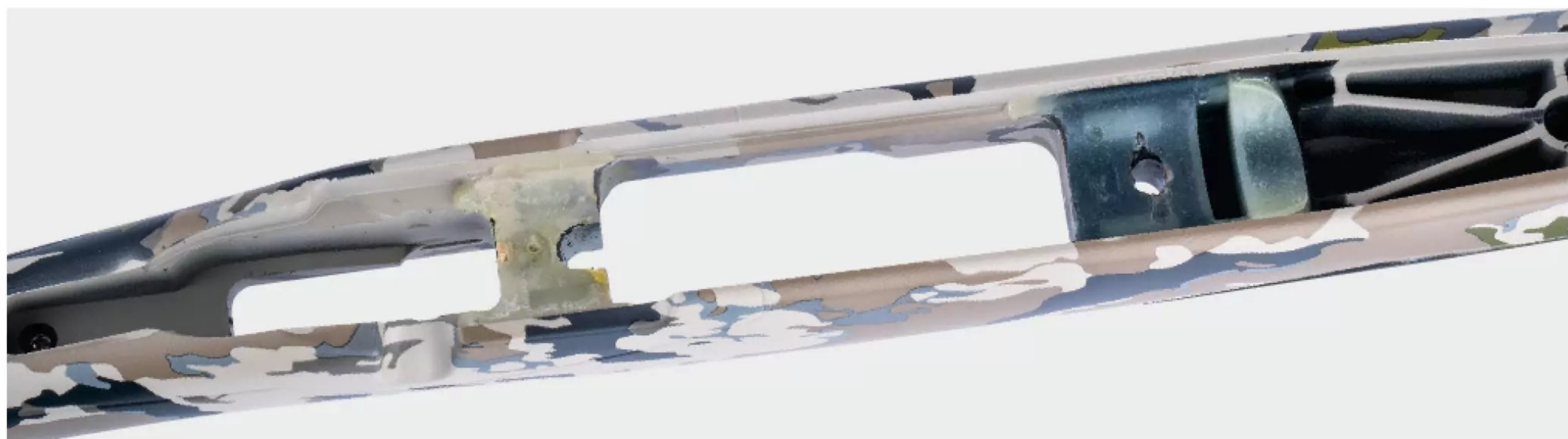
X-Bolt rifles have always come glass bedded. The Gen 2 X-Bolt has well-done glass bedding that provides proper and consistent support for the action.
