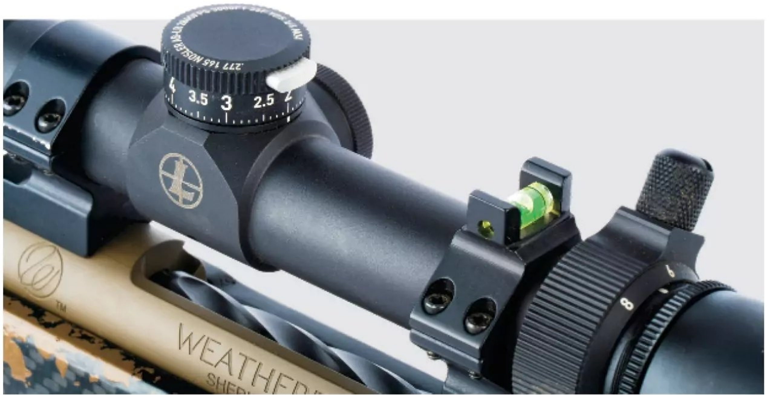
Leupold's CDS-ZL stands for Custom Dial System, Zero Locking. It's an outstanding turret that is low in profile, simple to use, and extremely reliable. Not only does it have a zero-stop, but the silver button is a zero lock so you don't accidentally spin the turret.
