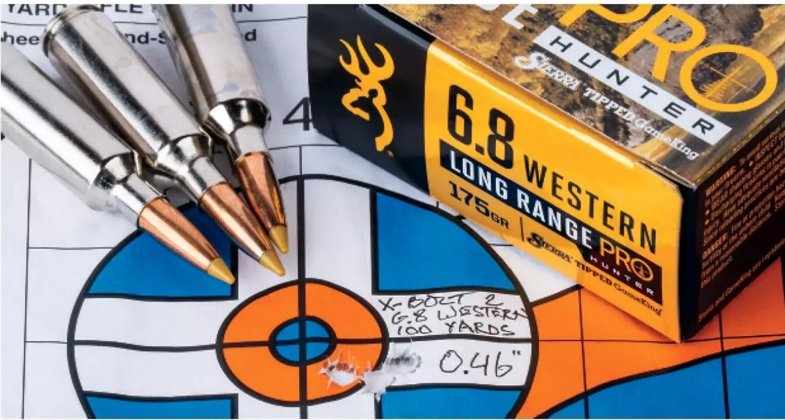
Four of five different factory loads tested averaged well under MOA, and Browning’s 175-grain Long Range Pro ammo averaged just a whisker over 1/2 MOA.
