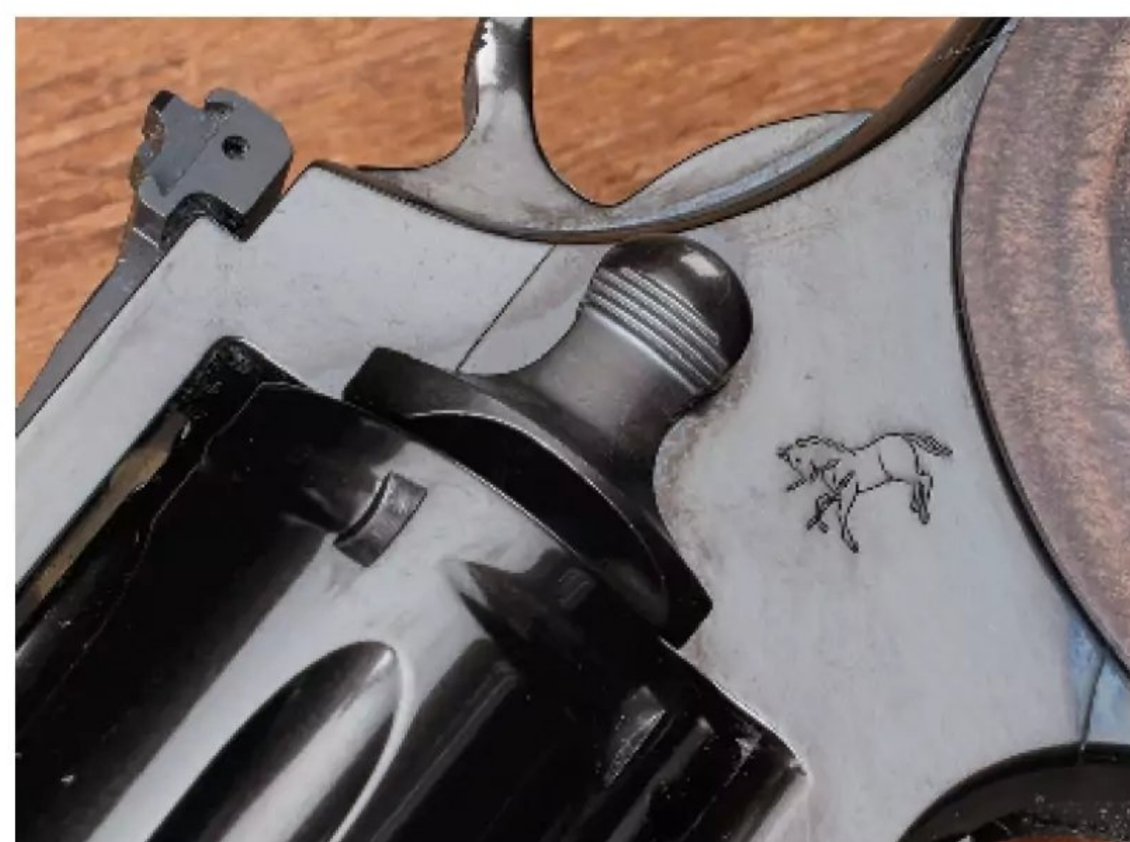
The new Python's cylinder release is shaped just like the original Python's. Pulling the release to the rear allows the cylinder to swing out to the left side.
