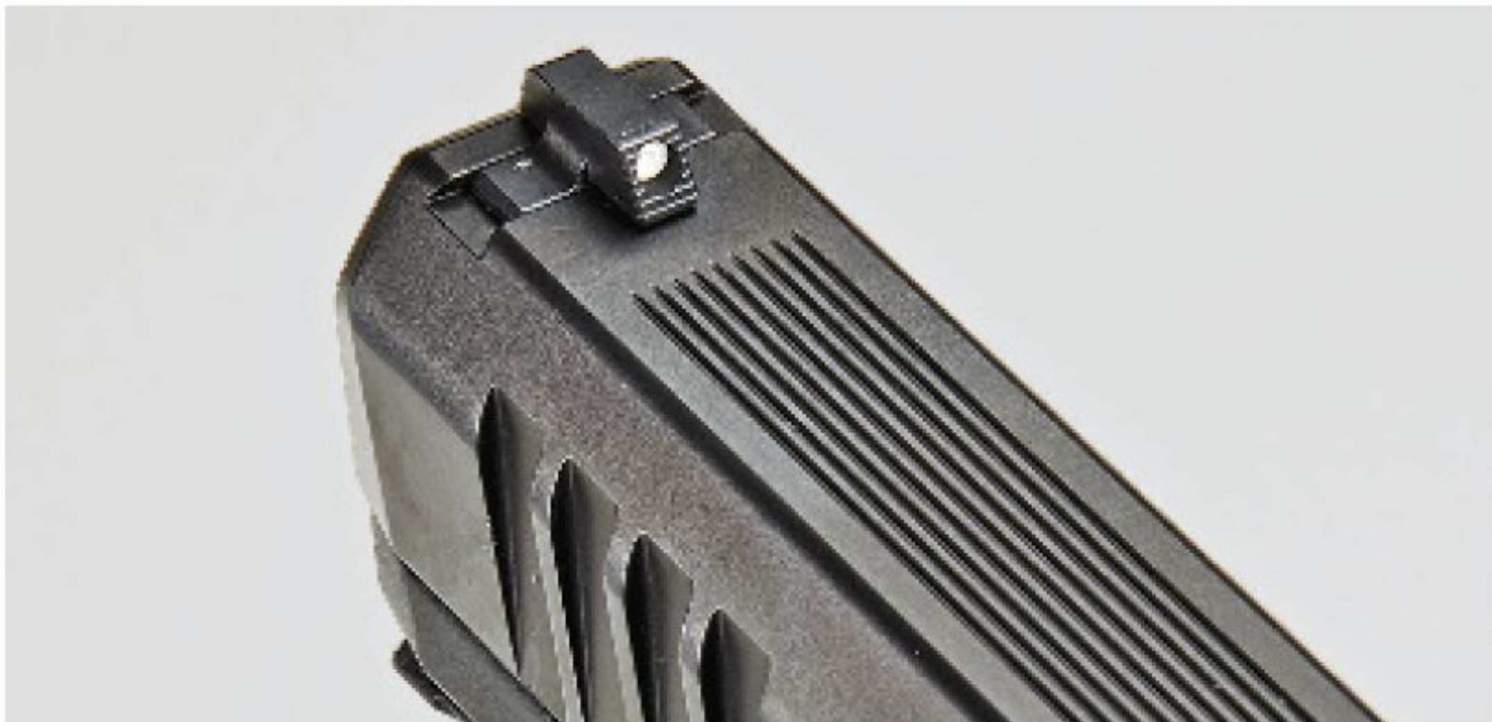
The pistol’s front sight has a single white dot, and the post is angled to facilitate a snag-free draw. Note the glare-reducing striations on the slide’s top.
