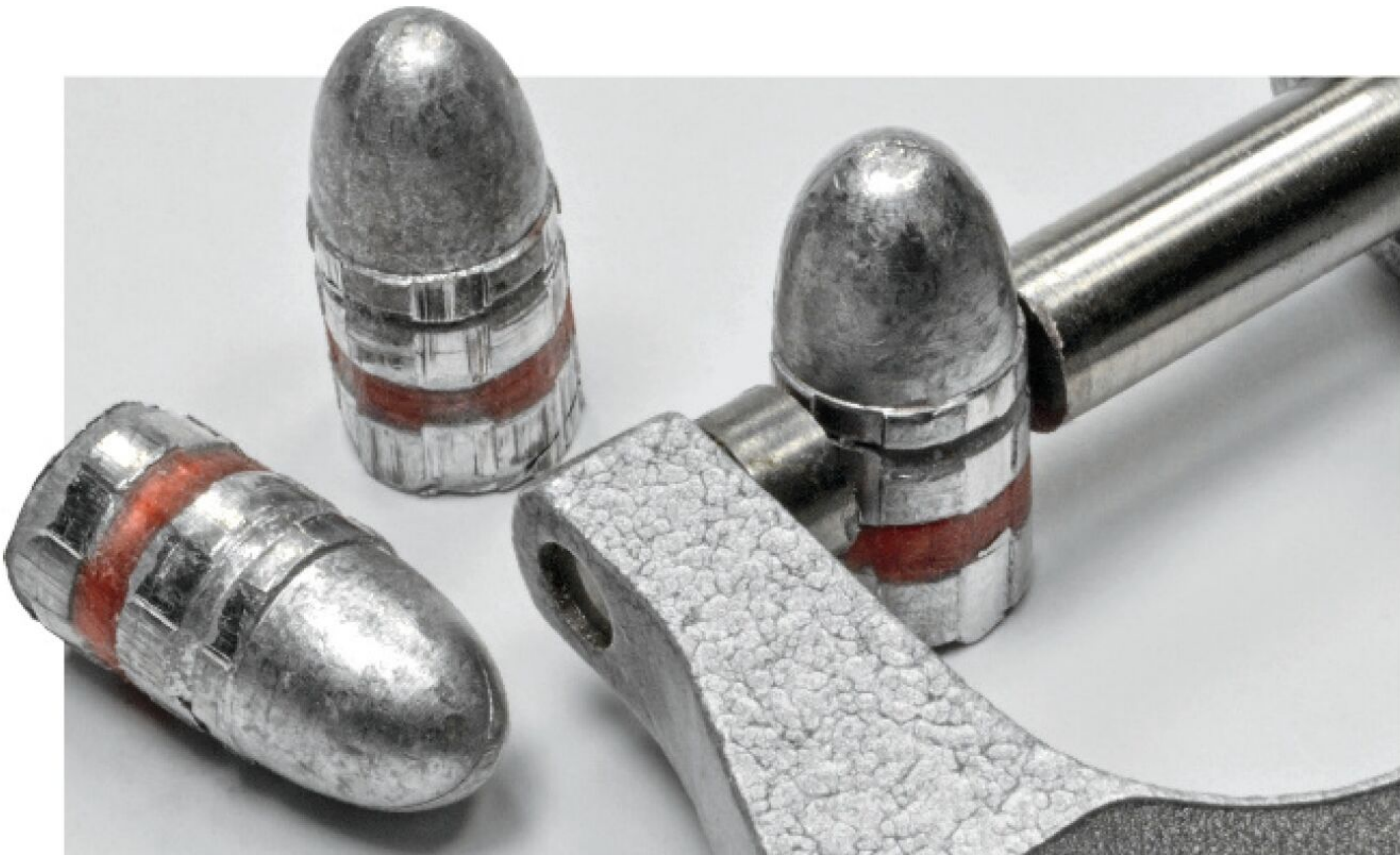
Dr. Miller used soft cast bullets to slug the barrels of 9mm pistols and .38/.357 revolvers for this report.
