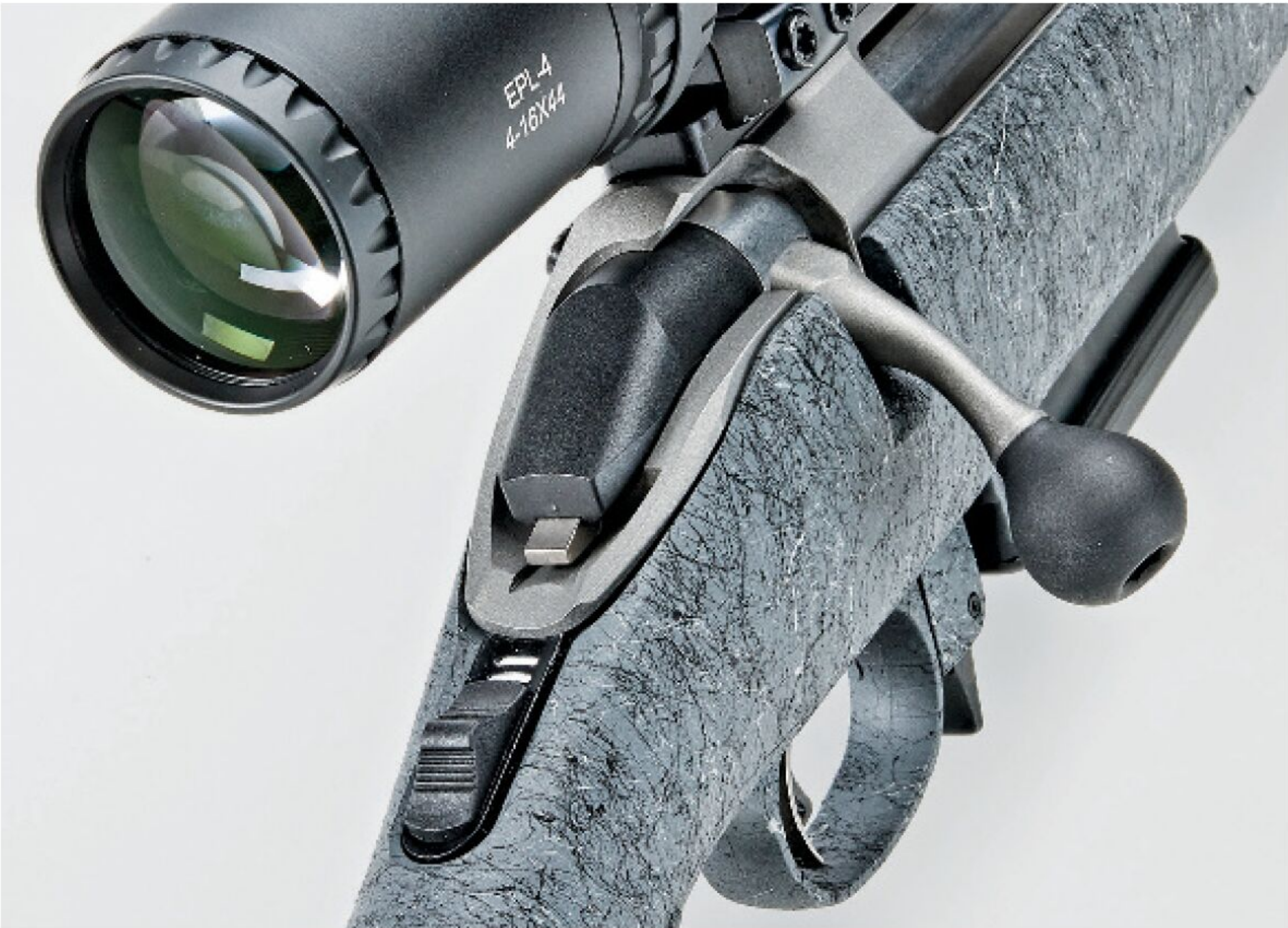
Also new is the Gen II rifle’s safety. It is a three-position, forward-to-fire mechanism. The middle position prevents the trigger from being operated but allows the bolt to open for unloading a chambered round with the safety engaged.
