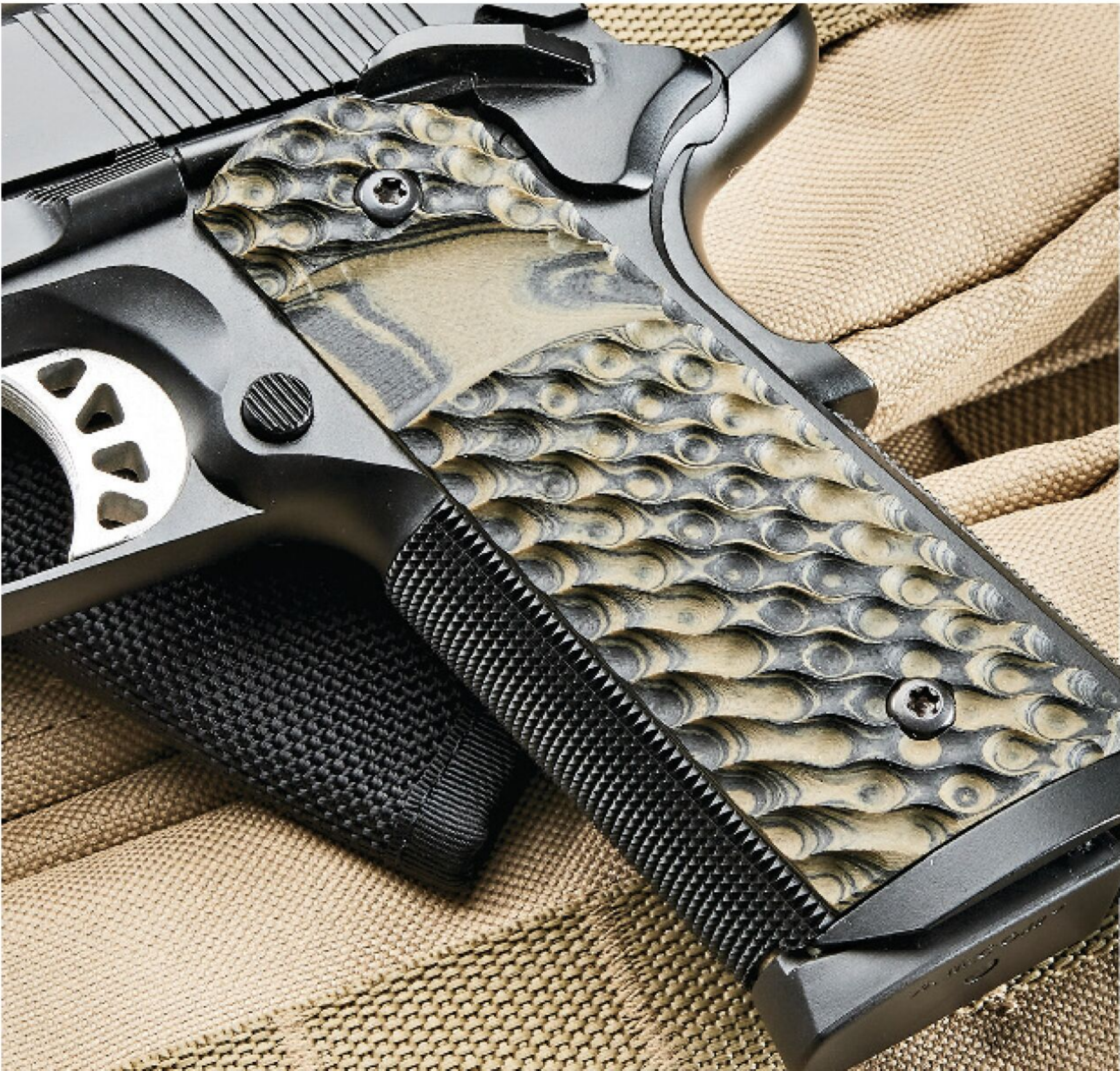
The grips are VZ Hydra G10 grips, and they feature an aggressive texturing pattern and a deep contour for the shooter’s thumb. The grip frame has 20-LPI checkering on the front-strap and the flat mainspring housing. Note the bolt-on magazine well.
