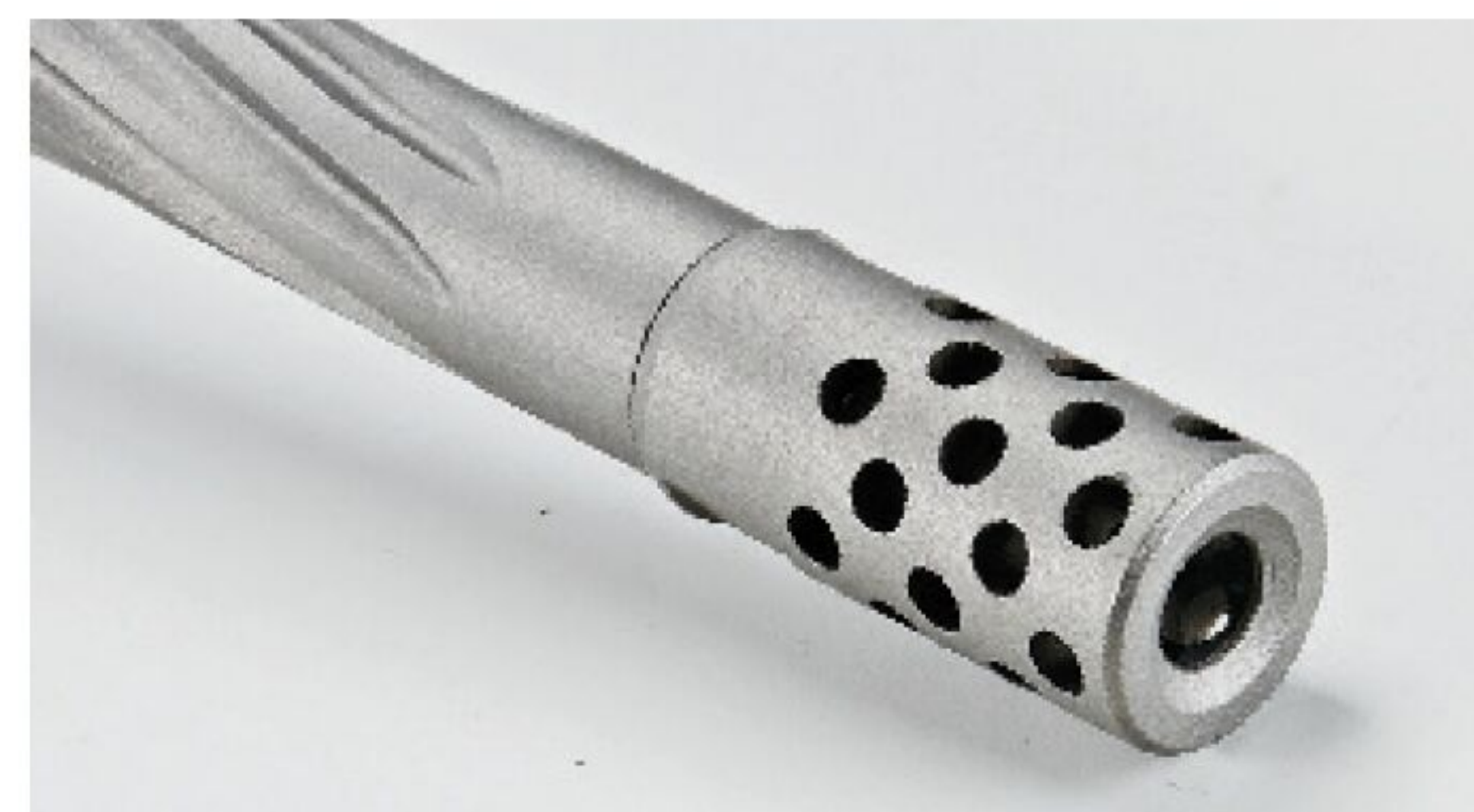
The barrel length of the Gen II Standard rifle is 20 inches. It is cold-hammer forged, spiral-fluted, and threaded. It comes with a removable radial muzzle brake installed.
