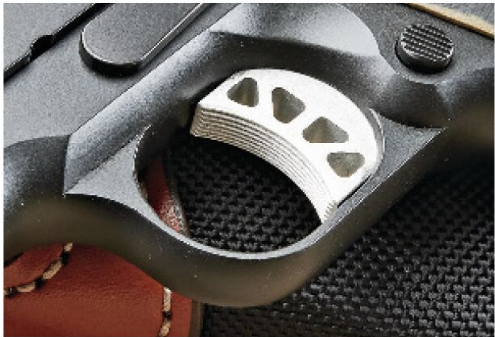
The aluminum match-grade trigger is skeletonized and striated. Our sample’s trigger pull averaged 4 pounds, 11 ounces over a series of 10 measurements with an RCBS trigger pull gauge.
