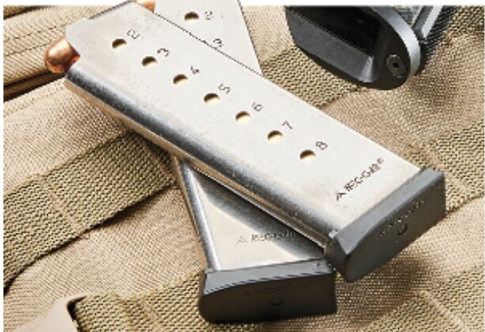
The TRP Classic came with three Mec-Gar magazines that feature flat followers and removable baseplates/bumper pads. Each one holds eight rounds of .45 ACP ammunition.
