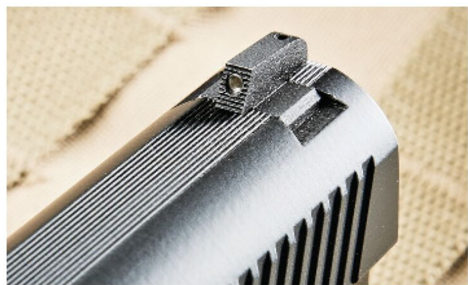
The front sight has a tritium dot and fine horizontal striations to reduce glare. Note the top of the slide features full-length striations, again to reduce glare.
