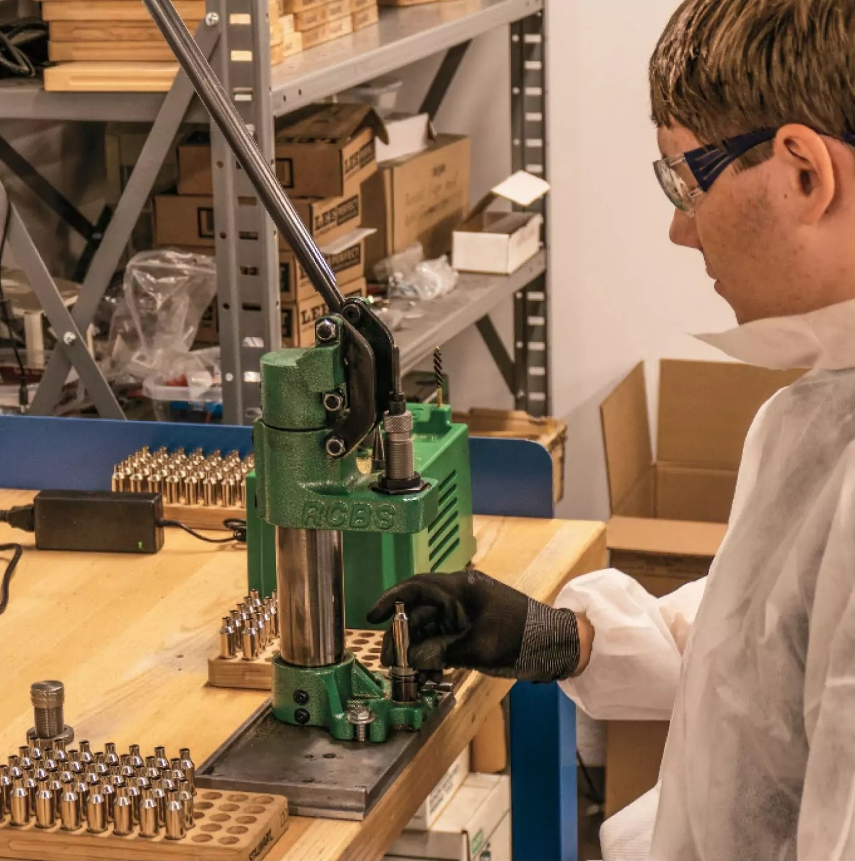
Bulletseating is given an inordinate amount of attention. A cartridge discarded due to excessive bullet run-out at this stage is a costly loss in time and resources.
