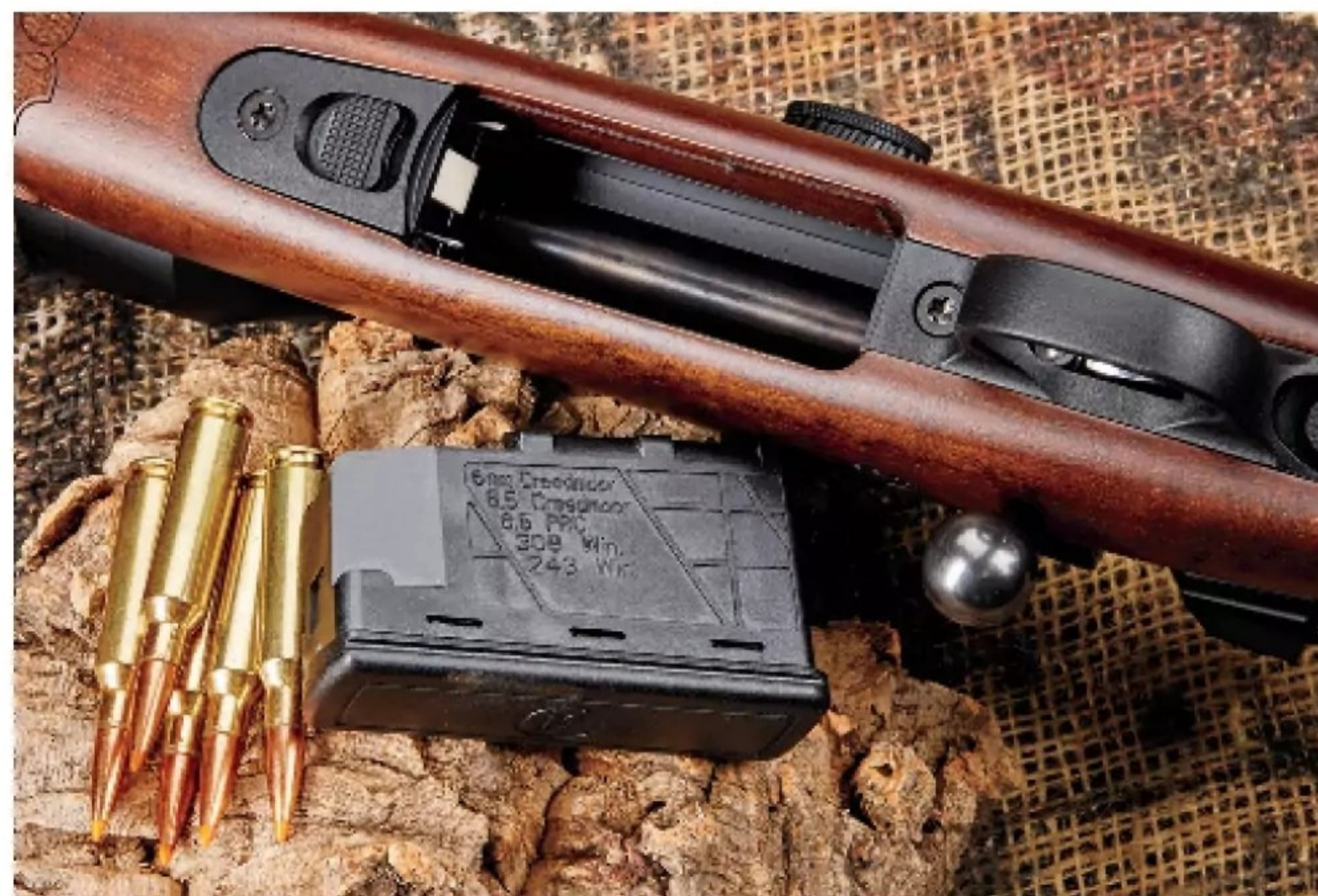
The polymer double-stack magazine holds five rounds. The magazine release is located under the receiver, and it slides forward to lock the magazine in place.
