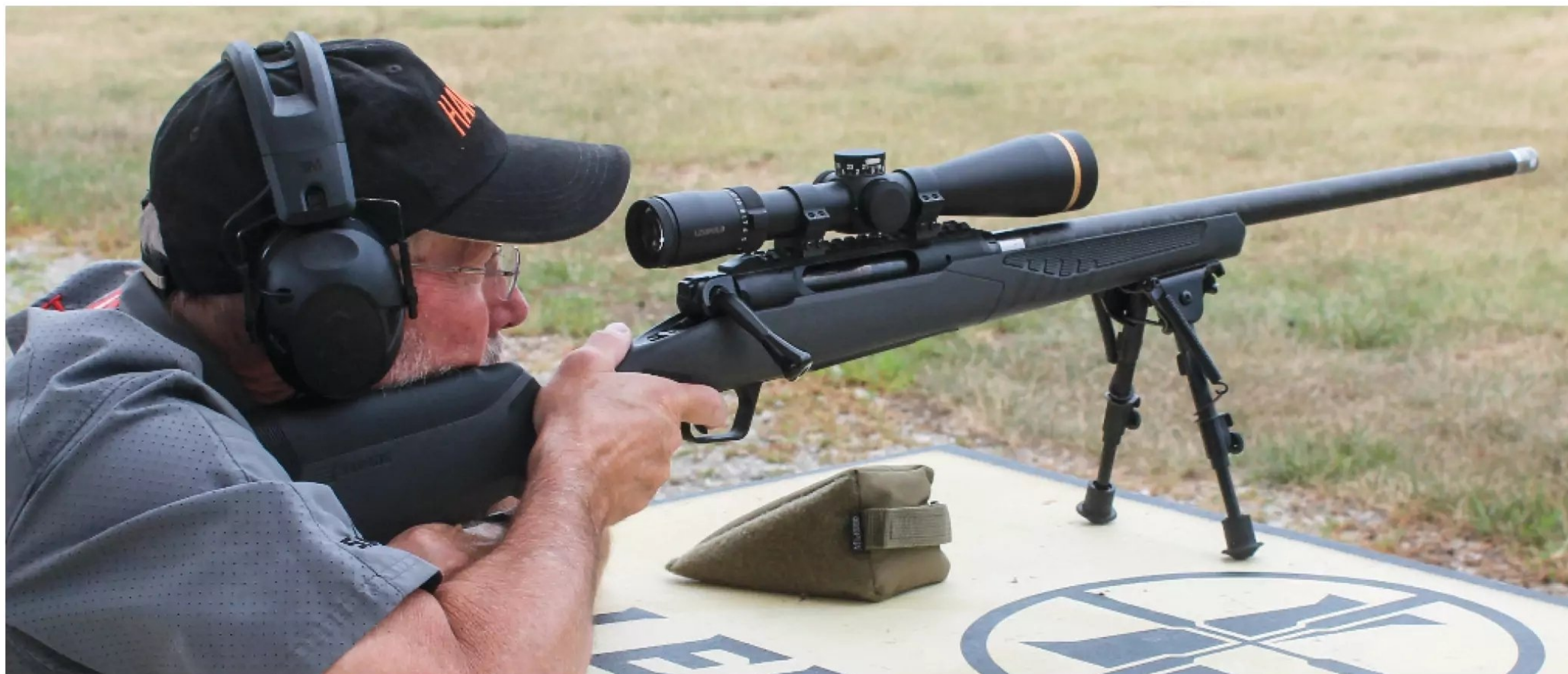
The U.S.-made Savage Impulse is the most economical straight-pull rifle, and uniquely, the bolt handle can be instantly switched from the right side to the left.
