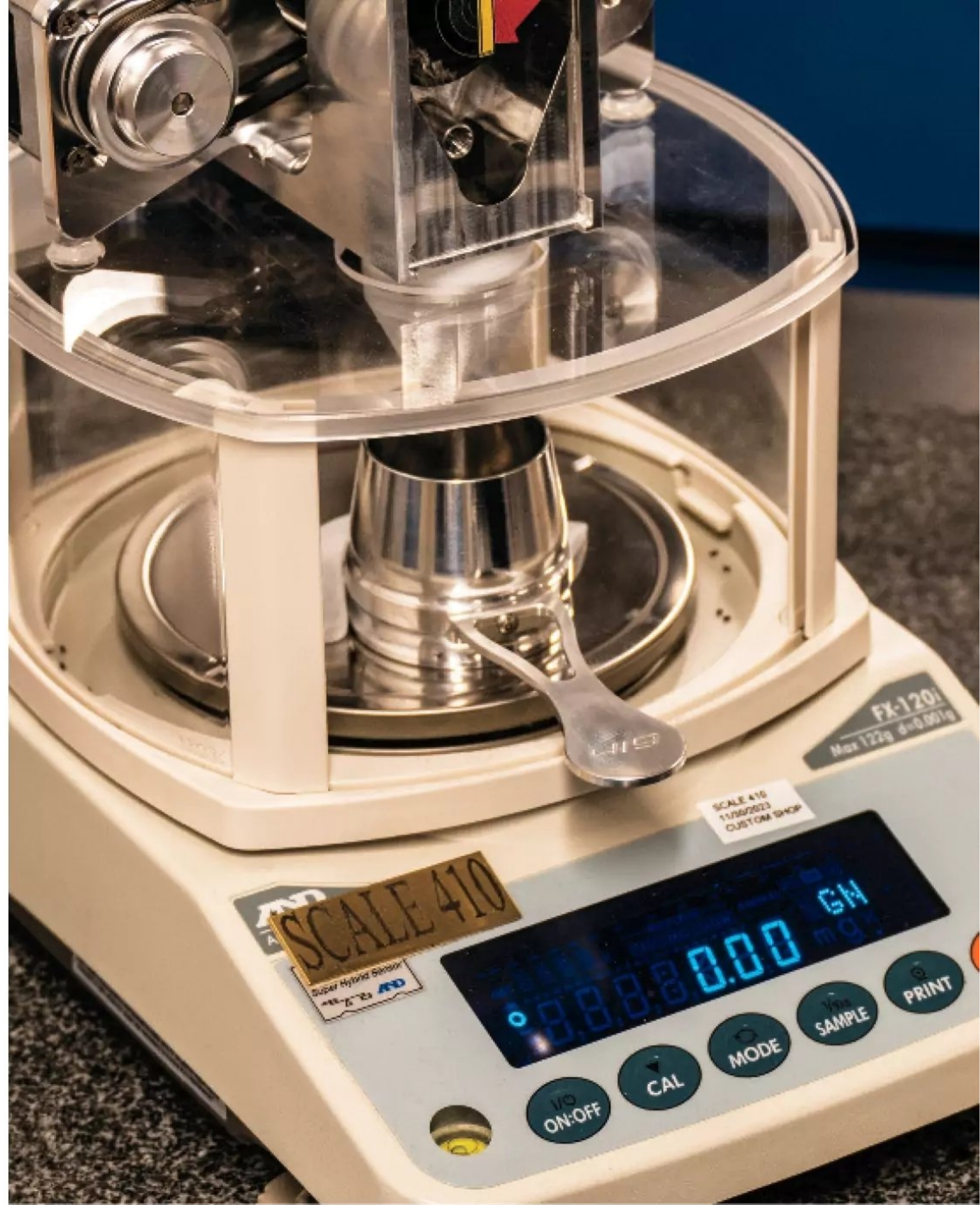
Powder charging is accomplished using weighed charges thrown by some of the most sophisticated lab-grade scales on the market.
