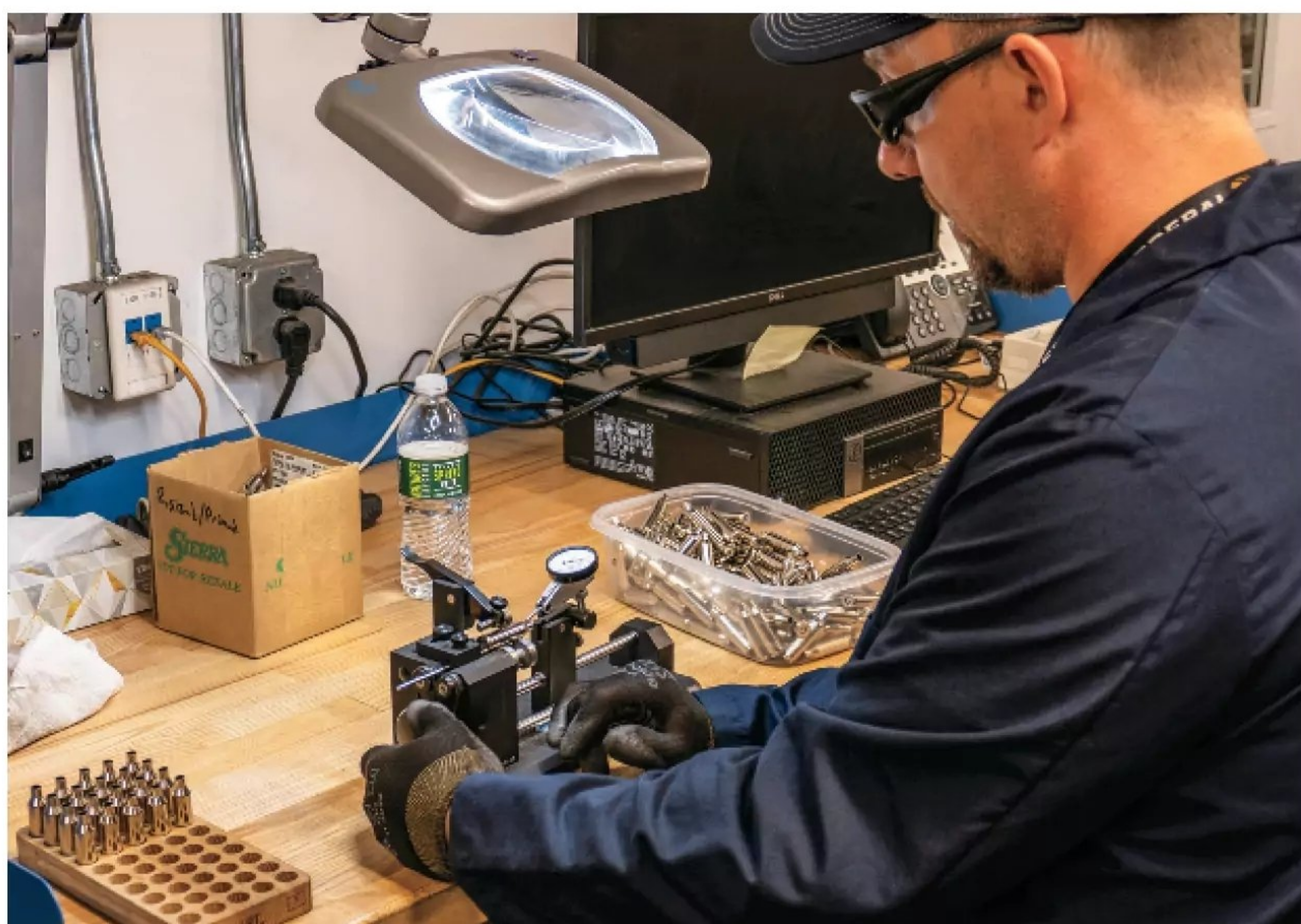
Step one of the loading process is selecting perfect cartridge cases. An amazing number of cartridge cases are discarded during the inspection process.
