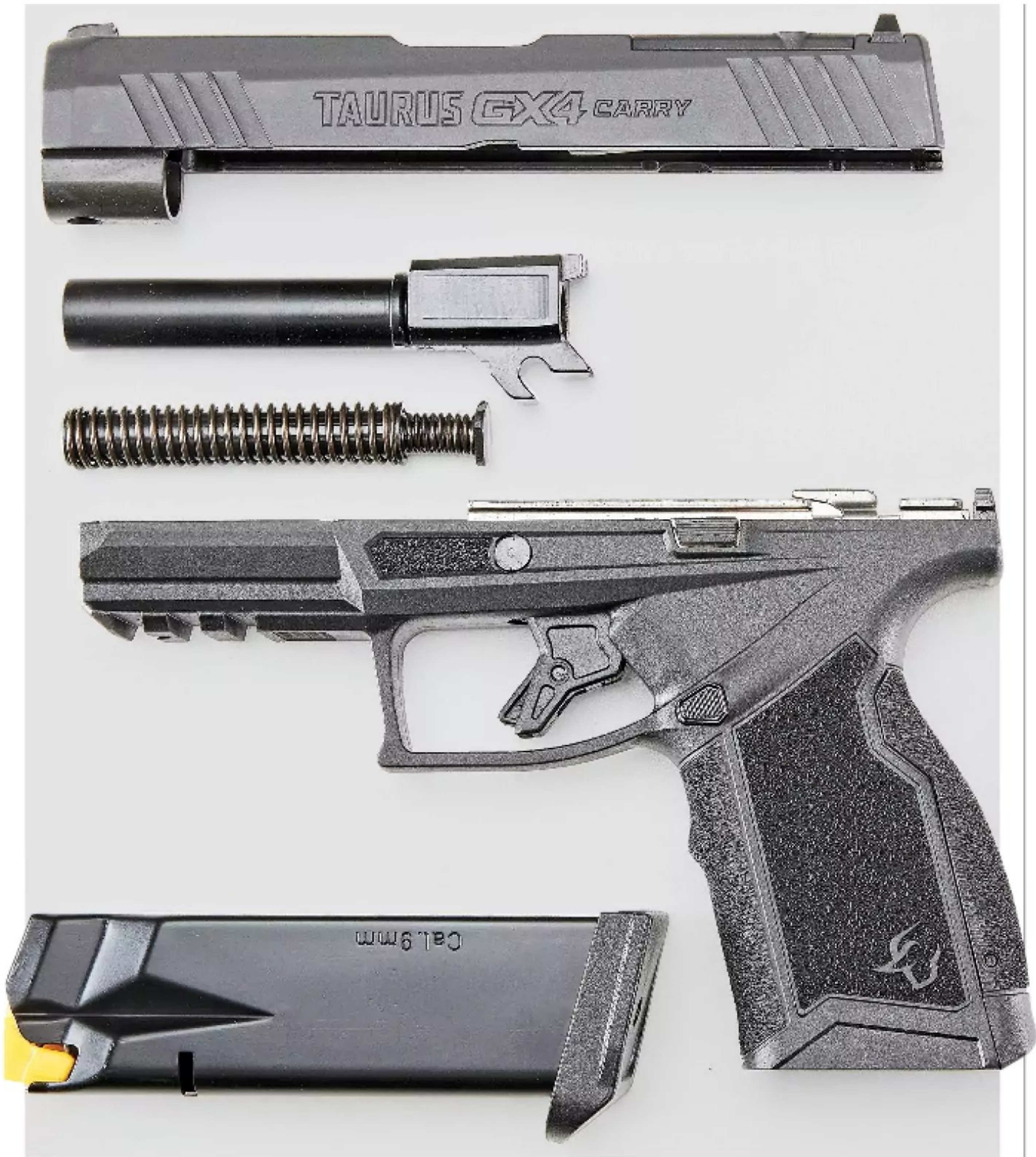
Disassembly requires a flathead screwdriver to rotate the recessed takedown pin (located on the right side of the slide/frame), squeezing the trigger, and removing the slide.
