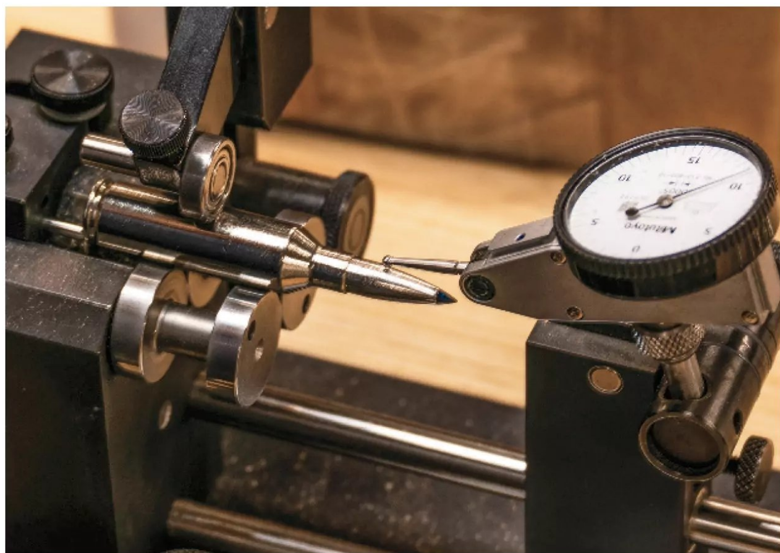
Final inspection includes testing each cartridge on a concentricity gauge. Very little run-out is tolerated.
