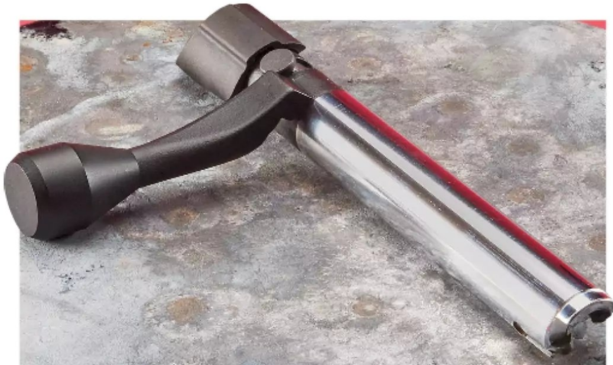
Springfield’s new bolt-action Model 200 Rimfire rifles are built around a blued steel action that utilizes dual cocking cams and provides a 60-degree bolt throw. The 4140 steel bolt has twin extractors, a high-polish white chrome coating, and a threaded bolt handle.
