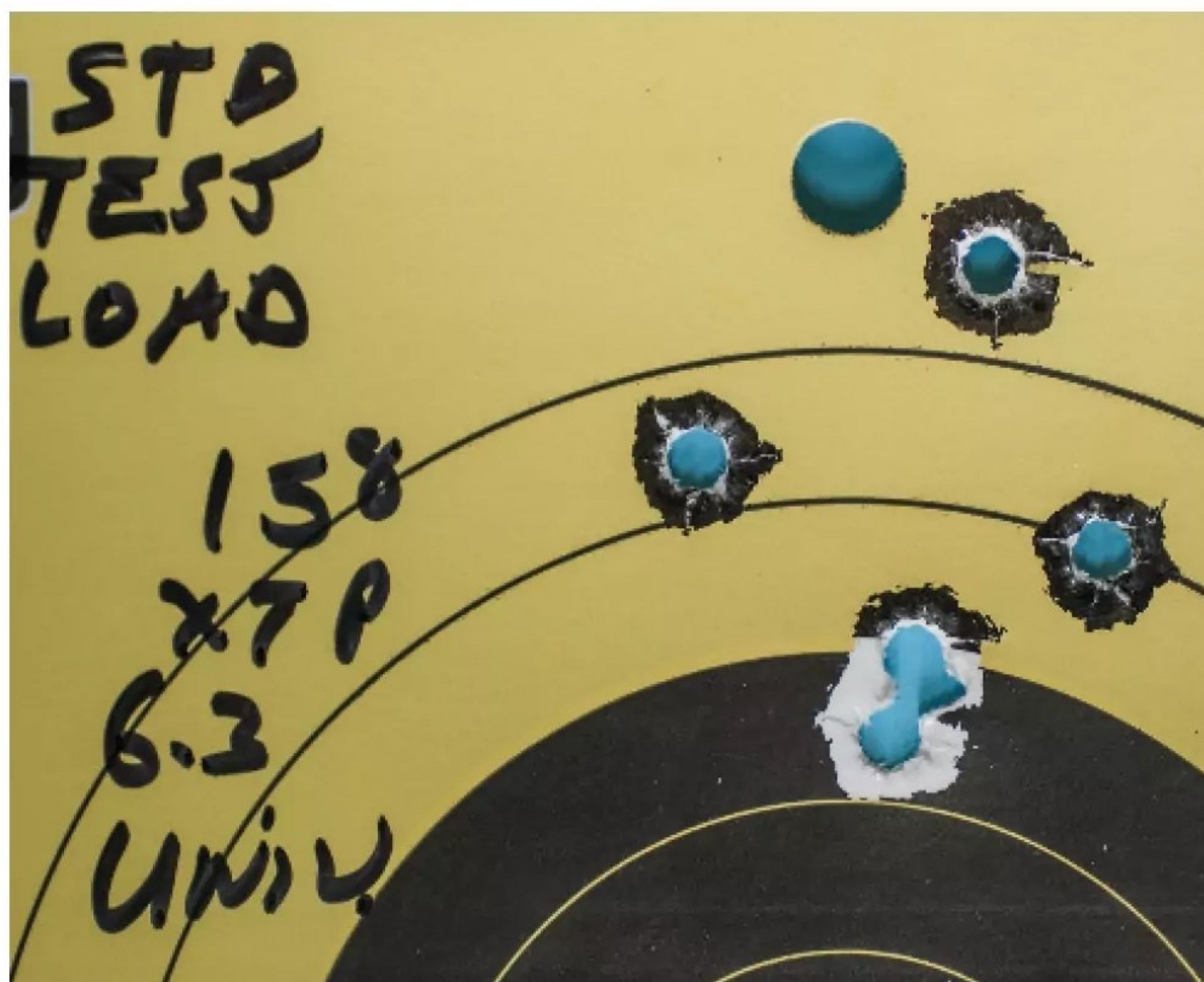
Steve’s go-to .357 Magnum handload consists of the Hornady 158-grain XTP over 6.3 grains of Universal powder, and although it wasn’t the most accurate load in the Defender 605 revolver, it’s still his standard test load.
