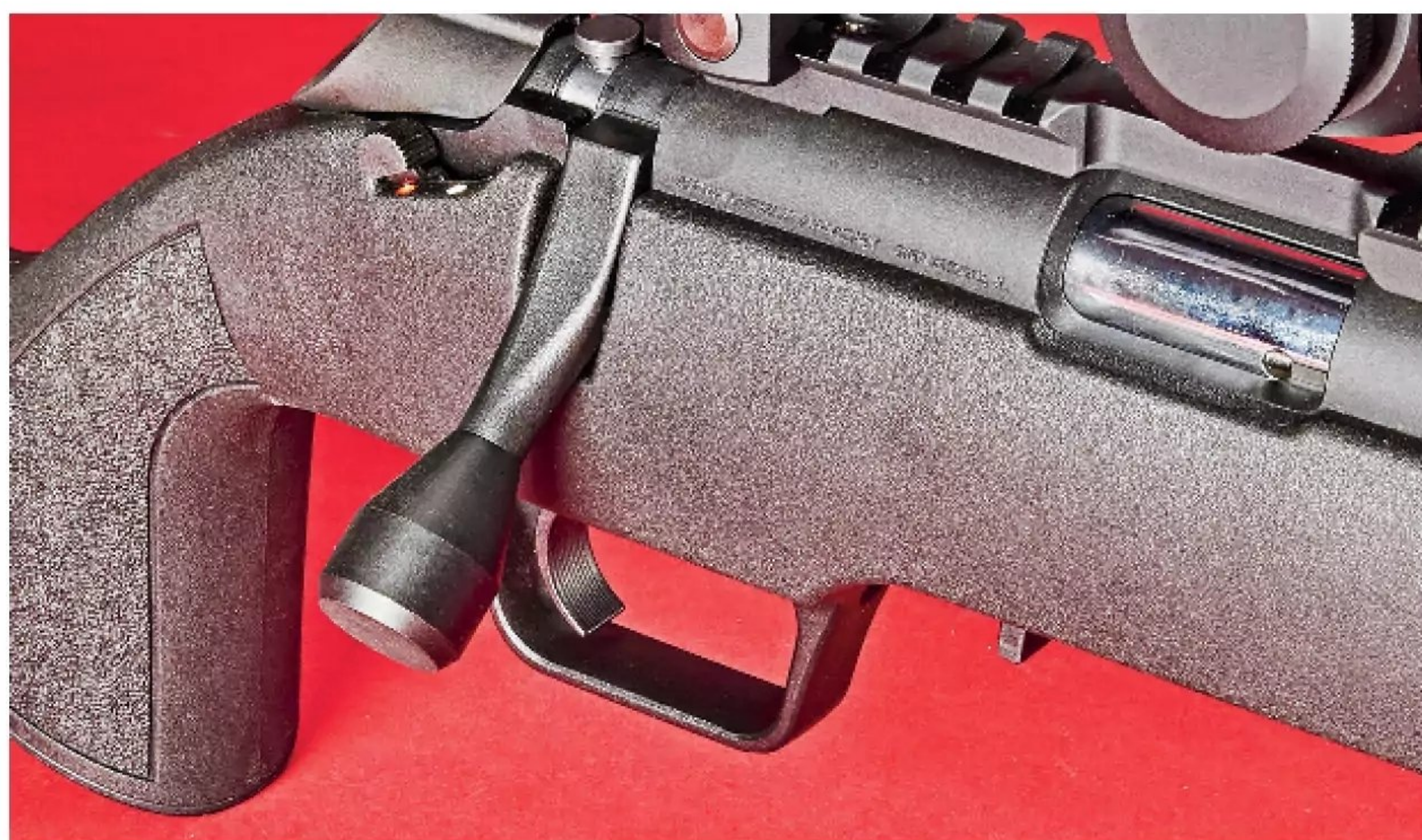
The 700-pattern trigger is user-adjustable for pull from 4.0 to 5.5 pounds. Our Classic rifle was factory-set at 5.5 pounds of pull, and our Target rifle was set at 4.75 pounds of pull.
