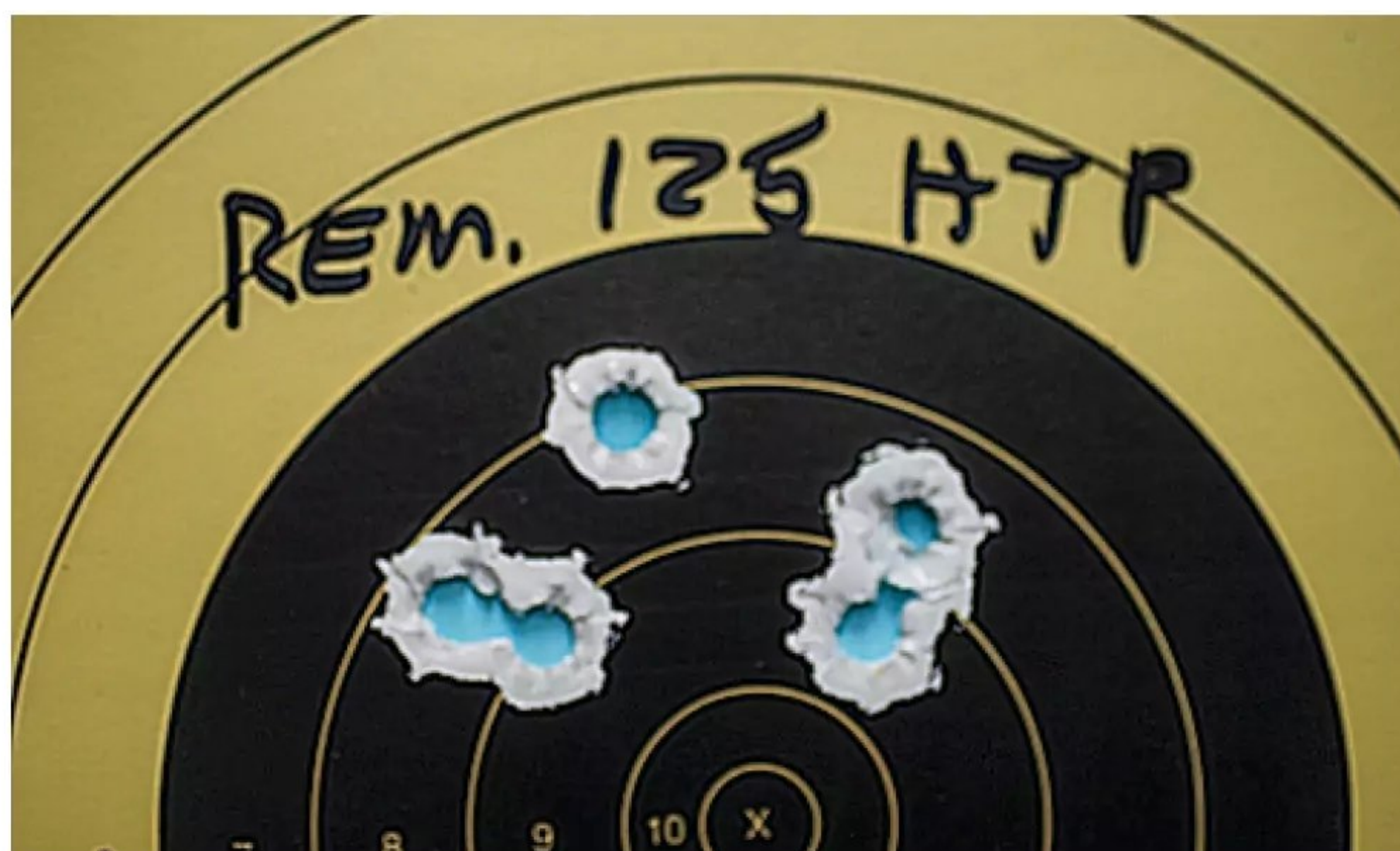
Another fine five-shot group was made by the Remington HTP 125-grain SJHP ammunition. It measured 1.50 Inches. This load also achieved the highest velocity, averaging 1,332 fps.
