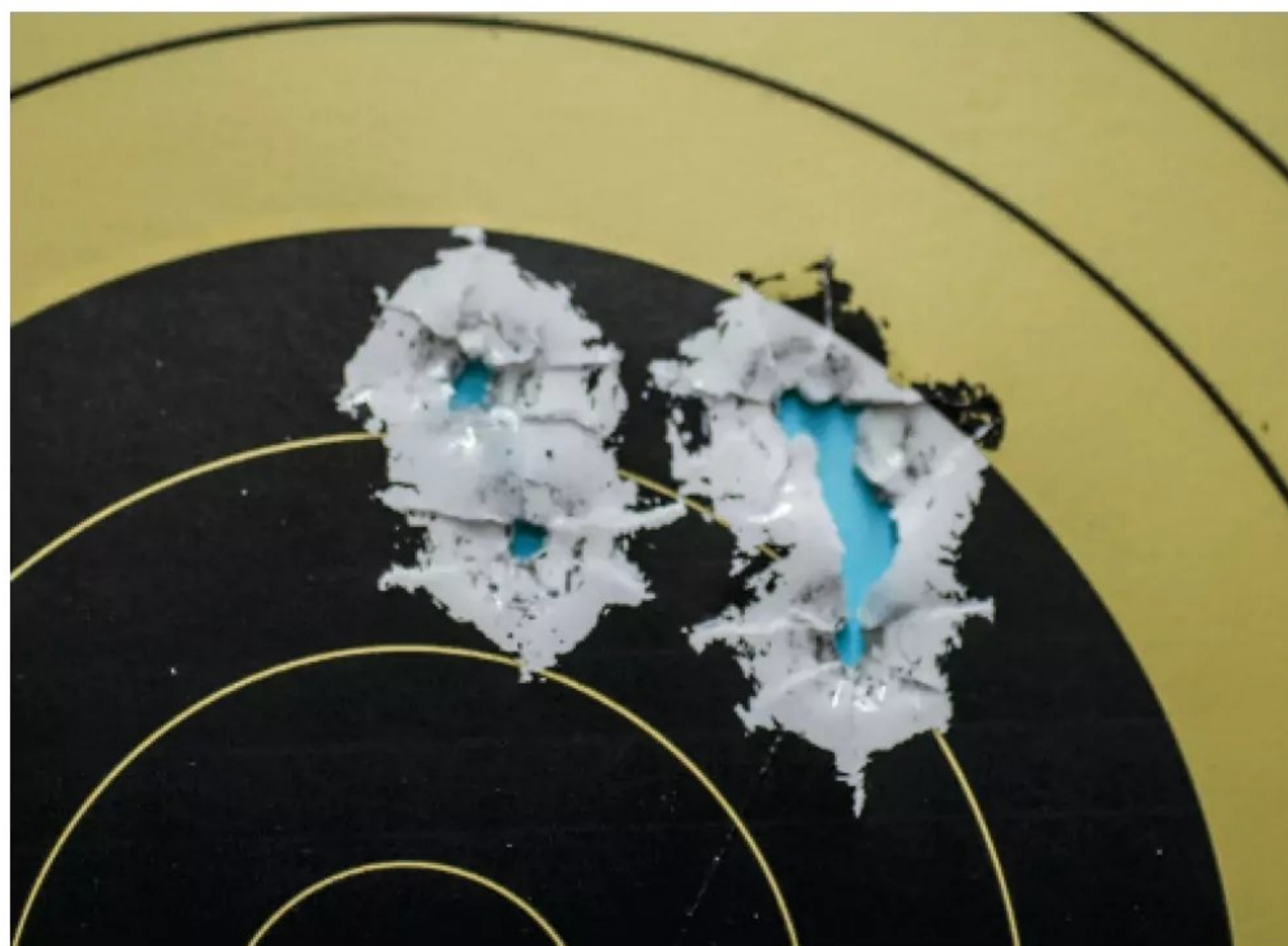
On average, the factory-loaded ammo produced higher velocities and better accuracy than the handloads. This five-shot group was made by the Hornady Custom 158-grain XTP loading, and it measured 1.36 inches.
