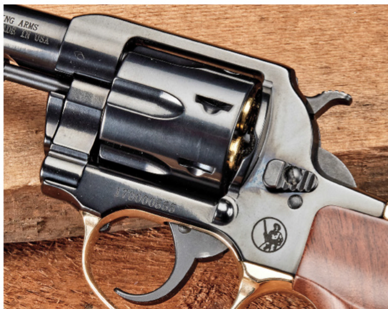
The wheelgun's cylinder, cylinder frame, cylinder release thumbpiece, hammer, trigger, sights, and barrel have a polished blued steel finish.
