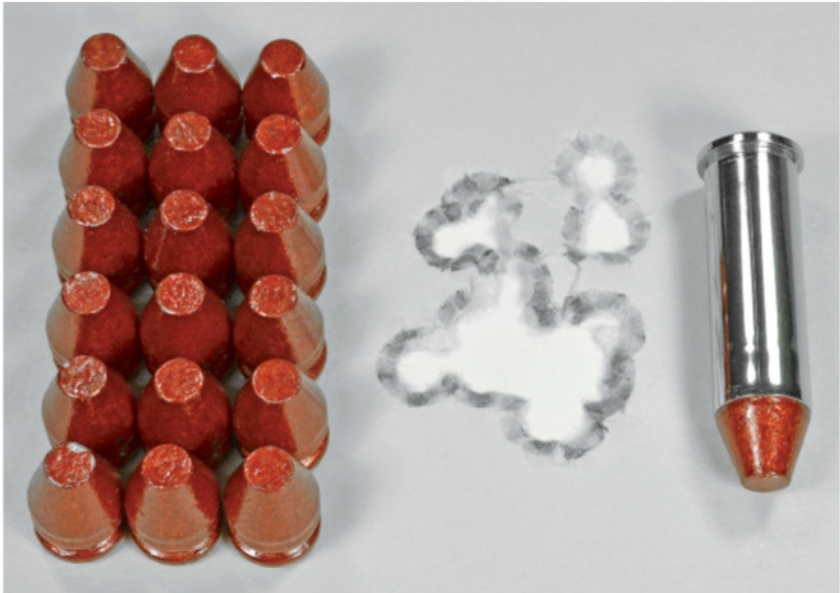
This 18-shot group fired at 25 yards measures 1.2 inches center to center, and it is smaller than the length of a loaded .38 Special round.
