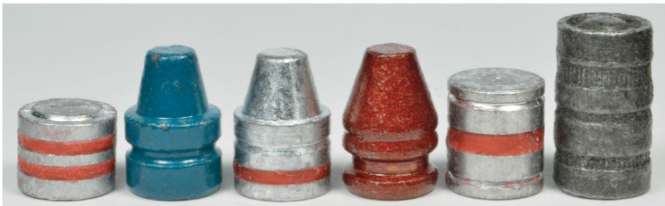
Dr. Miller tested lightweight bullets in .38 Special handloads, including (left to right) Matt's Bullets 75-grain wadcutter, Ibejiheads polymer-coated 100-grain SWC, Matt's Bullets 105-grain SWC, Summers Enterprises polymer-coated 105-grain truncated cone, Matt's Bullets 110-grain wadcutter, and Remington 148-grain hollowbase wadcutter. He fired them for accuracy in an S&W Model 67 with a 4.0-inch barrel mounted in a Ransom Rest.
