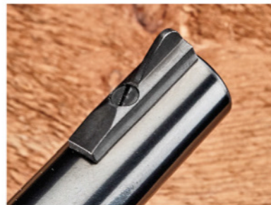
The front sight is a ramped blade held in place by a slot-head screw. The gun comes with three different front sights in low, medium, and high sizes.
