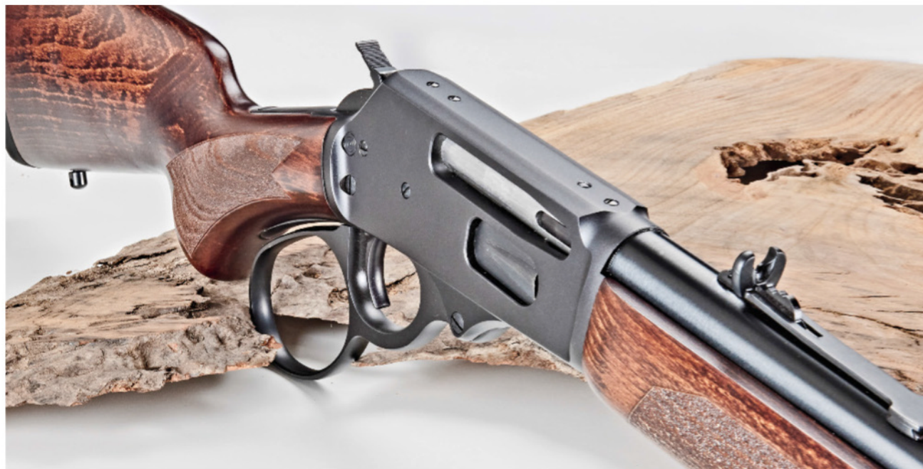
The R95 triggers are smooth and measure 0.27 inch wide. Our Classic version's trigger pull averaged 6.4 pounds. Our Trapper version's trigger pull averaged 5.4 pounds. The hammerspurs are 0.33 inch wide, grooved, and shaped for easy installation of a hammer extension.
