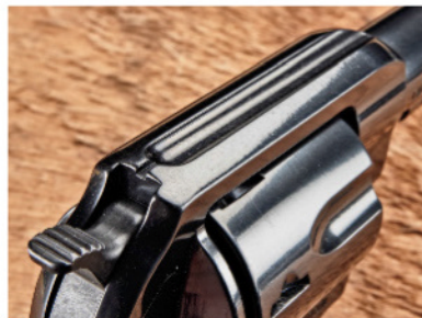
Like many traditional single-action revolvers and vintage double-action revolvers, the Big Boy's rear sight consists of a groove along the topstrap.
