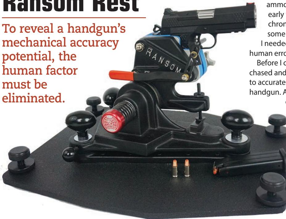
The Ransom Rest eliminates any shooter-induced movement during the firing process, revealing a handgun's mechanical accuracy. Inserts (blue) match the specific model of pistol to ensure a proper fit.
