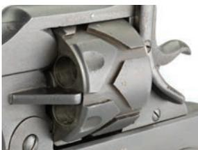
Opening the Webley-Fosbery revolver's top-break action was accomplished via a lever pressed by the shooter's thumb (for right-handed shooters) • Cut into the cylinder, the zig-zag channels helped operate the Webley-Fosbery.
