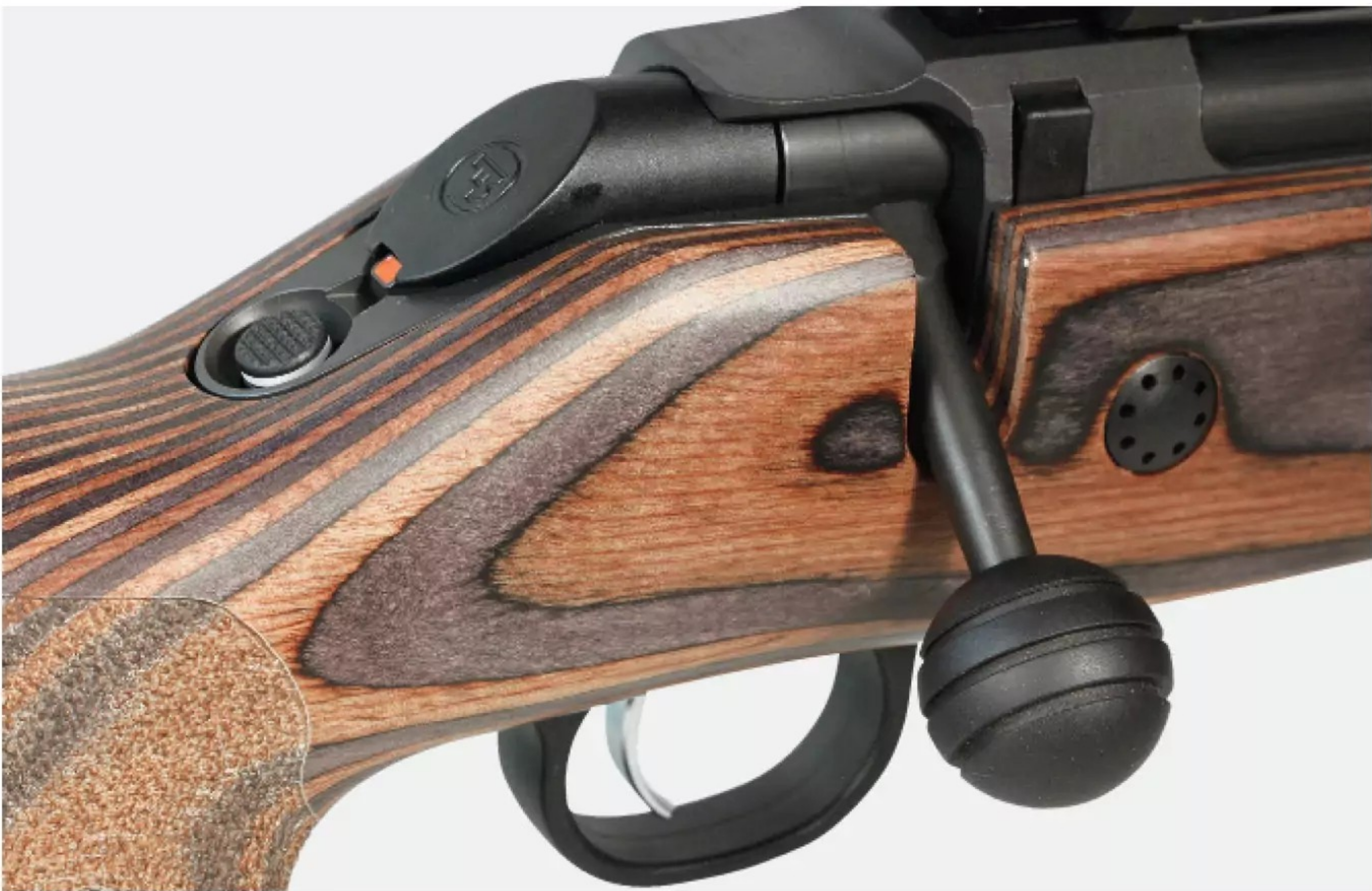
The safety is a vertical crossbolt on the tang, and it locks the bolt on Safe but can be unlocked via the release forward of the bolt handle.
