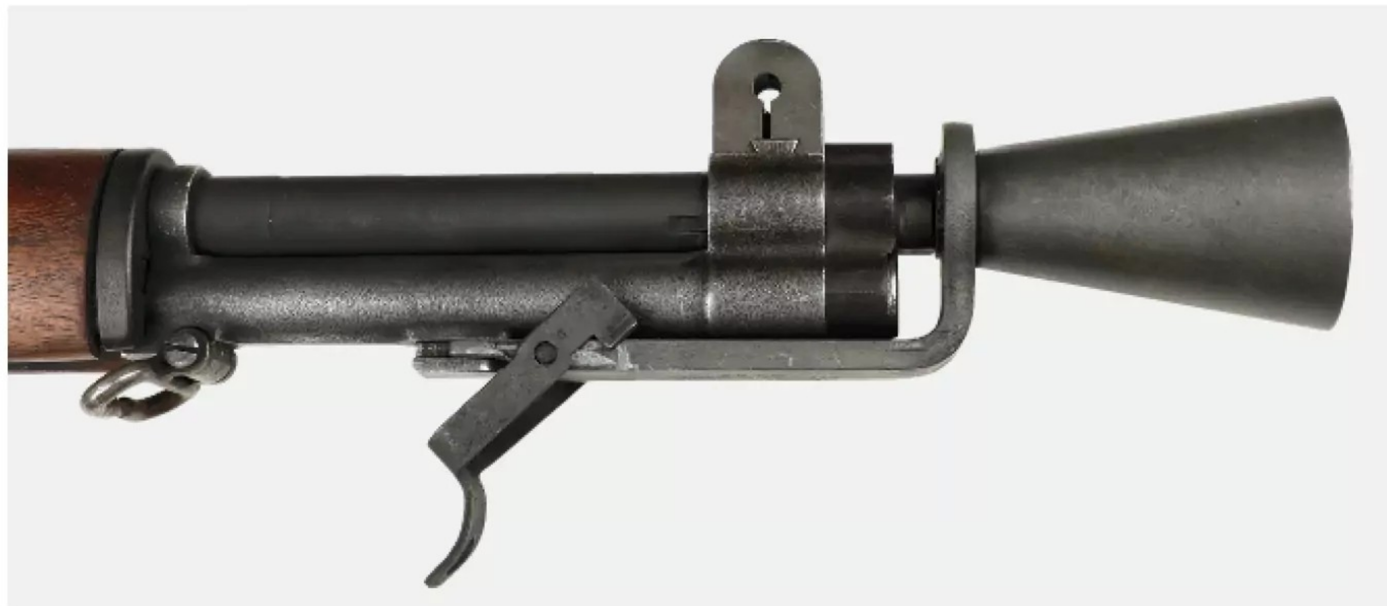
The M2 flash hider weighs nearly a half pound and will change point of impact about an inch at 100 yards. It slips over the muzzle and latches onto the bayonet lug.
