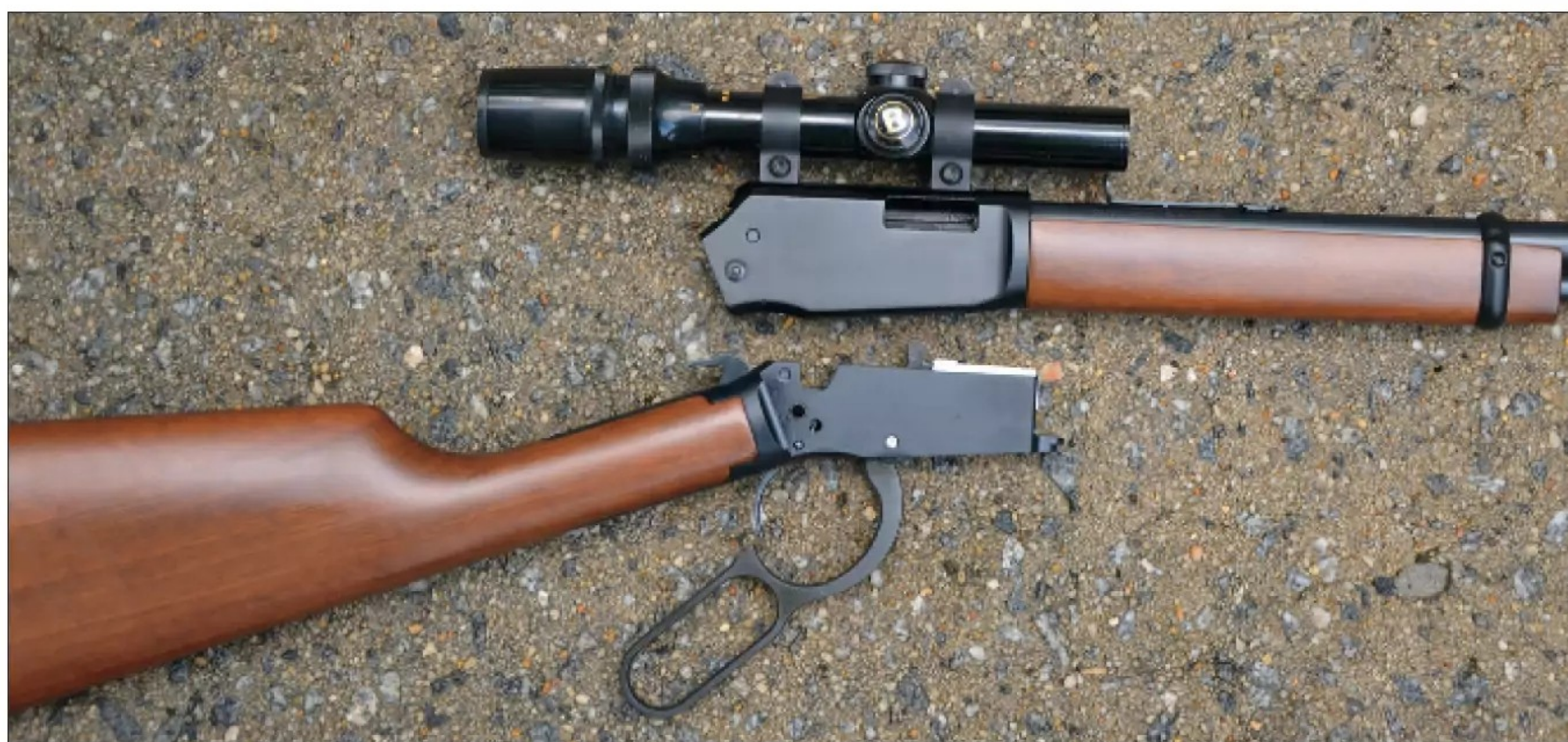
Zero is not lost when the Ranger is taken down and put back together because the scope remains attached to the receiver/barrel assembly.
