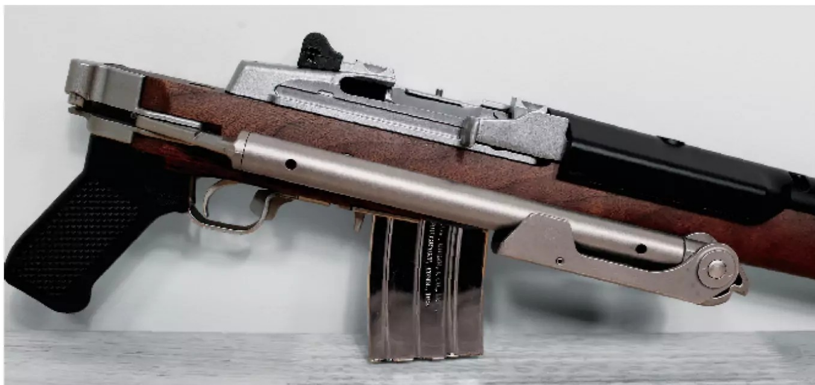
The folding stock not only gives the rifle a cool retro look but also makes for convenient transport and storage. Folding and lockup are solid and secure.
