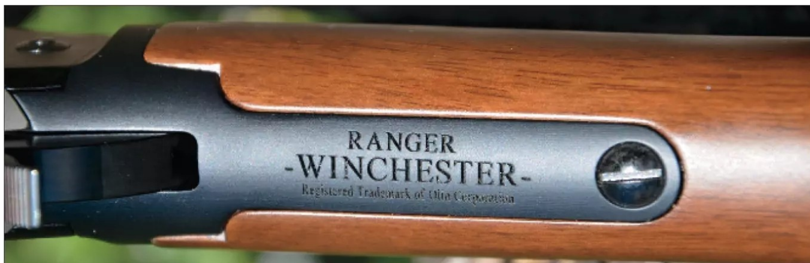
The straight-grip stock is held in place by a large machine screw down through the upper tang of the receiver and into the lower tang.
