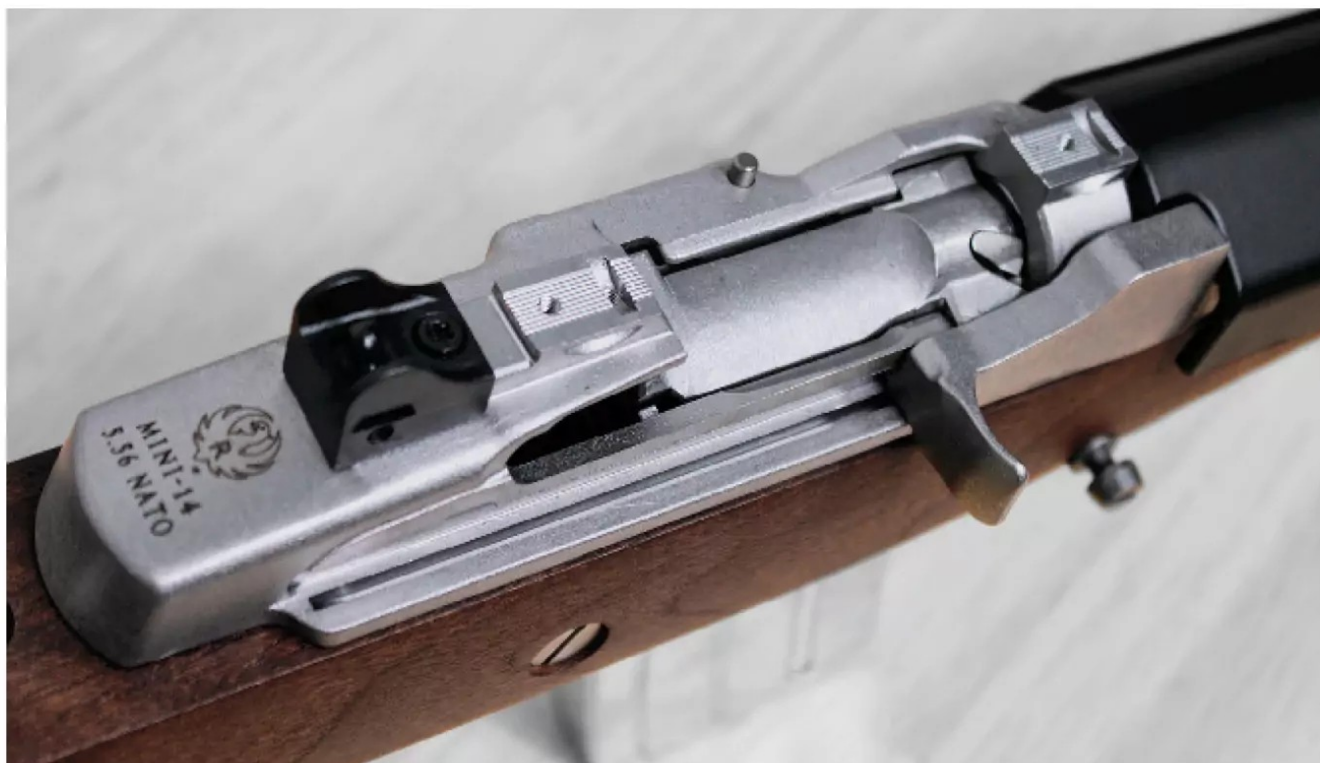
While the Mini-14's gas system is different than the M14's, the bolt is quite Garand-like. The receiver is machined to accept the supplied Ruger rings, and the ghost-ring sight is adjustable.
