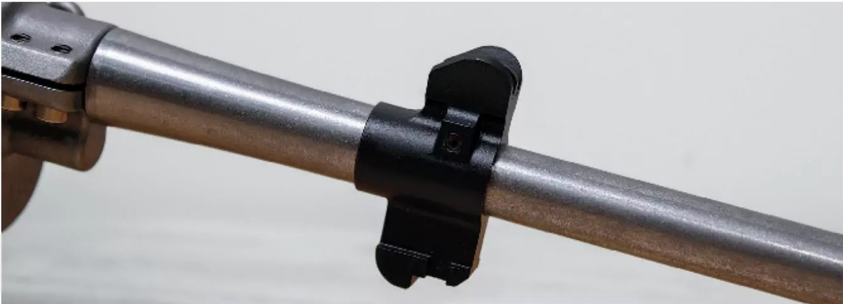
The front sight sits several inches back from the muzzle and includes an integral bayonet lug.
