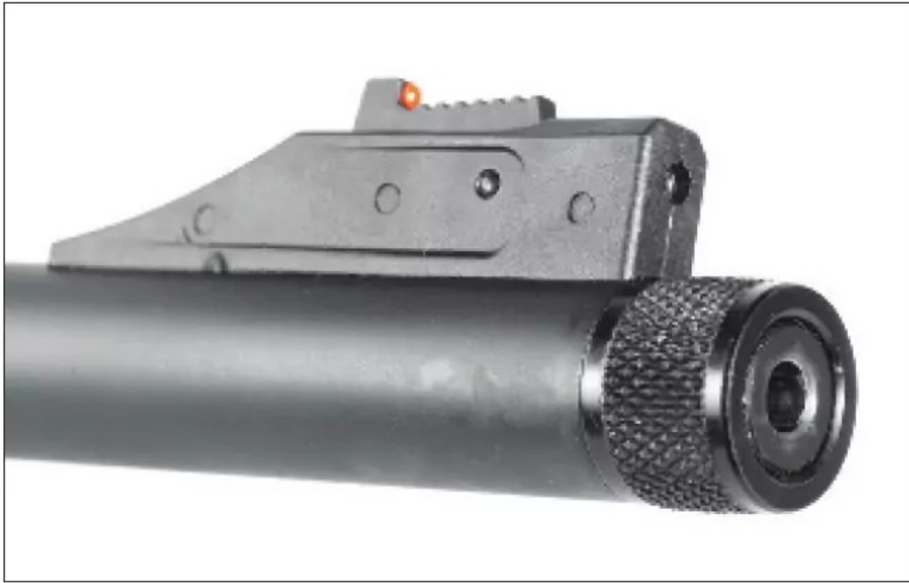
The front sight can be adjusted for elevation via a screw in the front of the sight base. While the barrel is threaded 1/2x28, Rupp's rimfire suppressor did not fit.
