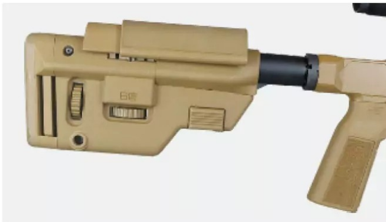
The B5 Systems CPS stock is easy to adjust for length of pull. Gross adjustments are made with a lock lever, finer ones with a thumb wheel. A separate thumb wheel adjusts the cheek riser.
