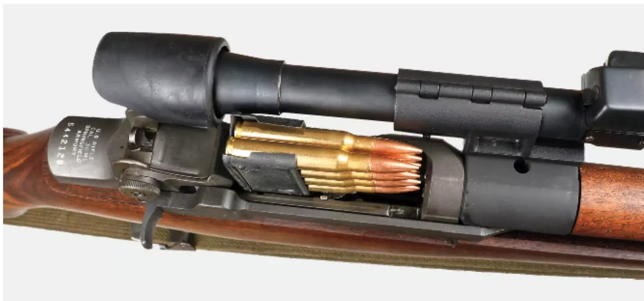
The need to load the M1 from the top meant that the M84 scope had to be placed to the side, which resulted in point-of-impact disparities.
