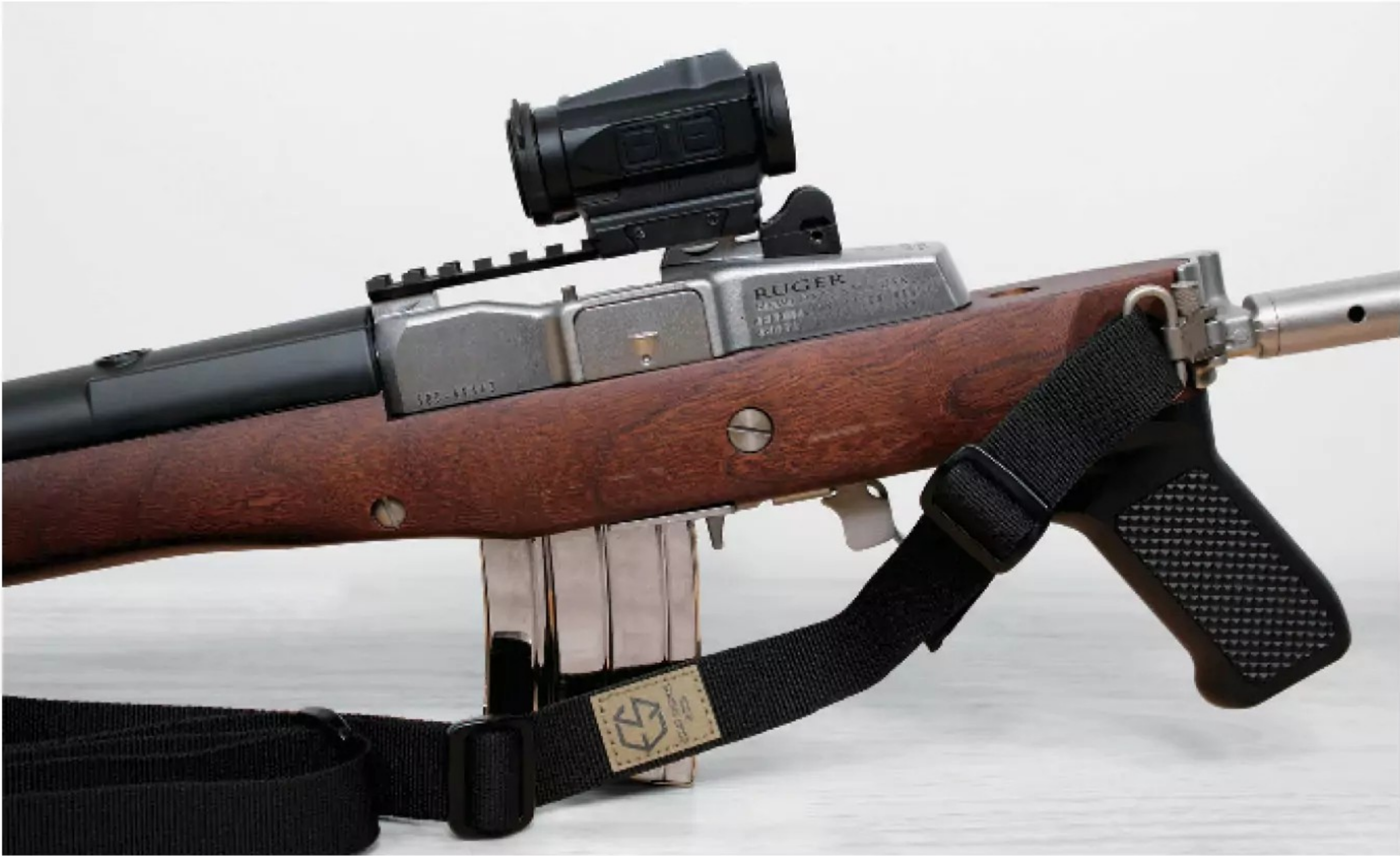
The included Picatinny rail provides for easy optic mounting. The rear sling attachment point is located just behind the receiver.
